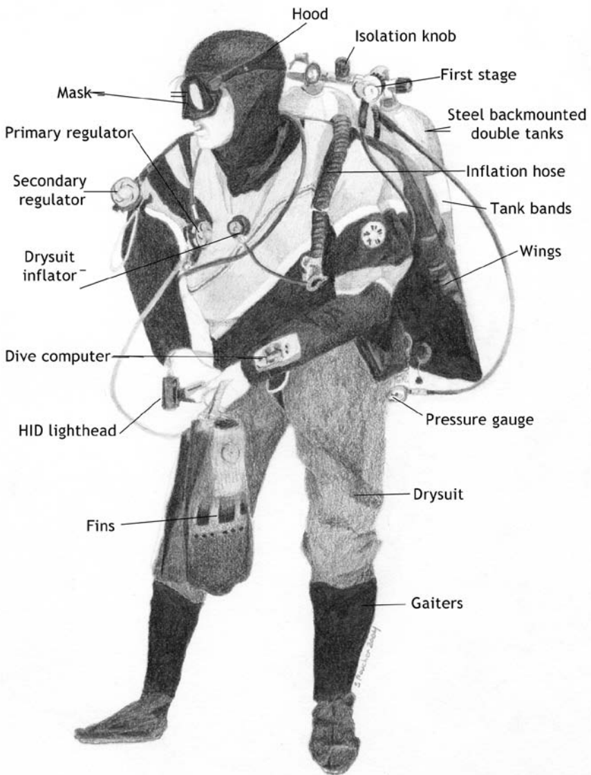
Figure 2. Cave Diving Equipment. Drawing by Sandra Poucher.
