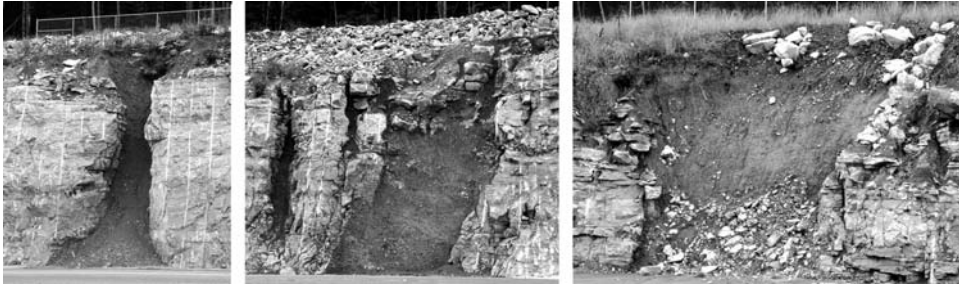
Figure 5.2. Various profiles within some of the buried sinkholes exposed in a single road cut, about 7 m deep, through a limestone hill outside Huntsville, Alabama.
