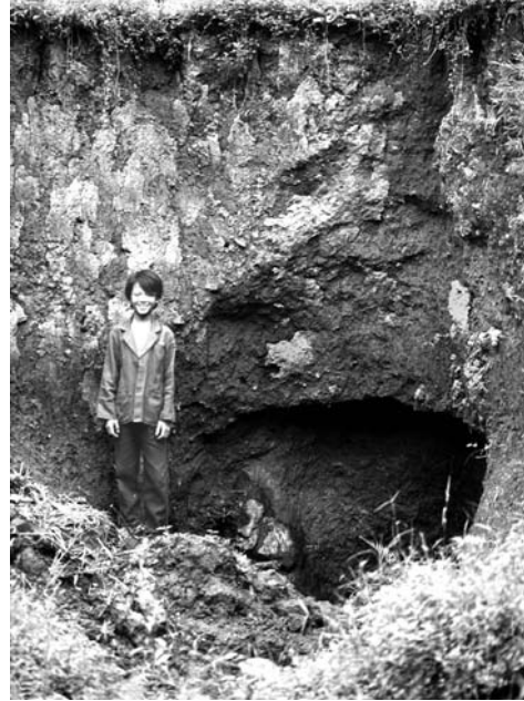
Figure 4.12. A thick soil arched over a piping cavity in the edge of a fresh dropout sinkhole in the Xingwen karst in Sichuan, China; rockhead is deeply pinnacled in this mature karst, and the edge of a limestone pinnacle is exposed just to the right of the boy's feet.
