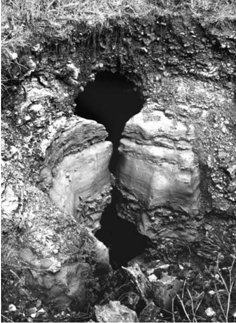
Figure 4.11. A soil arch beneath about 150 mm of cover over a cavity developed over a fissure in limestone rockhead, exposed in the side of a small collapse in Kentucky.
