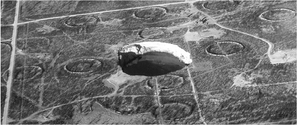
Figure 13.11.4. Aerial view of Wink Sink #2 in March 2003; the sinkhole is about 185 m across, with its 240 m length foreshortened, and each circular earth berm is about 100 m in diameter.
