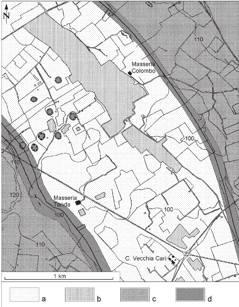
Fig. 13. Vulnerability zonation at the second level of analysis, with indication of the point centres (fault zones, collapse and solution dolines, quarries, etc.). Explanation of vulnerability levels: a, low; b, moderate; c, high; and d, very high.
