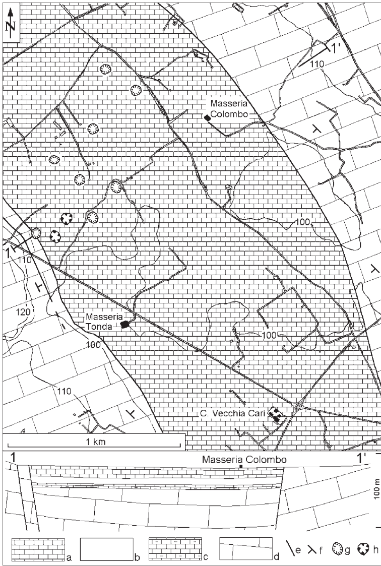
Fig. 2. Geological and morphological sketch of the study area (simplified after Martinis 1970). Key: a, top calcarenites; b, argillaceous silts with sandy intercalations; c, bottom calcarenites; d, limestone bedrock; e, fault; f, strata attitude; g, solution doline; and h, collapse dolines.
