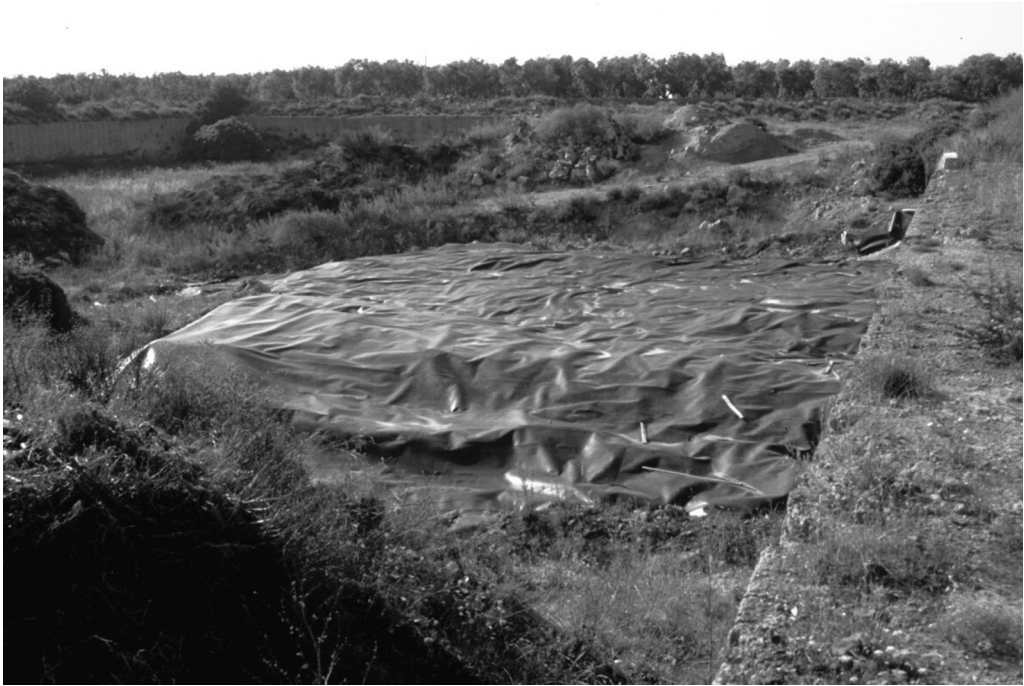
Fig. 10. The drums of waste industrial oils that were stored in one of the quarries (site B in Fig. 6) in the year 2000, and which are still there below the plastic cover (photograph taken in June 2003).
