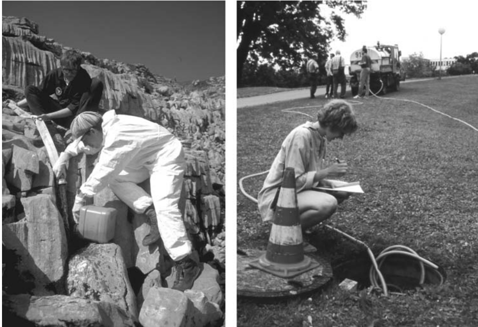
Figure 8.1. Left: Injection of 1 kg of uranine from a plastic container into a karst shaft in the Hochifen-Gottesacker area, Austro-German Alps. A helicopter delivered a tank with 800 L of flushing water (Goldscheider 2005). Right: Injection of 155 kg of naphthionate, dissolved in a tank of 2000 L, into an observation well in the confined karst aquifer of the mineral springs of Stuttgart, Germany (Goldscheider et al. 2003).
