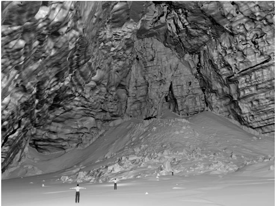
Figure 3.4. 3-D view of an underground chamber. This 3-D model has been obtained by combining 3-D and 2-D lasers canner techniques (by ATM3D/SISKA 2006).
