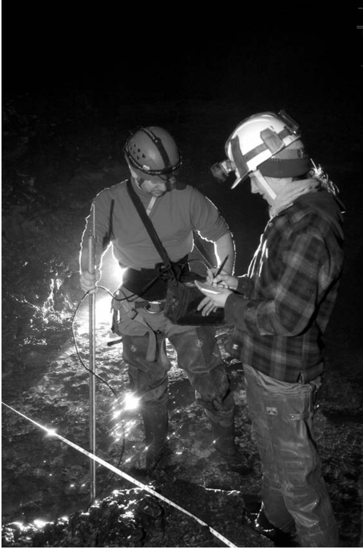
Figure 4.3. Discharge measurements using wading methods can be made underground, although this is somewhat limited by the portability of the equipment. This measurement is being made more than a half kilometre from the Doyel Valley Entrance to the Mammoth Cave System, but in this case relatively large passages make transport of the equipment feasible, if not particularly convenient (photo Groves).
