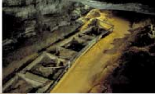
Fig. 19. Vats used in the 1800s to leach saltpeter for gunpowder. Mammoth Cave, Mammoth Cave National Park, KY.
