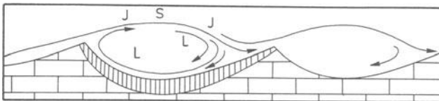
Fig. 12.8. Movement of water over scallops according to Blumberg (1970). S shearing surface; L lee-whirl; J jet stream; hatched corrosion or erosion
