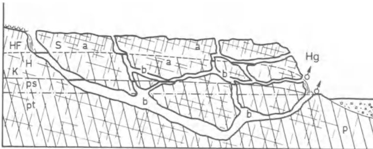
Fig. 9.19. The origin of the water of a karst spring. a narrow open joints, fissures; b karst-hydrologically active cavities; S, H vadose zone with percolation zone S (seepage zone) and high-water zone H ; ps, pt shallow, deep phreatic zone; K karst water surface; HF high-water surface; Hq high-water spring
