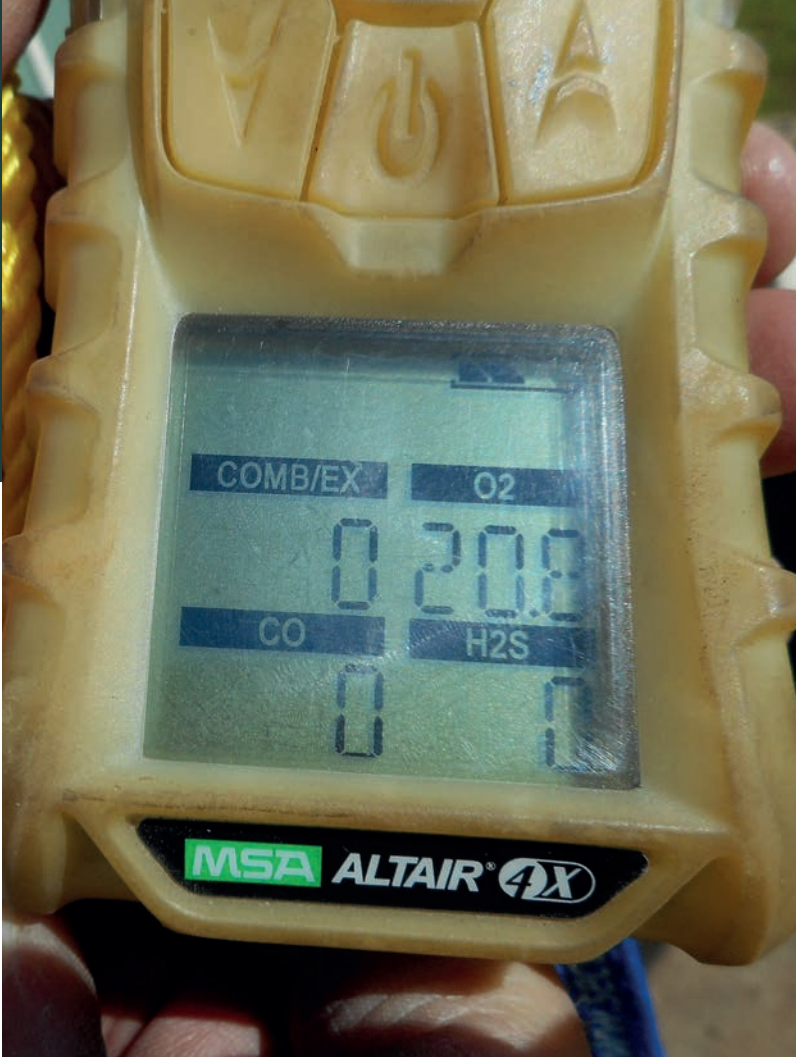
Continuous gas detector showing Safe O 2 levels with no atmospheric contaminants detected.
