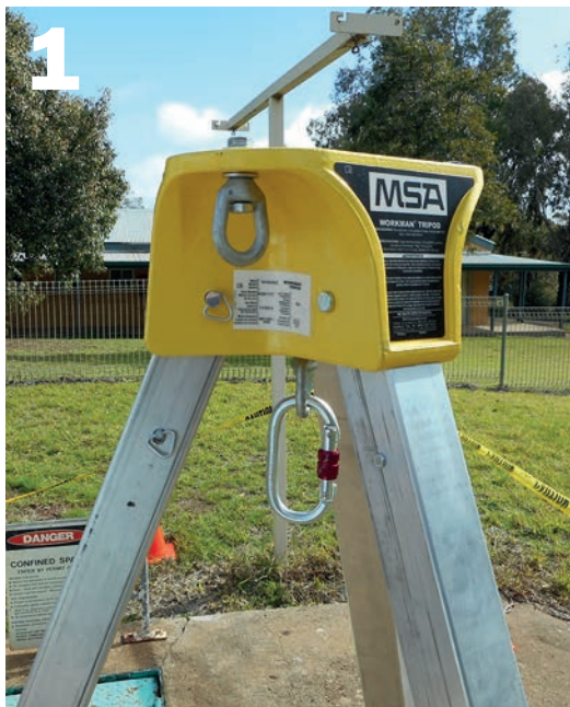
1 Remove the tripod from the carry bag and attach the connecting device to the tripod (in this case a carabiner).
