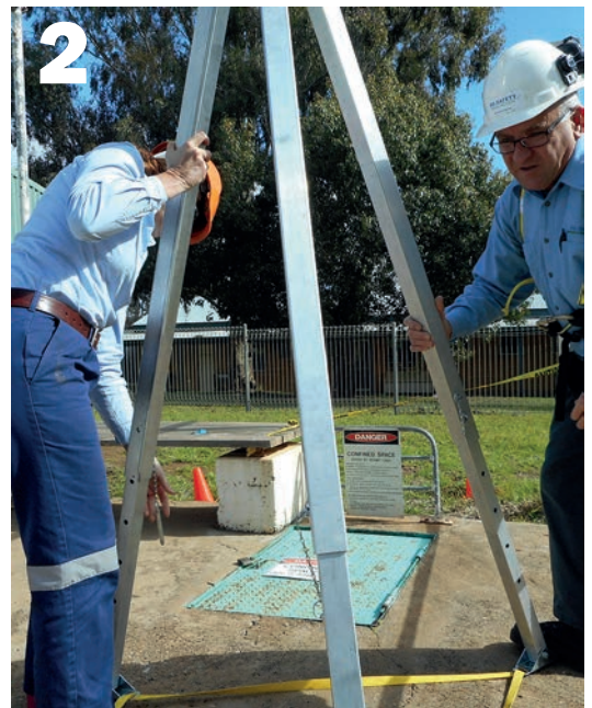
2 Expand legs so that the set up height allows the connecting device to be at a suitable height above the load and then insert holding pins in legs and tighten base straps.
