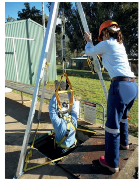
Rescue simulation of unconscious worker using spreader bar attached to retractable lifeline and tripod.
