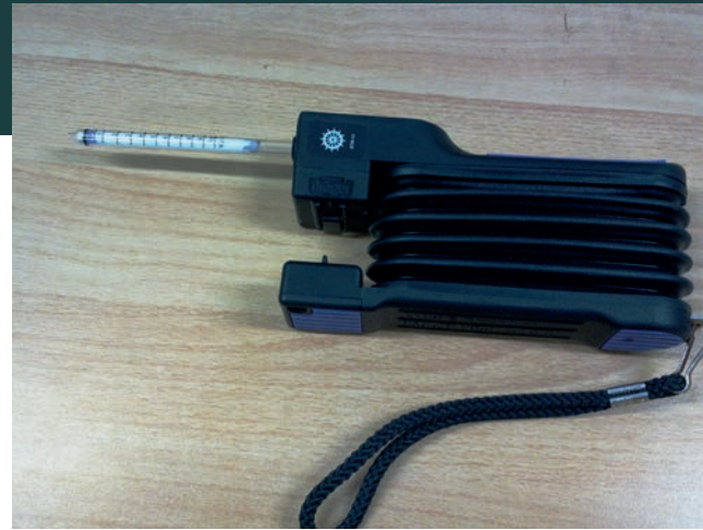
Example of colourimetric tube in manufacturer's bellows (or pump).
