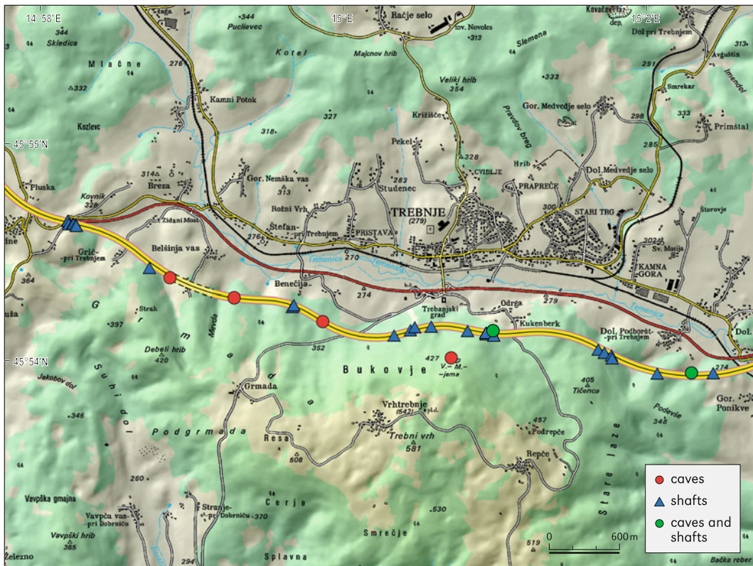
Fig. 16.6 Caves uncovered on the Pluska–Ponikve motorway route
