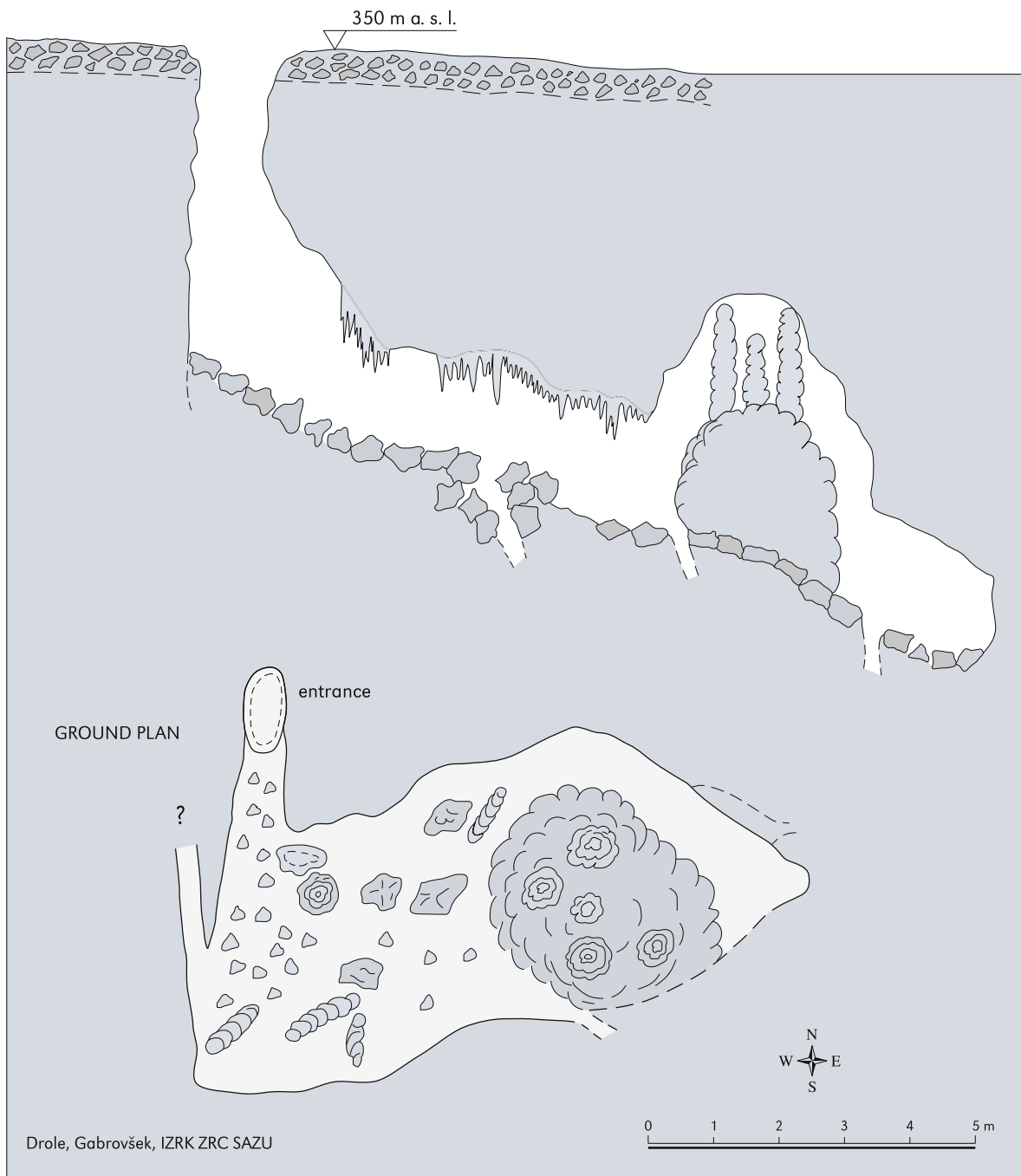
Fig. 5.2 A cave whose roof collapsed during gravel reinforcement works on the route
