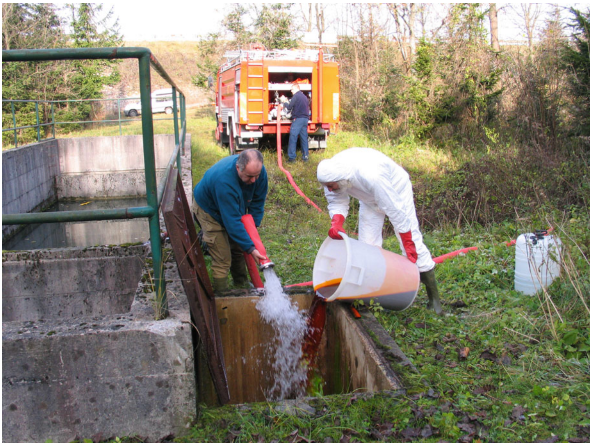
Fig. 28.8 Injection of uranine into the sinking stream of the oil separator B at Postojna
