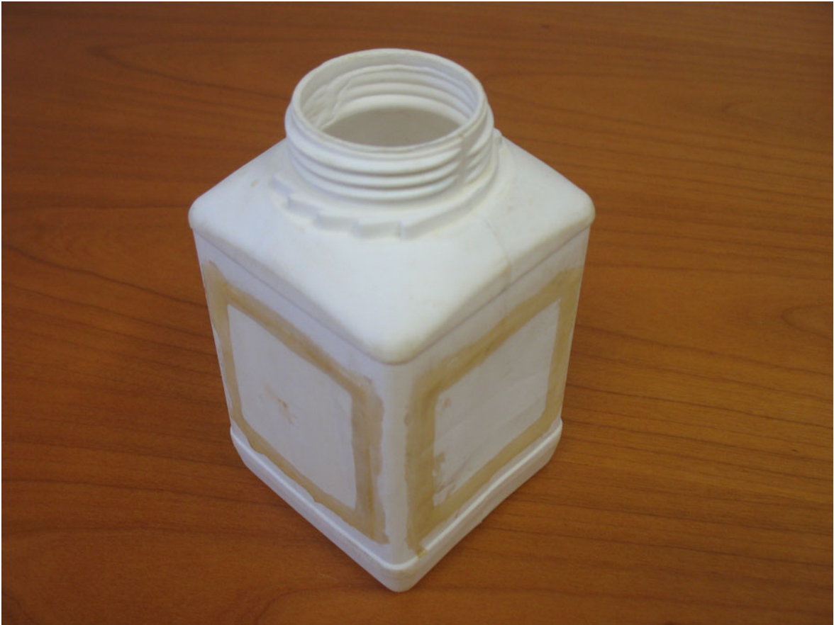
Fig. 26.4 Filtering bottle with mesh screens on the sides that allow water to pass through and retain all organisms entering via the drips
