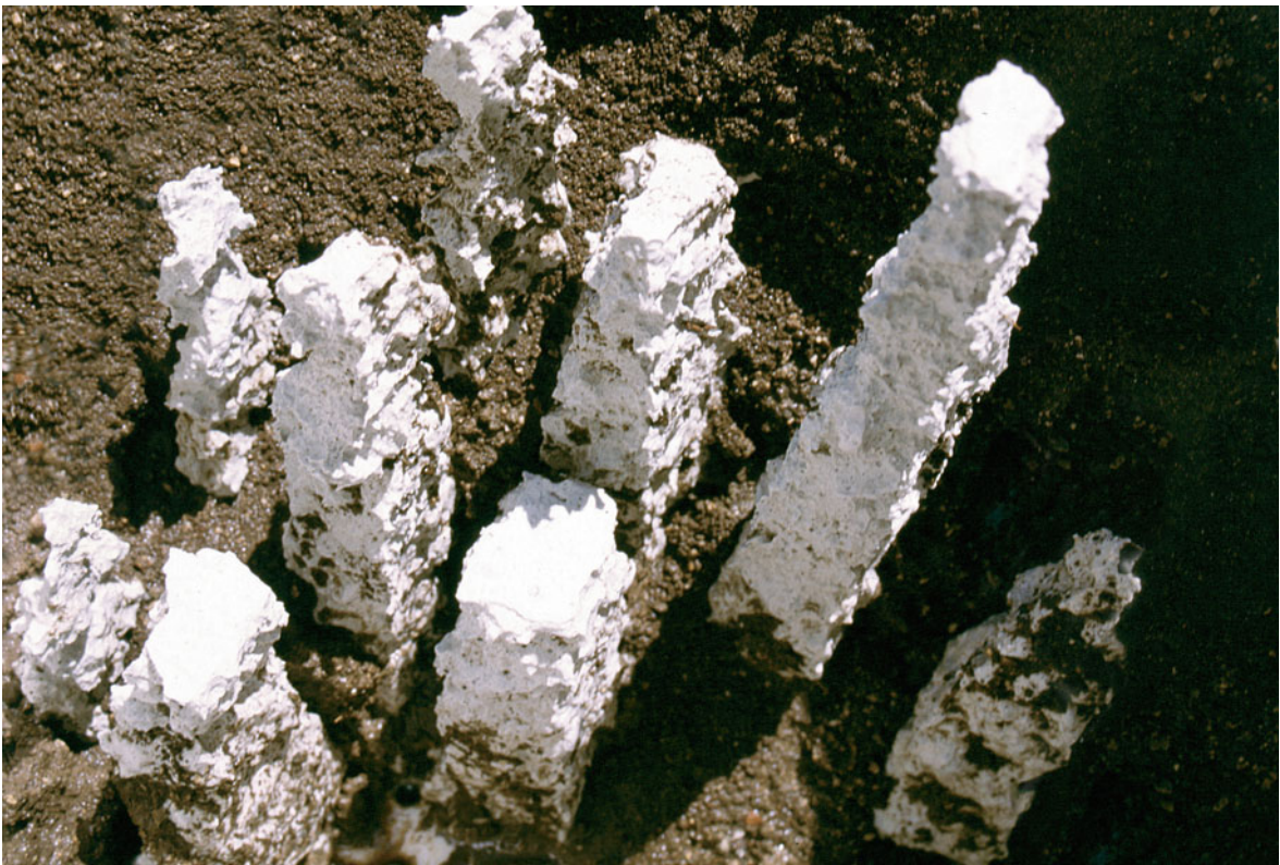
Fig. 21.5 Uncovered subsoil forest in the course of laboratory testing with gypsum
