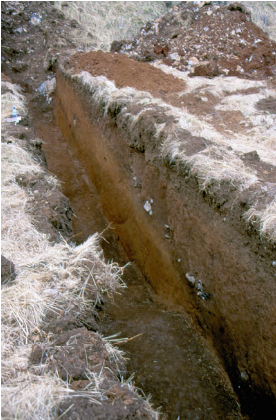
Fig. 10.4 Profile in the doline V2. Visible in the bottom are the layers of red and yellow loam from which two samples were taken for mineralogical analyses
