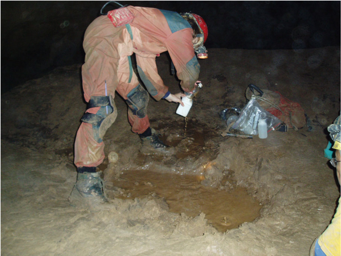
Fig. 26.3 Collecting of water from a pool and filtering through a filtering bottle
