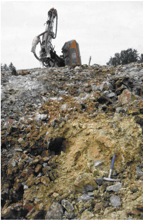
Fig. 10.7 A cave filled with a yellow clastic sediment in the motorway route Divača–Kozina, from which a JSED sample was taken for analysis
