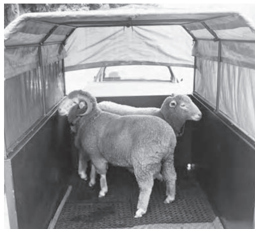
A well-designed trailer for moving sheep – non-slip floor, well ventilated and weather protection.
