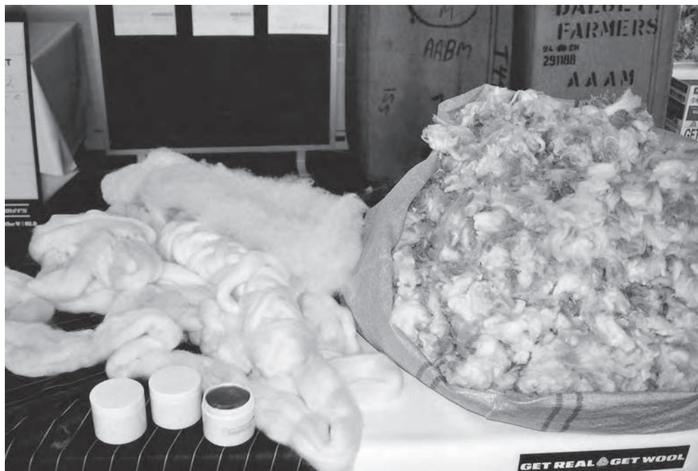
Post farm gate wool processing – branded bale, scouring, top making to final cloth and by-products (lanolin).
