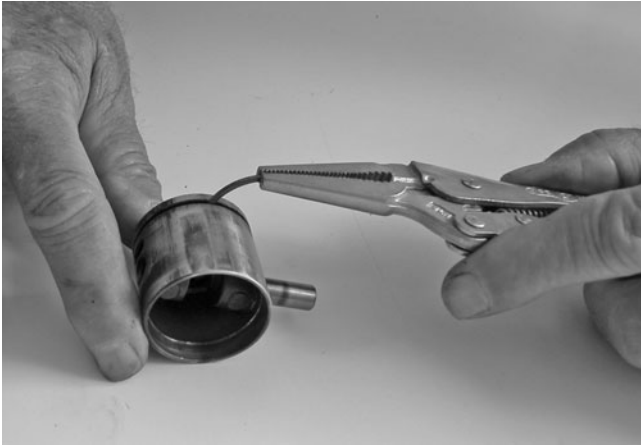
FIG. 6-11. Cleaning ring grooves prepares the piston to accept new rings. Robert Shelby
