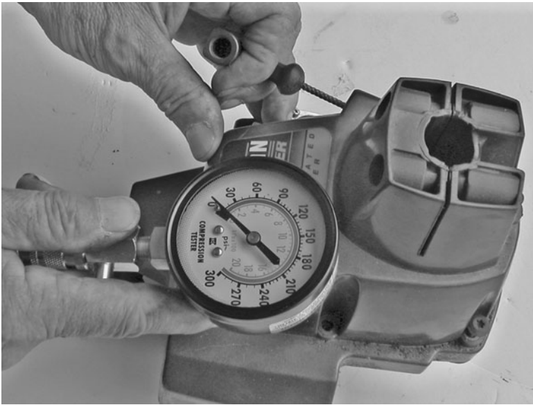
FIG. 2-11. Cylinder compression is a basic indication of engine health. Robert Shelby
