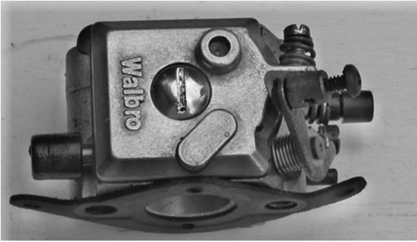
FIG. 4-5. Pumps on smaller carburetors usually are on the side opposite the metering diaphragm. Robert Shelby
