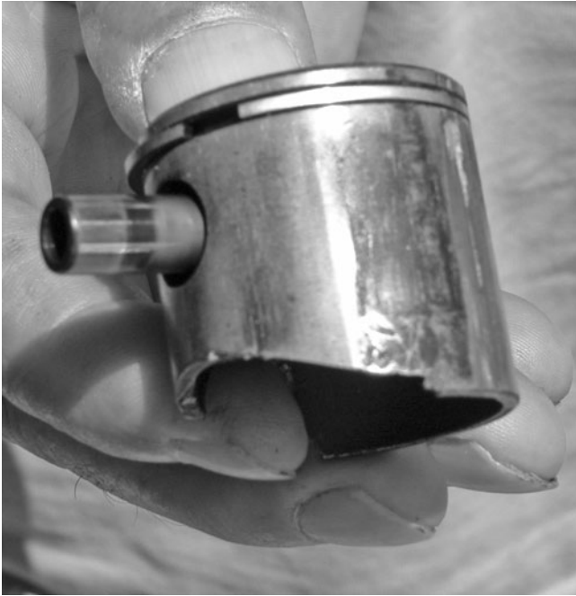
FIG. 2-8. High combustion temperatures are death on pistons. This example exhibits pock marks left by metal fragments, deep scores, and, near the crown on the right of the photo, weld splashes. Robert Shelby
