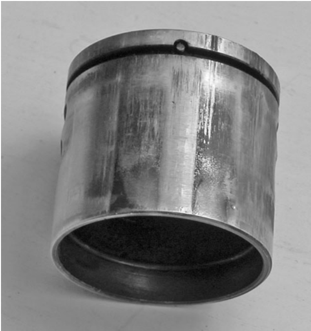
FIG. 6-14. This sort of damage calls for a new piston and cylinder. Robert Shelby
