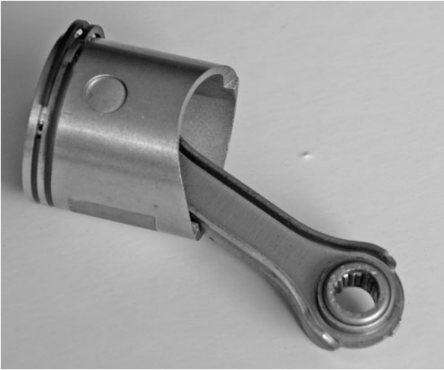
FIG. 6-8. If rings were free to rotate, the ring ends would snag on the ports. By looking closely, you can see the locating peg between the ends of the upper ring. Robert Shelby
