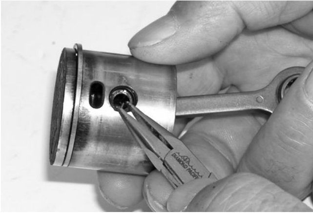
FIG. 6-16. Circlips with bent tangs are removed and installed with miniature long-nosed pliers. Snap-ring pliers, available from auto supply stores, are used to remove clips with pierced “ears.” Robert Shelby
