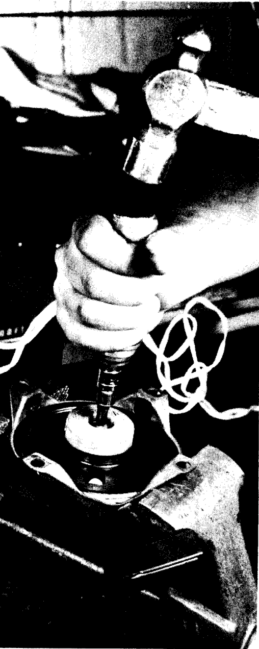
6-46. A hammer-actuated hand impact tool with a Phillips head loosens the lock screw.
