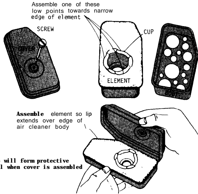
7-1. You saw this Briggs and Stratton polyurethane foam air filter in Chapter 5. Here it is again, disassembled for cleaning and oiling.
