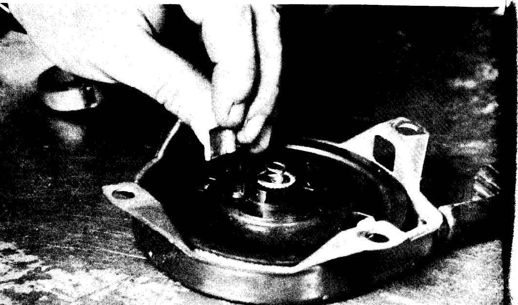
6-55. Starter dogs should be checked to see if they have good spring tension. If not, lift them out and install new springs.
