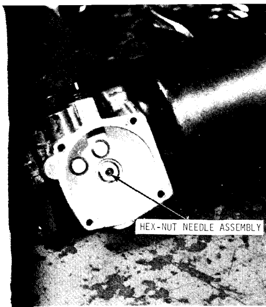
7-23 and 24. Left the diaphragm bears against a spring-loaded needle in the center of a hex-nut assembly. At right, you see the wrong way to remove the needle assembly. If the pliers slip they can damage the hex and possibly bend the needle.
