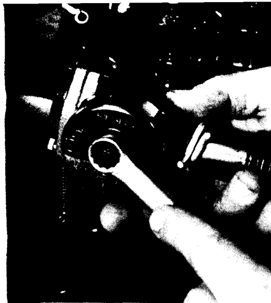
7-35 and 36. Remove the bolt that holds the carburetor bowl, as shown left. When the bolt is out, at right you can see that it also serves as a fuel jet. The tipoff is a tiny pinhole between the threads and the bolt head. Make sure this tiny hole is clear before reinstalling.
