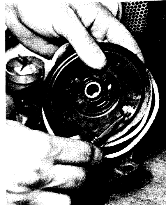
6-52 and 53. Twist the spring cover clockwise to disengage it from the pulley; then lift it away, as shown left. For this model, you can obtain a replacement cover with the spring installed. To install a new rope, just run the old one out through the hole, first digging it out with a small screwdriver.
