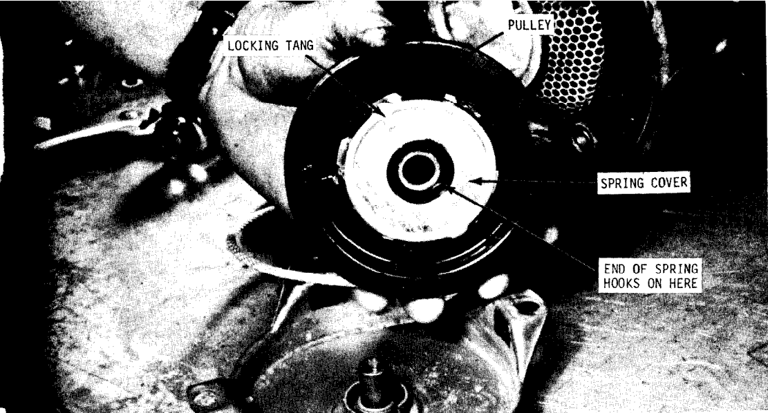
6-51. Next step is to lift the pulley up and out, exposing the spring cover, which is held by tangs that lock to the pulley body.
