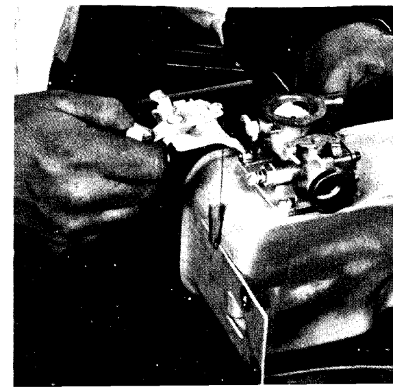
7-8 and 9. The bracketscrews come off next Then lift the bracket itself away This provides access to the mounting screw underneath
