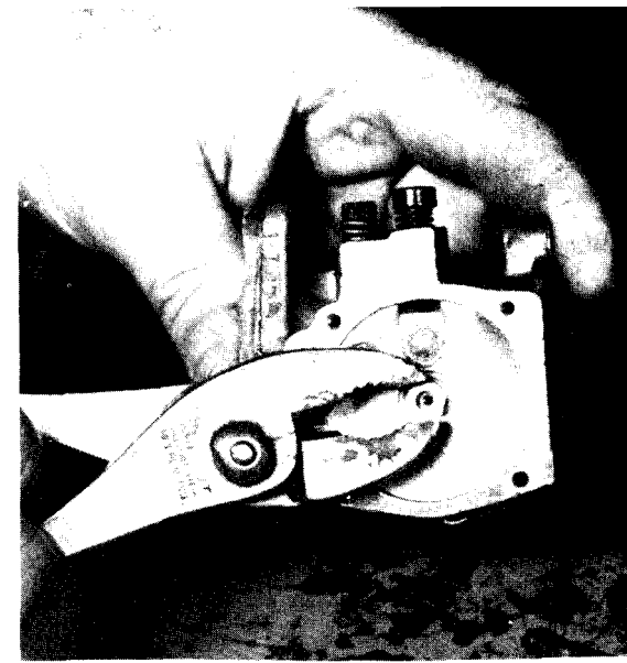
7-23 and 24. Left the diaphragm bears against a spring-loaded needle in the center of a hex-nut assembly. At right, you see the wrong way to remove the needle assembly. If the pliers slip they can damage the hex and possibly bend the needle.
