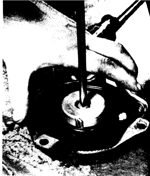
6-49. Once the screw is loose, it can be removed with an ordinary Phillips screwdriver.
