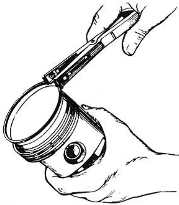
FIGURE 7-30. Installing a compression ring on an Onan piston with the aid of a ring expander. Expand the rings only enough to slip them over the
