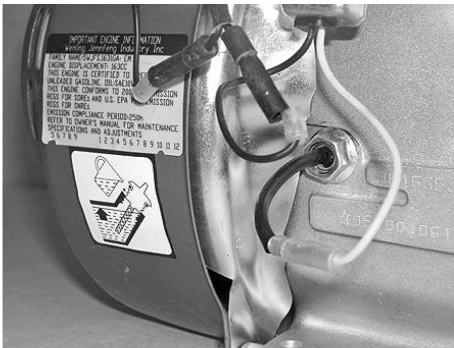
FIGURE 2-4. A wire running from the crankcase means that the engine is equipped with an oil-level monitor that illuminates a warning lamp or, as is most often the case, shuts down the ignition. Robert Shelby
