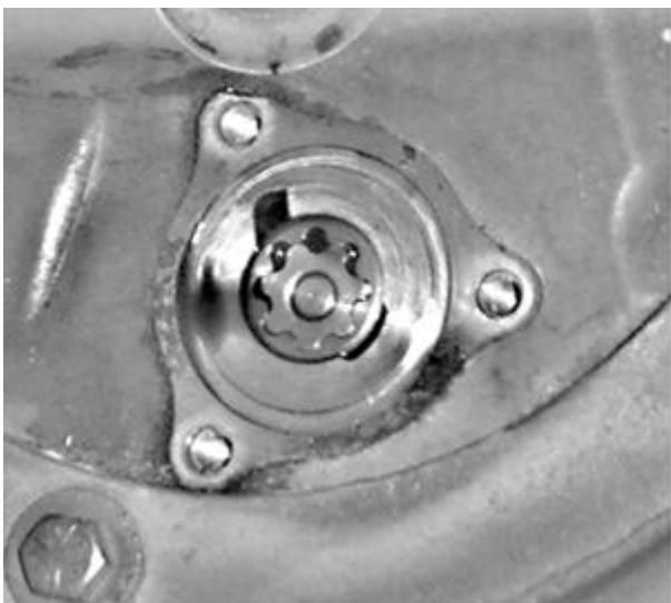
FIGURE 1-5. An Eaton-type oil pump of the kind favored by many small-engine
