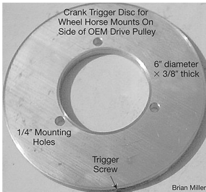
FIGURE 3-26. The aluminum timing disc mounts on the pto end of the crankshaft and uses a precisely located steel screw to excite the trigger
