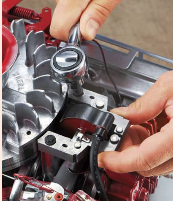
Replacing the Ignition
