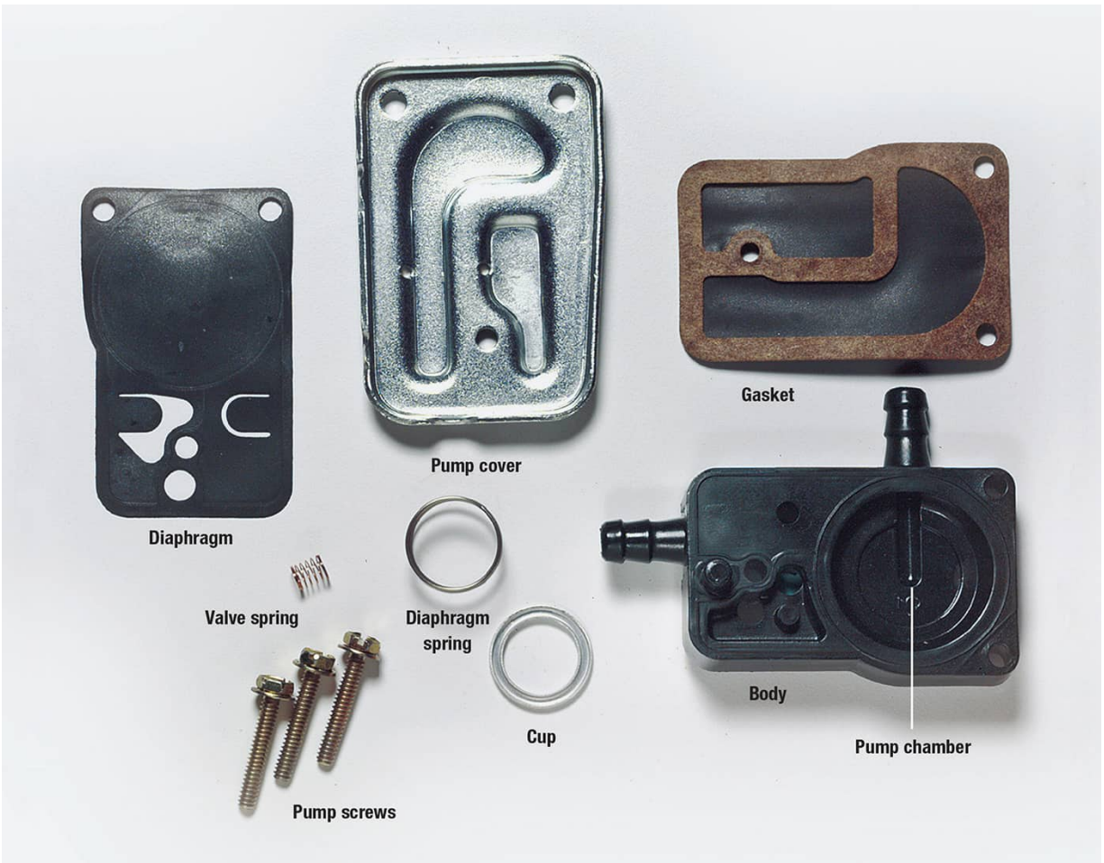
The parts of a typical small-engine fuel pump. The device relies upon vacuum pressure generated by the piston motion to advance the fuel upline from the tank.
