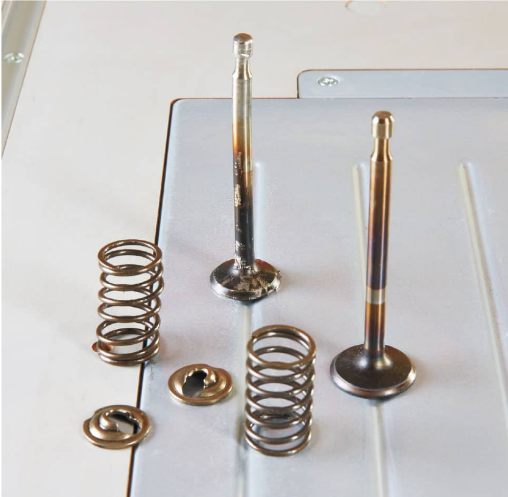
Small-engine valves are not big but their job is very important. A typical assembly includes the valve, valve spring, valve rotator, and valve spring retainer.
