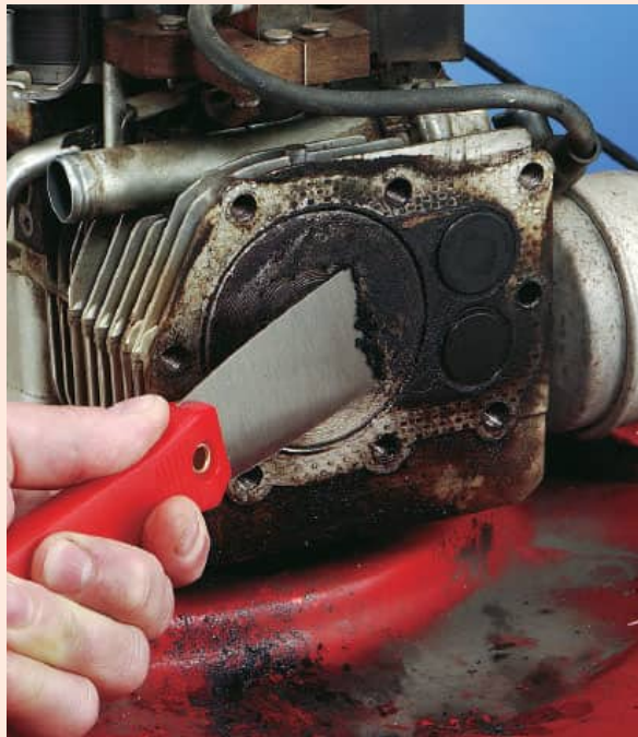
Removing Carbon Deposits
