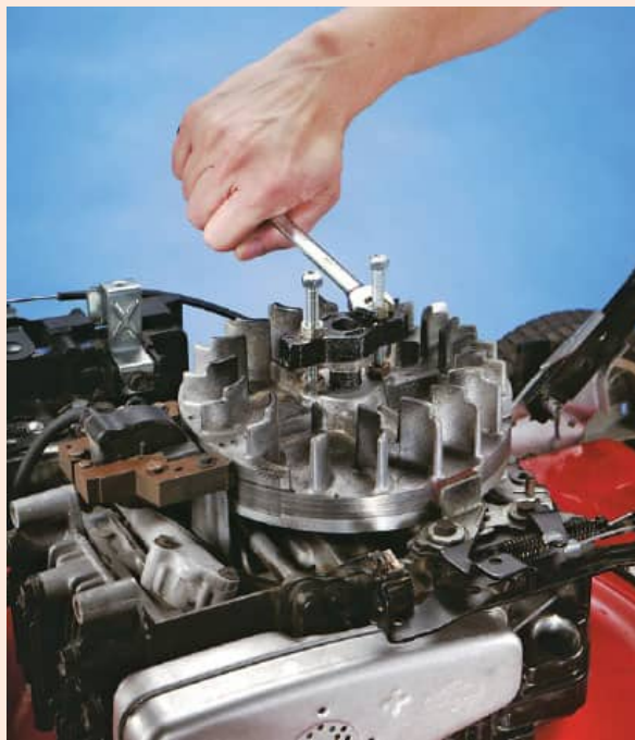
Inspecting the Flywheel & Key
