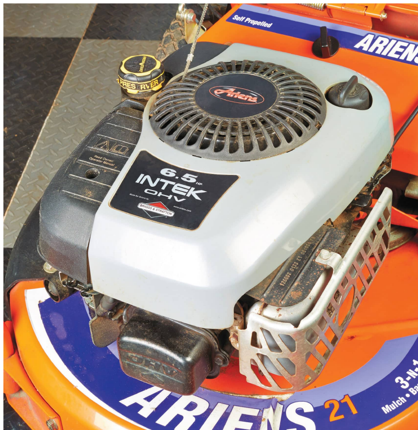
A typical 4-stroke, overhead valve gas engine. At 6.5 horsepower it is of average power for a lawn mower.
