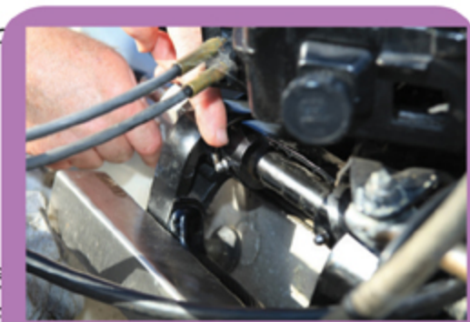
1. Typical throttle/shift linkage lubrication pivot points
