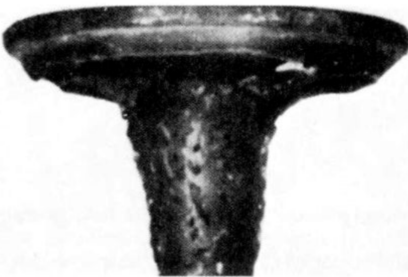
Fig. 6-13. Valve inspection: (D) gas channeling at valve face, probably caused by an improper valve grind; (E) heavy carbon buildup on intake valve, normal flow slow-turning engines, (valve usually can be reused after cleaning); (F) gum deposits from stale gasoline, one of the major causes of valve sticking (ream guides and clean valves).
