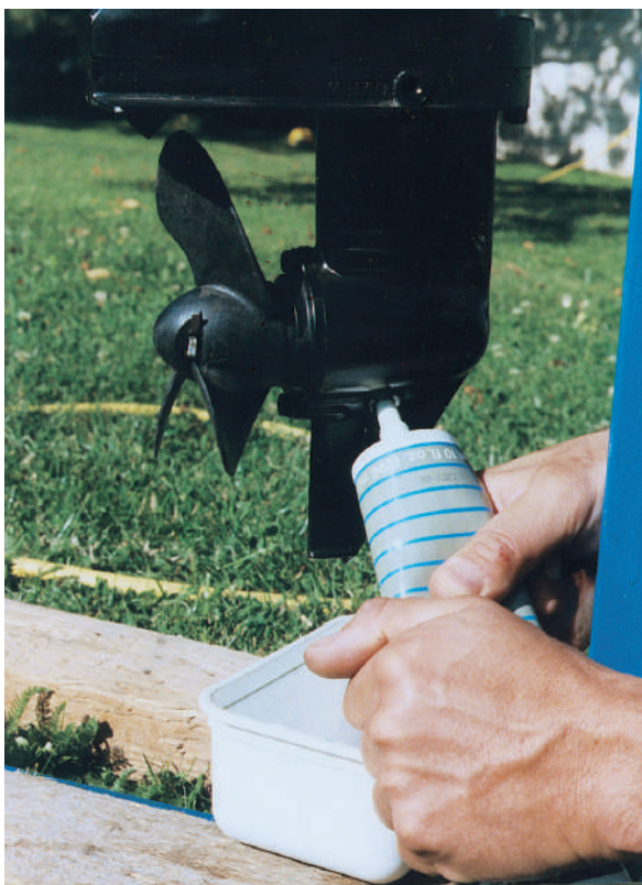
3 Make sure that the vent screw is removed before filling the gearbox with oil. The box is refilled through the lower hole with the engine in a vertical position.
