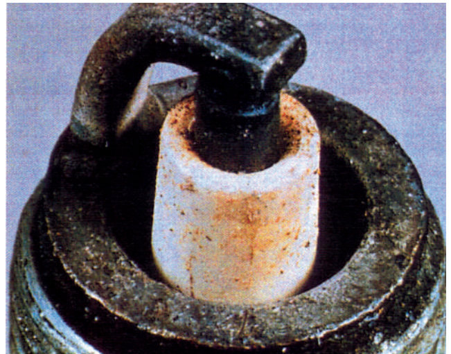
Overheated spark plug with a shiny insulator cone (Champion).
