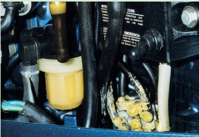
1 Check the condition of your filter regularly.
