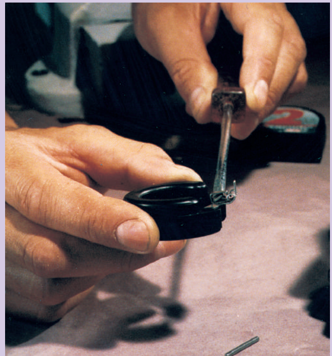
4 You can adjust the bowl level by bending the float bowl tab. Beware: this job is very delicate. Make small adjustments.
