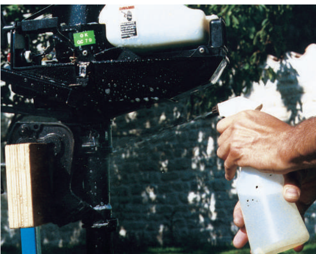
2 Spray the entire engine with detergent. Clean with a brush.
