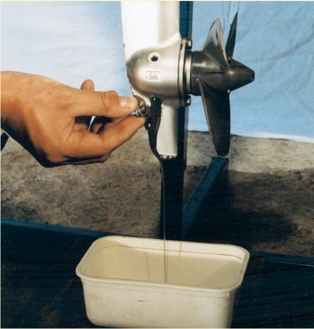
3 Remove the gearbox oil plug. Note the oil colour. A whitish colour is a sign of water in the oil.
