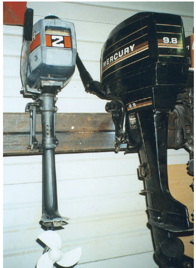
Whew! It's finished. It is best to keep the engine in a vertical position in a dry, well ventilated place.
