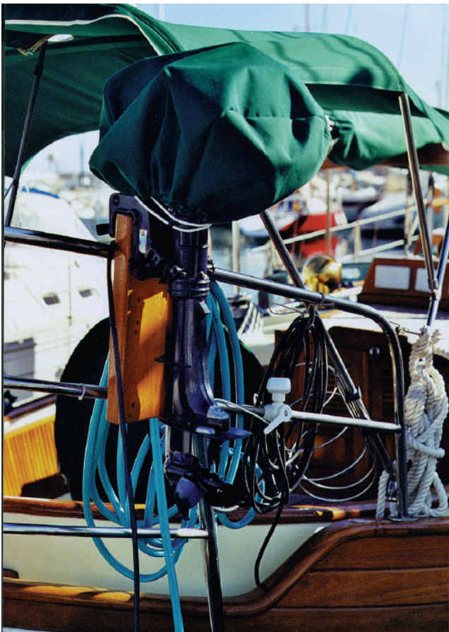
If you leave your engine on your boat's transom, consider protecting the power head with a cover. Don't use plastic covers.
