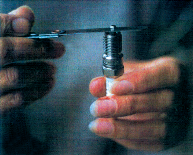
Electrode gap adjustment is done with a feeler gauge.
