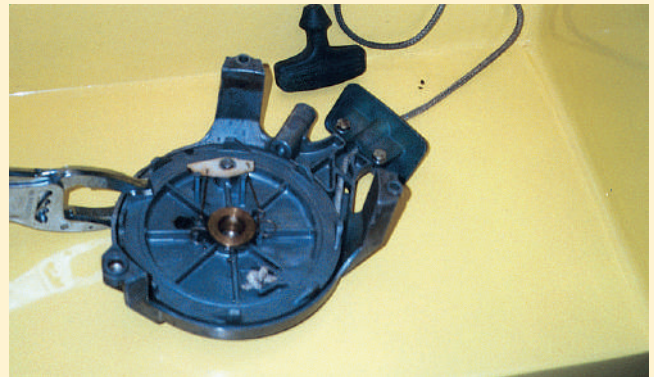
Lock the drum. A mole wrench or vice grip is good for this.
