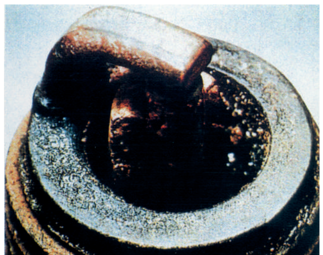
Broken insulator (Champion).
