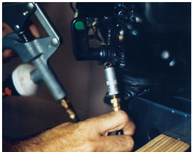
7 The engine has several grease points that must be lubricated using a grease gun and cartridge sold by your engine dealer.
