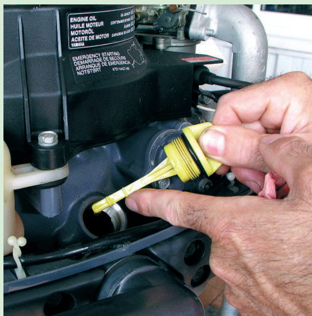
Check the oil level in a four-stroke engine regularly by unscrewing the oil cap and checking the dipstick.
