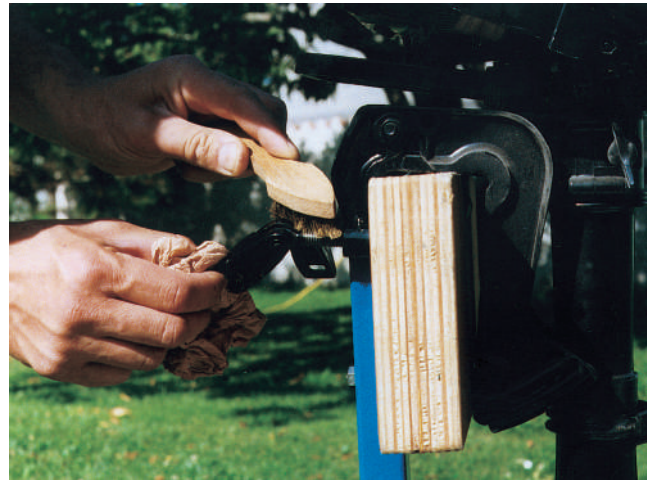
5 Check the transom clamp screws. A thorough brushing, followed by cleaning with petrol, will prevent any seizing.
