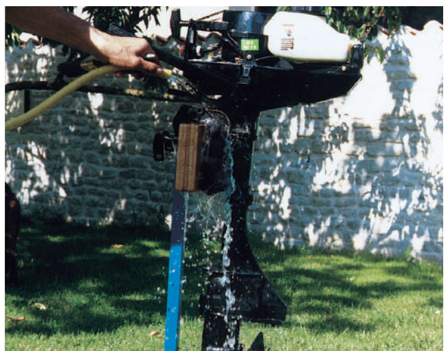
3 Be sure to thoroughly rinse the engine with a jet of fresh water. Dry it until every trace of moisture is gone.
