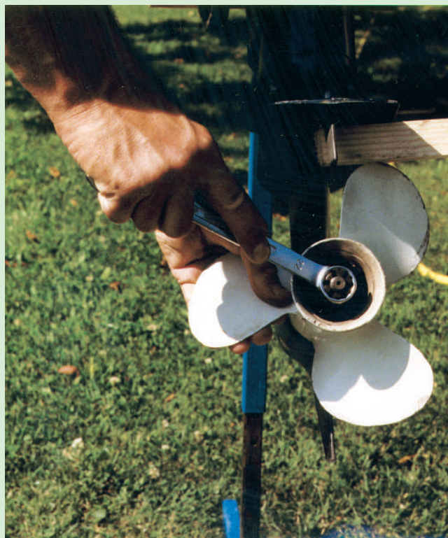
2 Put a block of wood between the anti-cavitation plate and the propeller blades to unlock the nut.
