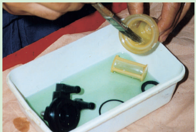
4 Clean the filter and the bowl with a brush and petrol. If possible, finish the cleaning by drying with compressed air.
