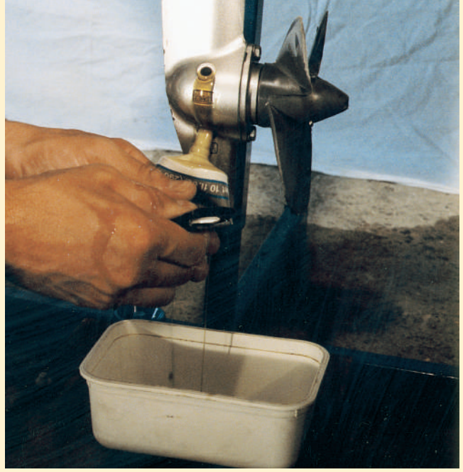
4 Fill the gearbox through the lower oil plug opening until there are no air bubbles coming out and the oil flows out of the upper opening.
