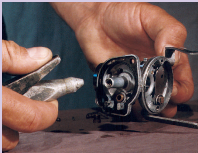
6 Clean with clean petrol, then blow into all the holes.
