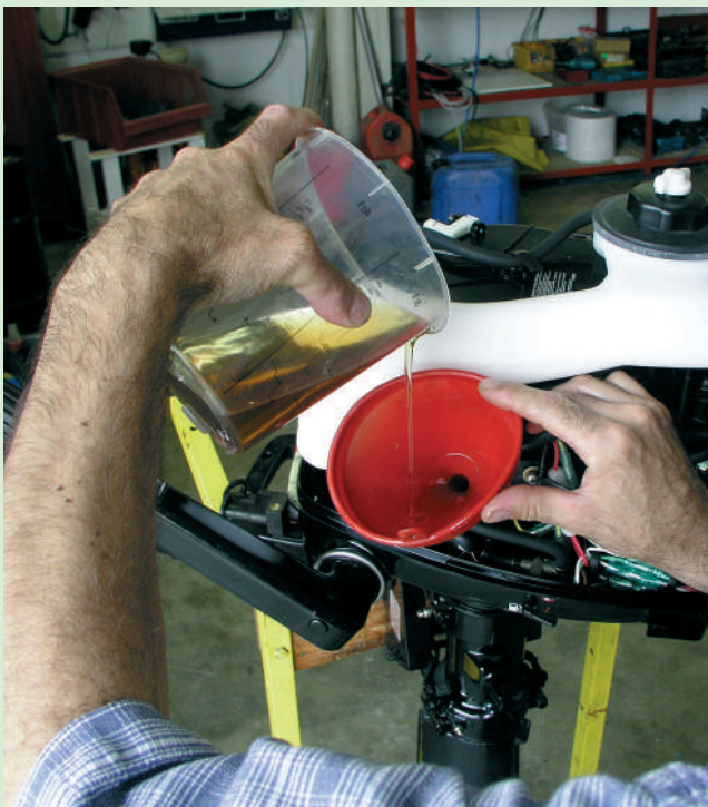
Use a funnel to avoid spills. Pour the new oil in slowly to aid flow and prevent overfilling.
