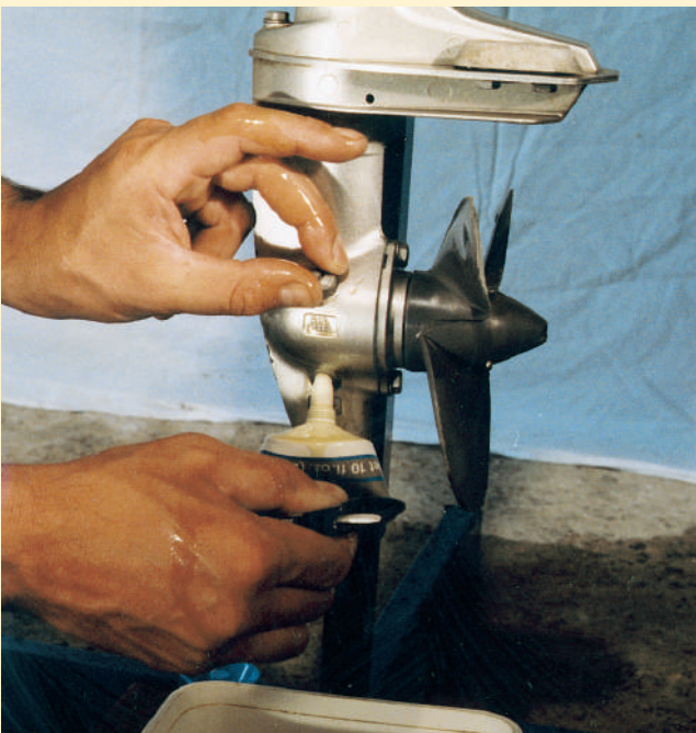
5 Screw in the upper plug, remove the tube and screw in the lower plug.
