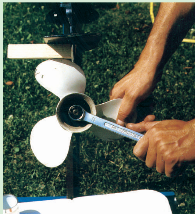
4 After cleaning and greasing the shaft, remount the propeller, screw the nut on, then install the split pin and bend the washer tab.
