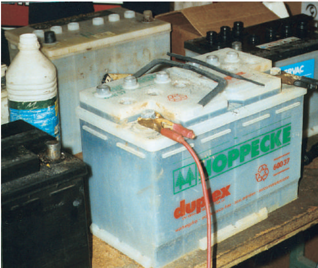
One more thing to check closely: the battery. Clean and recharge it before storing.
