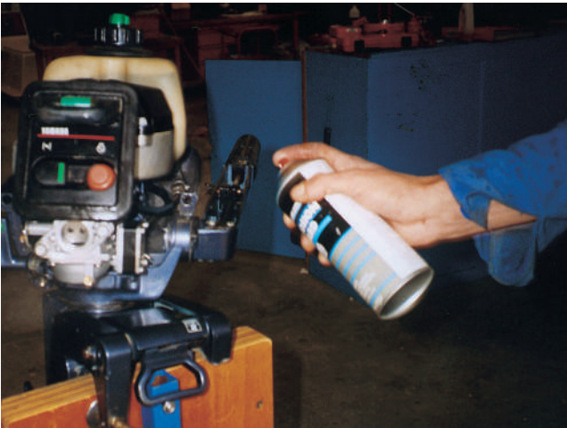
4 Spray the entire engine head with an external protection oil or penetrating oil.
