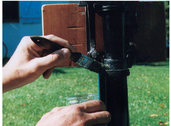
1 Grease the joints with a brush and marine grease.
