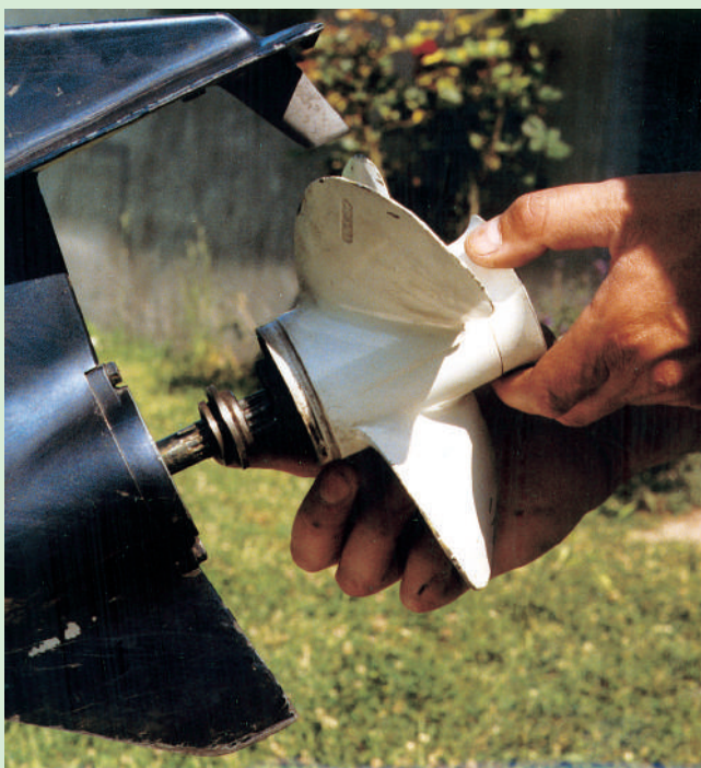
3 Tap the hub with a mallet, if necessary, to loosen it.
