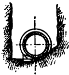
3. Trench in firm ground.
