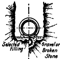
4. Trench in Rock.
