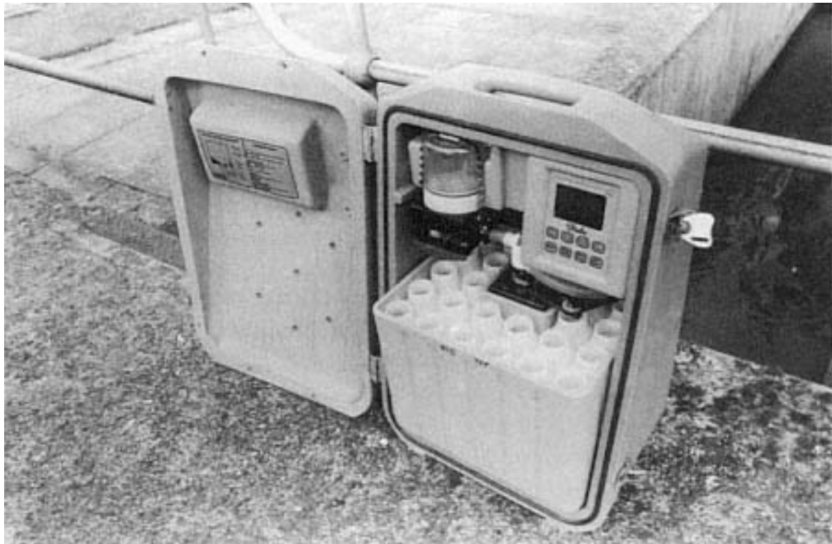
Figure 8.2 Portable sampler on site.
