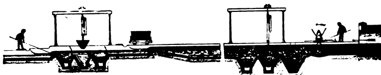
FIG. 5.—Schnependahl's System of Sieves and Detritus Tanks.
