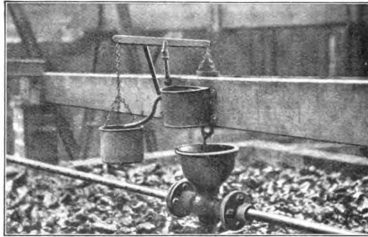
FIG. 106.—Apparatus for Feeding Candy Sprinkler intermittently at Leeds.
