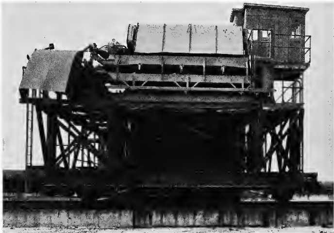
FIG. 206.—Transverse type of sludge-stripping machine at West Side works, Chicago.
