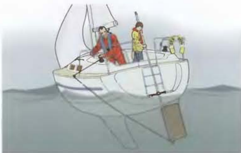
Jury rig a steering oar using the spinnaker pole and washboard or cabin locker cover.
