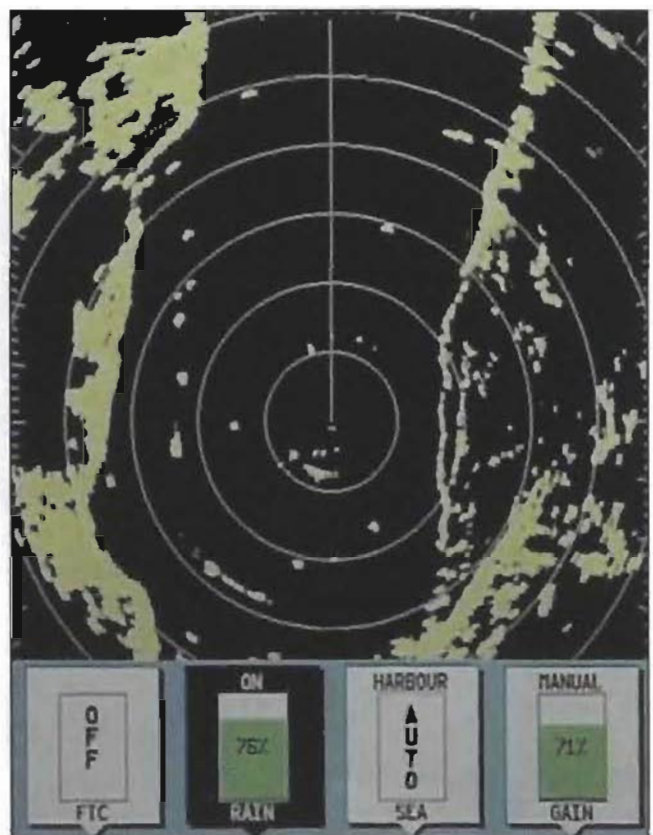
Coastlines with rain clutter control turned up: note how shelving coastline on right has been weakened
