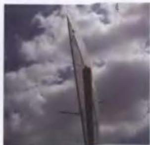
Hooked leech due to excessive kicker tension.
