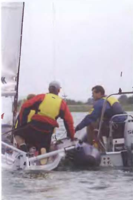
Recover the MOB over the forward beam between the two hulls. An exhausted MOB may find it easier to climb over the back beam.
