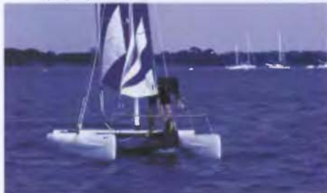
Recover the MOB over the forward beam between the two hulls. An exhausted MOB may find it easier to climb over the back beam.
