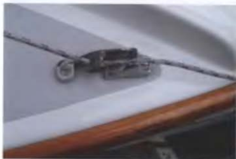
Reaching hooks are a simple way of holding the guy down and cleating it
