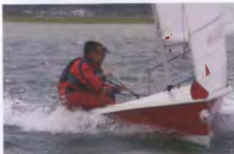
To bear away, ease main sheet and heel to windward
