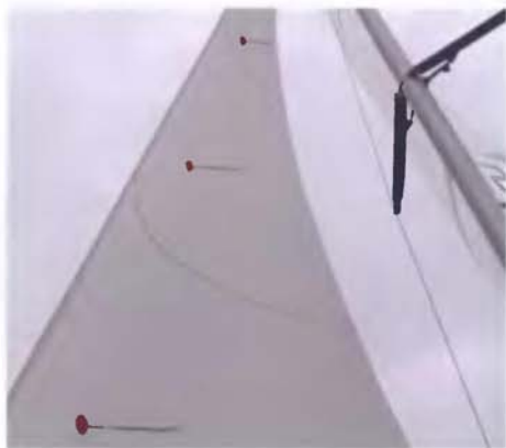
With perfect jib set-up, windward tell tales stream slightly upwards
