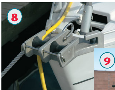
Left: Double bow roller. Below: CQR stowed in bow roller. Danforth stowed in bow-pulpit bracket.
