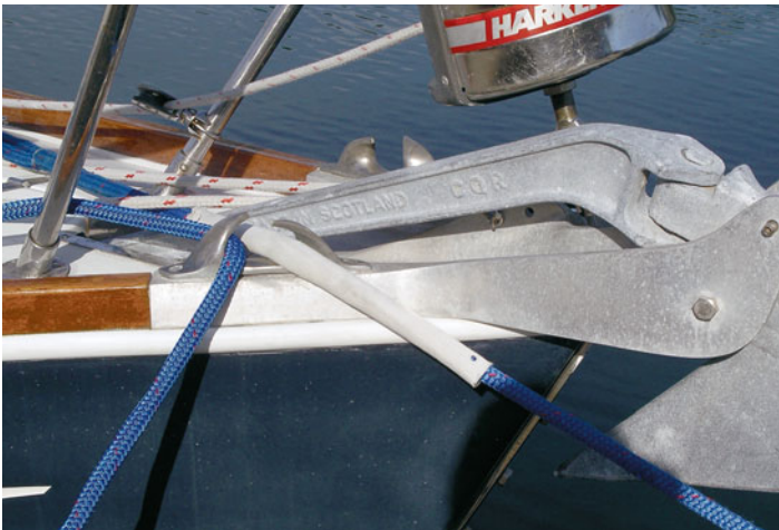
Chafe gear installed.
