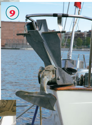
Left: Double bow roller. Below: CQR stowed in bow roller. Danforth stowed in bow-pulpit bracket.
