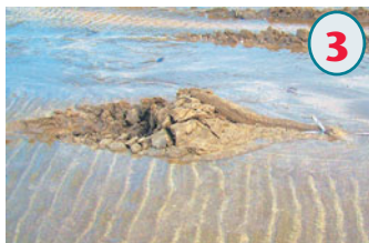
A plow anchor (in this case a Rocna) setting itself in firm sand during beach testing.
