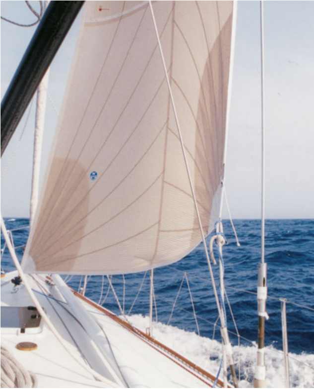
This storm jib's tack pendant should be longer.
