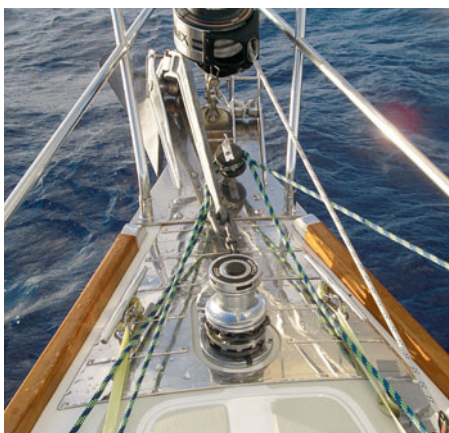
Multiple chafe points on foredeck.
