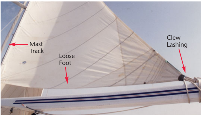
Storm trysail set on main boom and dedicated mast track.
