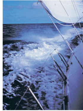
A fine, rail-down breeze. But when you heel this far, you should think about reefing.
