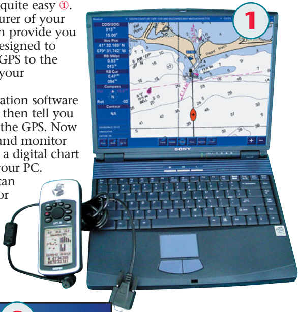
connecting cable for a Garmin handheld GPS
