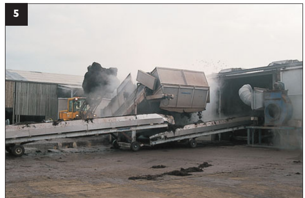
5 Bulk phase II compost being filled into the phase II room.
