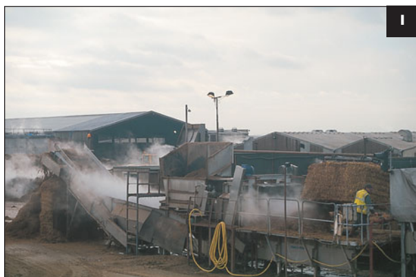
1 Straw bale breaker with a chicken manure hopper on a mixing line at the beginning of the prewet operation.
