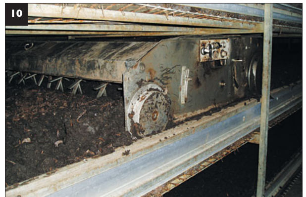
10 Equipment used to ruffle a shelf crop. The tines mix spawn-run compost with the casing. Photograph by kind permission of Brian Oxley.
