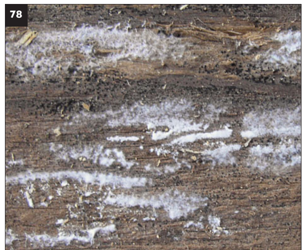
78 Trichoderma mould on wood, initially white in colour, but turning green as the spores are produced. A number of species can grow well, especially if the wood has not been seasoned or treated with preservative.
