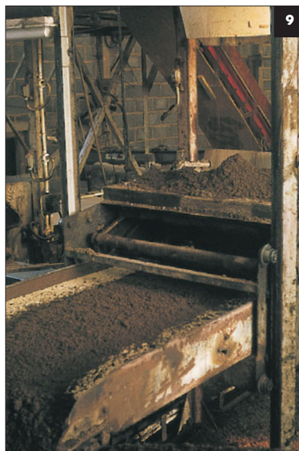
9 Casing application to trays.
