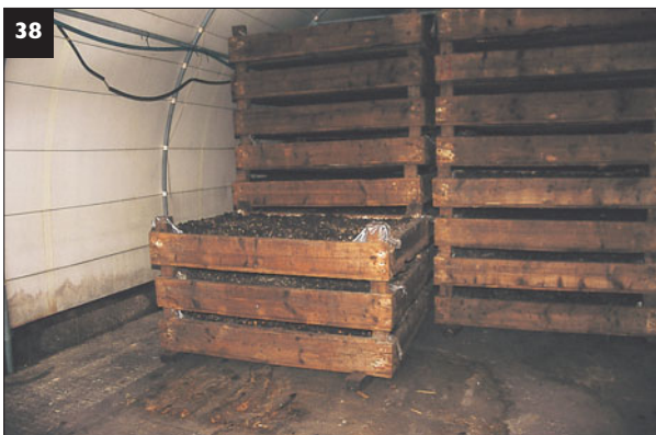
38 Trays stacked in a cook-out tunnel ready for treatment.
