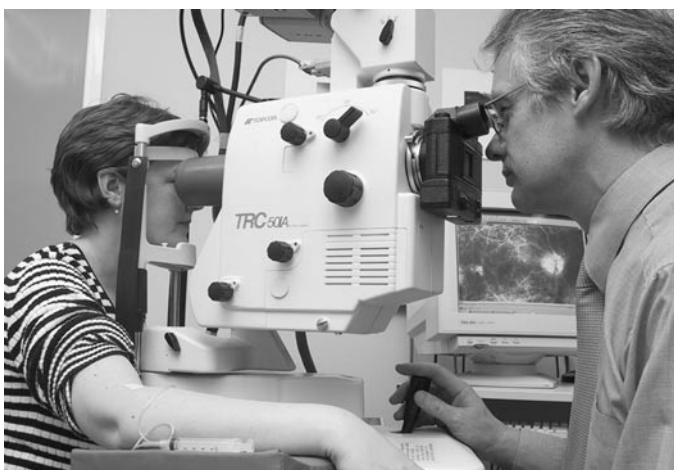
Fig. 31.17 A digital fundus camera images the retina following i.v. injection of fluorescein dye.
