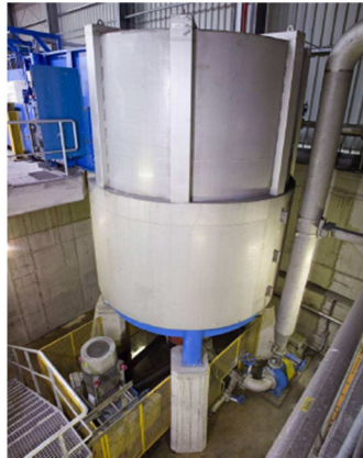
Figure 4.5 Andritz FibreSolve FSU high-consistency pulper.
