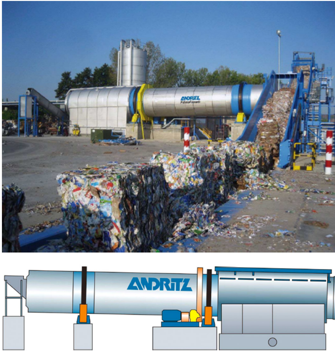
Figure 4.3 Andritz FibreFlow drum pulper. Source: Reproduced with permission from Andritz.
