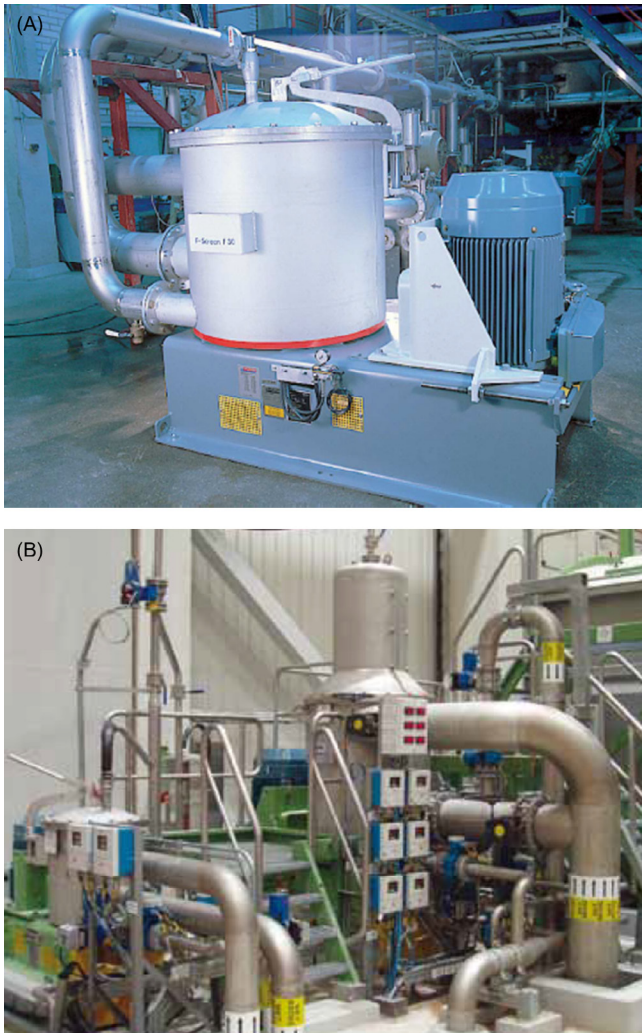
Figure 4.8 (A) Andritz ModuScreen F for coarse screening, (B) ModuScreen C&F screen for coarse and fine screening operations.
