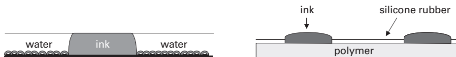
Figure 9.1. Illustration of an offset plate with ink and fountain solution (left) and a plate for waterless printing containing silicon rubber as non-image area (right).
