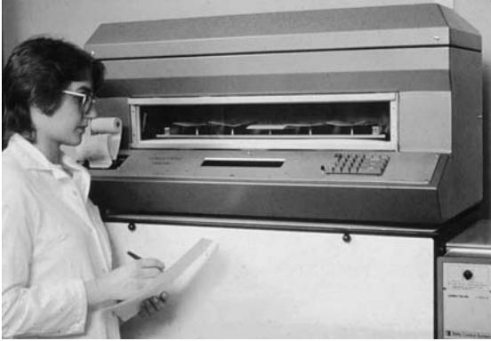
Figure 4.43. In the instrument the 100 mm by 100 mm samples are scanned by a laser gage and the three curl and twist components calculated.
