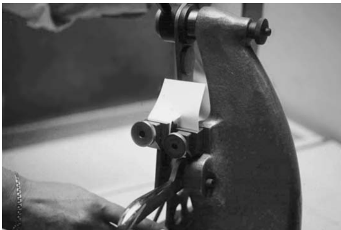
Figure 2.36. Tearing resistance according to Elmendorf.
