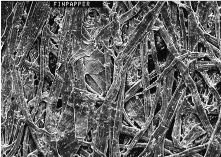
Figure 1.18. Fine paper, consists of chemical, undamaged fibres, which are often a mixture of hardwood and softwood. Note the filler particles. The pulp and structure is chosen mainly to give good opacity and surface properties.
