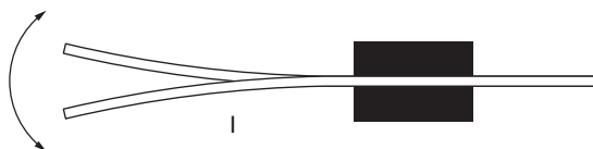
Figure 2.42. The bending stiffness for paper can be evaluated by determining the resonance length of the paper.
