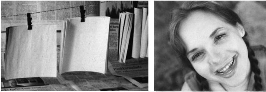
Figure 4.1. When adsorbing moisture, paper deform in different ways.
