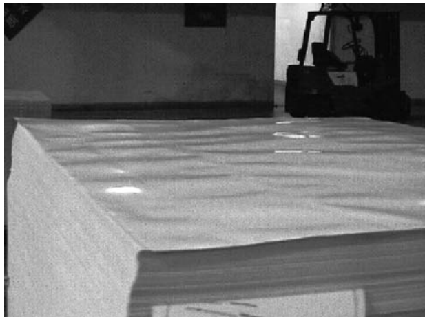
Figure 4.34. Cockling is out-of-plane movements locally over a paper.
