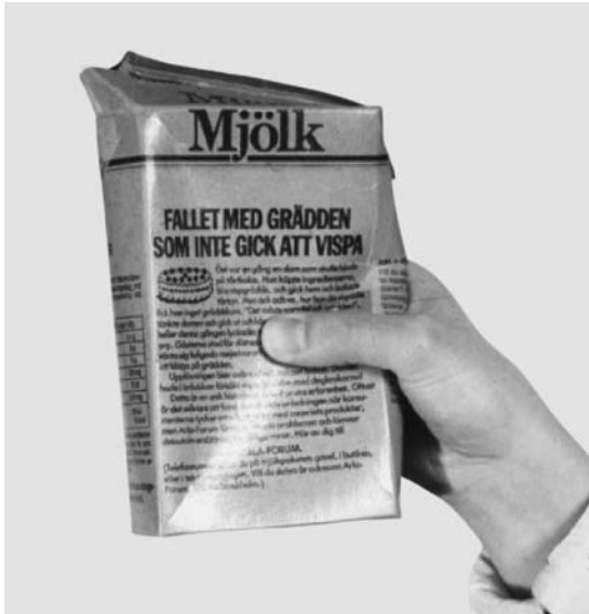
Figure 1.1. The bending stiffness is important for milk cartons as well as most paper grades.
