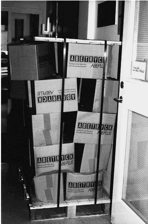
Figure 1.2. Compressive collapse of corrugated boxes after a long time of loading.
