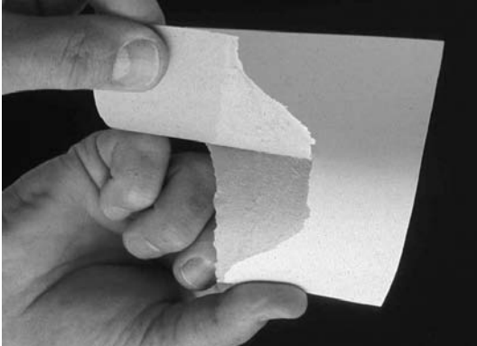
Figure 2.38. Tearing of thicker papers and highly oriented papers in the cross direction may be difficult to evaluate by the traditional tear method.
