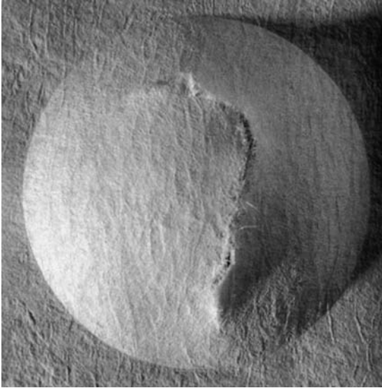
Figure 2.40. The fracture appearance in the Mullen test.
