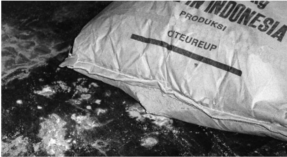
Figure 1.5. Break of a sack filled with cement.
