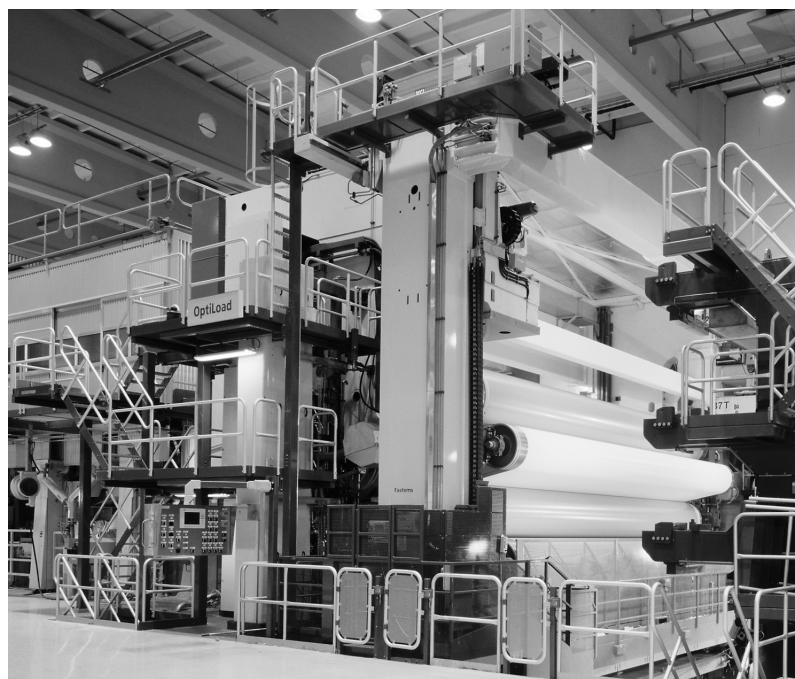
Figure 15.7. A multi nip soft calender installed on-line on a LWC paper machine (Haindl Papier) that started up 2000.
