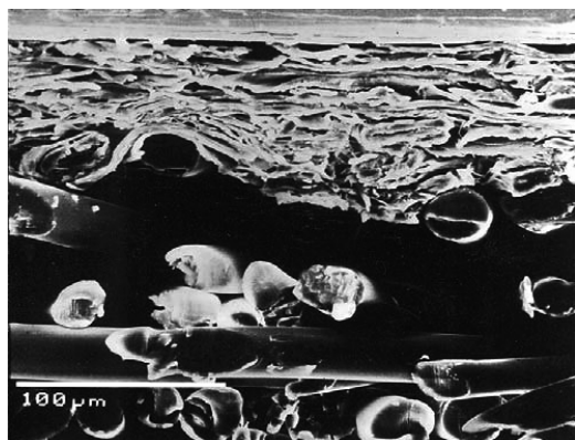
Figure 12.9. Press roll (top), newsprint sheet (middle) and press felt (bottom), (Beloit).
