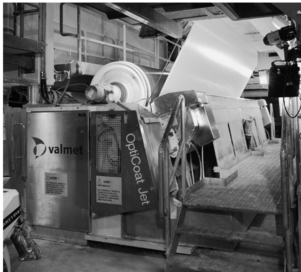
Figure 16.13. Blade coater. (Courtesy of Metso Paper Oy).
