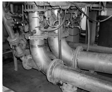
Figure 8.4. Thick stock mixing into white water flow on the FEX pilot paper machine.
