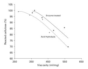
**Figure 12.14.** Reactivity of enzymatic pretreated pulp is higher at a given viscosity. The reactivity is measured according to a simulation of the viscose process (see chapter 9).
