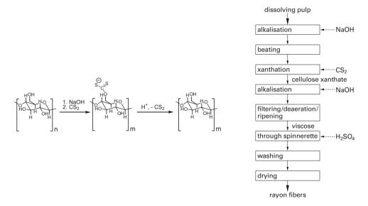
Figure 8.6. Process steps and chemical reactions encountered in the manufacturing of rayon fibers.
