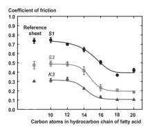
**Figure 7.20.** Coefficient of friction for paper impregnated with fatty acids of different chain lengths [8]. For paper the coefficient of friction will change with the number of slides. S and K stands for the static and kinetic coefficients of friction, respectively, and the number is the number of slides in the test.
