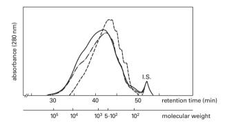
**Figure 9.26.** GPC of acetylated black liquor lignins from initial (--), bulk (-.-) and residual (--) delignification respectively. I.S. = acetone (internal standard). Calibration with polystyrene standards.
