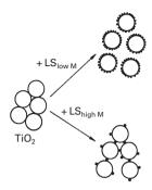
Figure 8.13. Schematic picture of the dispersing action on titanium dioxide pigment of lignosulfonates having an optimal ( $LS_{lowM}$ ) and a non-optimal ( $LS_{highM}$ ) molecular weight range. In the former case, a molecular weight range of 10000–40000 Dalton was found.
