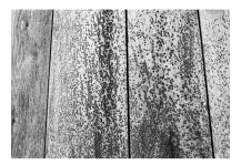
Figure 10.21. Heavy mould growth on untreated oak wood panels.
