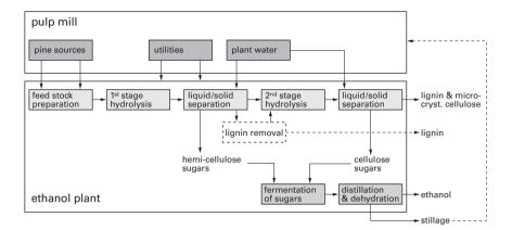
**Figure 8.18.** Suggested production unit for conversion of wood waste to ethanol using the CASH process employing sulfur dioxide and sulfuric acid in two stages. The integration with a pulp mill is indicated in the figure.
