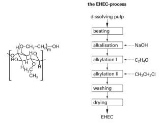
**Figure 8.9.** Process steps in the manufacturing of ethylhydroxyethylcellulose (EHEC) together with a simplified chemical structure of EHEC.
