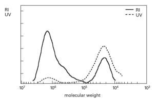
Figure 9.27. GPC of unbleached birch kraft pulp, dissolved in DMAC/LiCl. A series of pullulan standards were used for calibration and detection was done with UV-light at 295 nm and with refractive index (RI) respectively.
