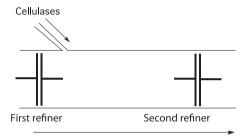
Figure 12.12. Cellulase treatment for decreased energy consumption in mechanical pulping.
