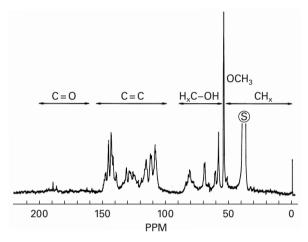
**Figure 9.19.**  $^{13}$ C NMR of milled wood lignin (MWL) from spruce. The regions of different types of carbon atom signals are denoted in the spectrum. (CH<sub>x</sub> = CH or CH<sub>2</sub>. S = solvent.)
