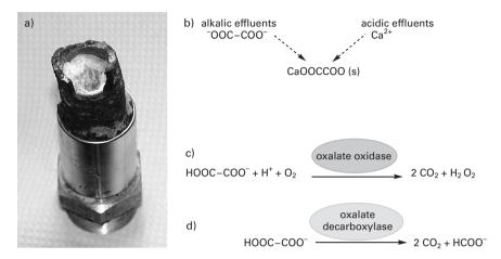
**Figure 12.16.** Enzymes degrading oxalic acid a) spray pipe with calciumoxalate precipitation. b) Principle behind precipitation. c) degradation of oxalic acid with oxalate oxidase d) Degradation of oxalic acid with oxalate decarboxylase.
