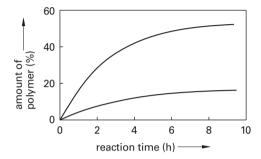
**Figure 8.11.** Radical initiated polymerization of vinyl chloride on bleached softwood kraft pulp. Amount of copolymerization (C) and homopolymerization (H) respectively.
