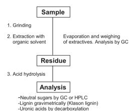
Figure 9.1. Analytical protocol for the analysis of wood and pulp samples.
