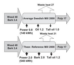
**Figure 8.24.** Energy balance (GJ/ton of pulp) in the average Swedish pulp mill in the year 2000. Comparison with a theoretical Reference Mill. Data from the Final Report of "The Ecocyclic Pulp Mill" (STFI 2003).
