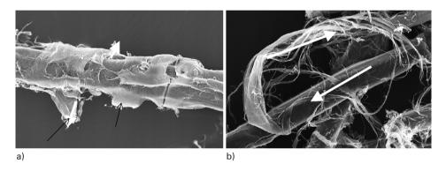
**Figure 3.18. Importance of the wood cell wall layers in pulping.** a) When wood fibres are refined the primary wall is often removed and the S1 layer becomes fibrillated (arrows); b) If refining is severe, fibrillation may also occur within the S2 layer. The orientation of fibrillation (arrows) reflects the MFA of the original wall layer.
