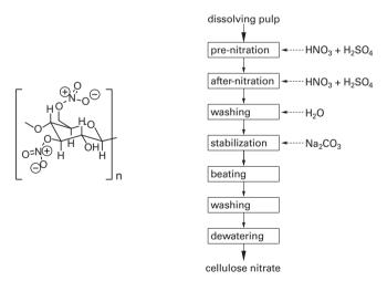
Figure 8.10. Process steps in the manufacturing of cellulose nitrate together with a simplified chemical structure.
