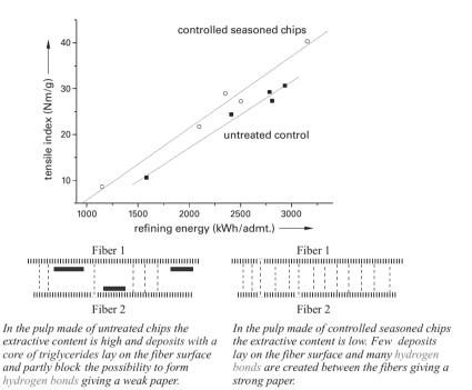
**Figure 12.5.** Effect of controlled seasoning on paper strength of thermomechanical Scots pine pulp. The graph above shows that the tensile strength is higher at similar refining energy for controlled seasoned chips than the untreated control. Thus a fungal pretreatment may save energy, or alternatively produce a stronger paper. The cartoon below shows a hypothesis for the mechanism behind the effect. For a discussion of the complex strength developments in mechanical pulp, see Volume 2.
