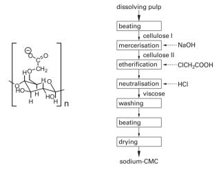
Figure 8.8. Process steps in the manufacturing of carboxymethylcellulose (CMC) together with a simplified chemical structure of CMC.
