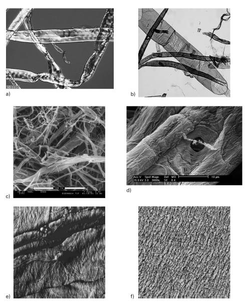
**Figure 9.29.** Light microscopy of a) pine kraft pulp  $(100\times)$  and b) aspen kraft pulp  $(200\times)$ . ESEM of c) spruce TMP, 50–200 mesh  $(500\times)$  and d) pine kraft pulp  $(3000\times)$ . AFM of e) fiber surface  $(5\times5~\mu\text{m})$  and fibrillar aggregation  $(1\times1~\text{mm})$ , aggregate dimensions 17 nm) (Courtesy: Joanna Hornatowska, STFI-Packforsk AB).
