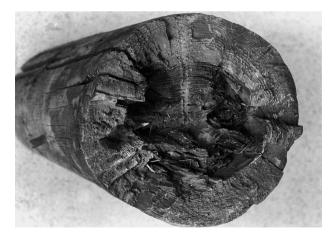
Figure 10.16. Severe soft rot attack in a preservative treated transmission pole has resulted in a brash fracture.
