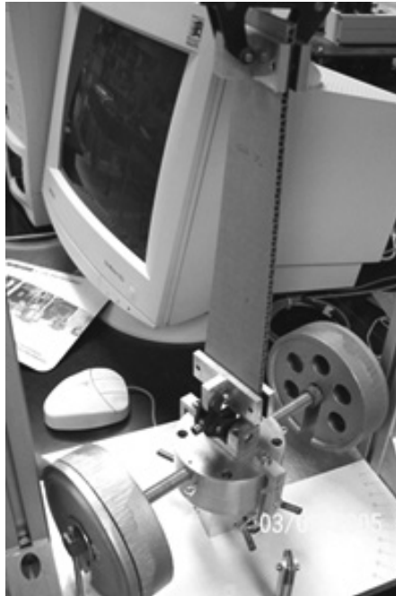
Figure 5.15 Torsion pendulum measurement of the twisting frequency of a corrugated board strip in the MD
