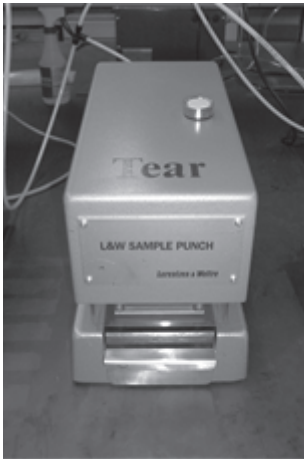
Figure 7.3 Punch and orientation of samples for the tear test
