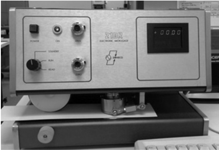
Figure 6.16 Stylus profilometer (Emveco 210-R) developed for the prediction of linerboard printability
