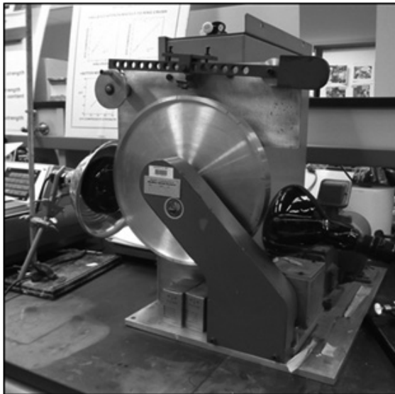
Figure 6.3 Bristow wheel equipment
