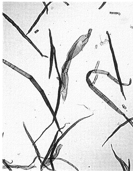
FIGURE 6.4. Northern hardwood bleached kraft (aspen) fibers. Magnification: 50 \times (courtesy of Integrated Paper Services).
