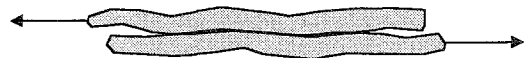
FIGURE 6.14. Cohesiveness is the resistance to shear provided by the hydrogen bonding of fibers during drying.
