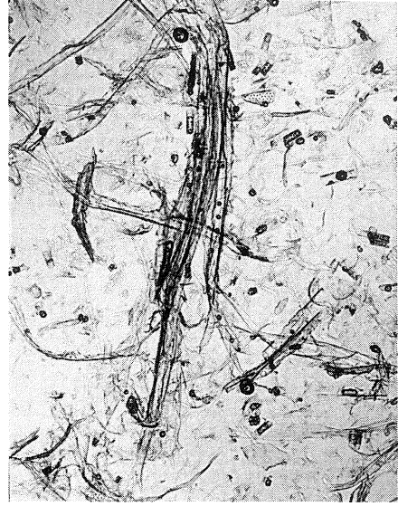
FIGURE 6.7. Northern softwood stone groundwood fibers (spruce and fir with trace of hardwood). Magnification: 50x (courtesy of Integrated Paper Services).
