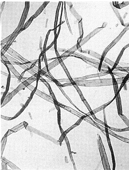
FIGURE 6.6. Northern softwood bleached kraft fibers (mostly spruce but mixed with some pine and others). Magnification: 50x (courtesy of Integrated Paper Services).
