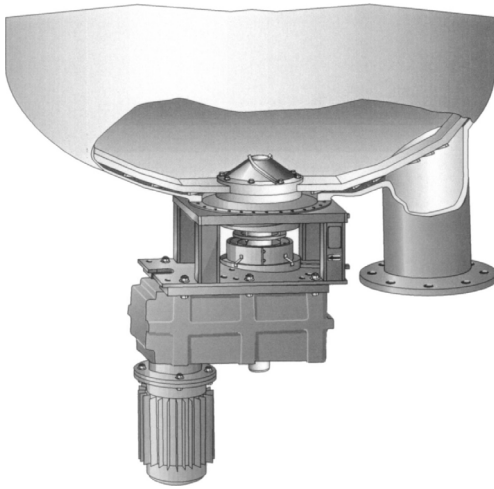
Fig. 7.17 Metso FlowScraper for medium consistency discharge [17].
