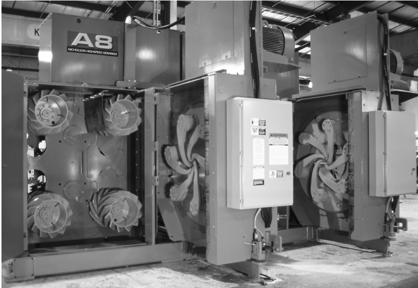
Fig. 3.8 Nicholson A8 Debarcker with tandem debarking rings [15].
