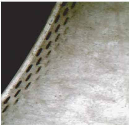
Figure 2.48 Elongational flow of fibers through small screen holes showing how different fiber structures can form.
