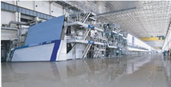
Figure 10.2 Operators' view from the wet end toward the dry end of a high-capacity paper-making line nearly 600 m long. (Source: Voith.)
