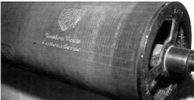
Figure 1.16 Dandy roll with soldered watermarks.
