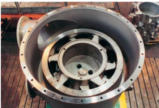
Figure 7.38 Example of a cylindrical screen with opened housing, showing the cylindrical screen and foil rotor. (Source: Voith.)
