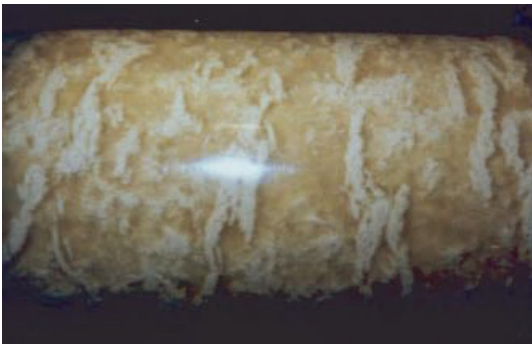
Figure 2.45 Plug flow with flocs rolling along the pipe wall at a lower velocity.
