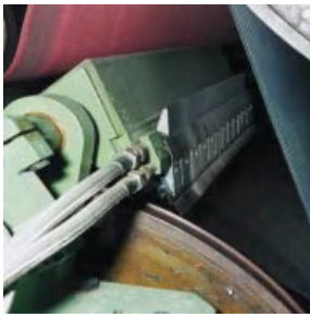
Figure 16.21 Ropeless tail threading in double-tier dryer sections by doctors with air nozzles. (Source: Voith.) (RM).
