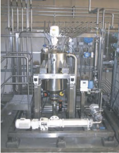
Figure 5.37 Continuous preparation of coating colors. (Source: BVG).
