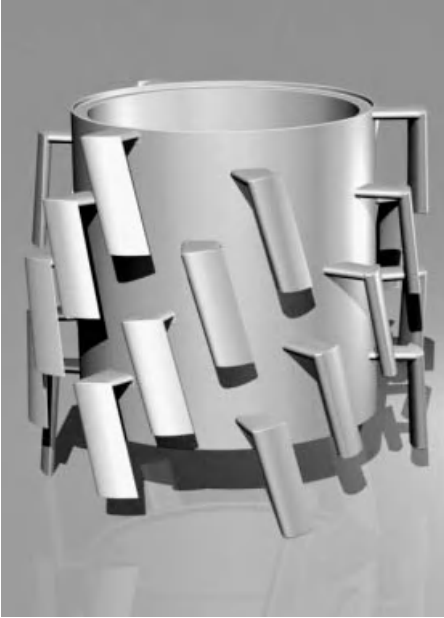
Figure 7.53 Rotor of a fine screen. (Source: Voith.)
