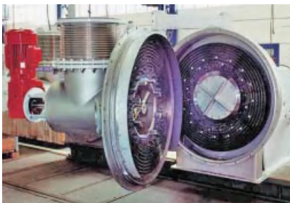
Figure 7.156 Disk disperser opened to show the fillings on rotor and stators. (Source: Voith.)
