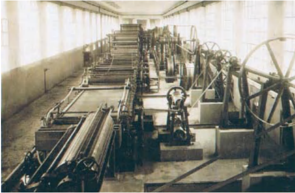
Figure 10.8 Central drive for a 183 cm wide paper machine in 1911.
