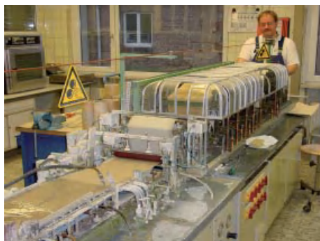
Figure 4.10 Pilot machine used for starch application trials.
