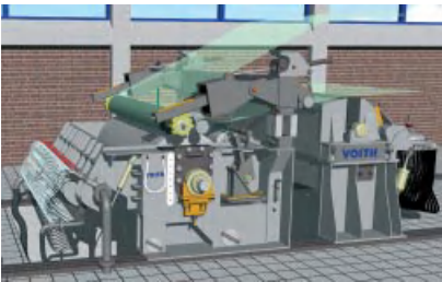
Figure 20.23 Cylinder mold sheet forming principle for banknote paper production. (Source: Voith.)
