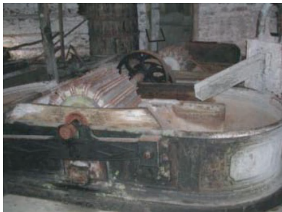
Figure 1.11 Hollander beater, cast iron tub, Papeteries de Vaux, Payzac (France), about 1860.
