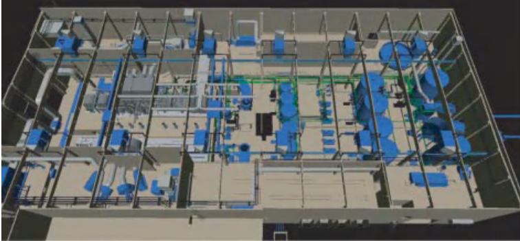
Figure 26.9 3D model of a plant with two 2 lines in one common building.
