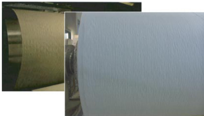
Figure 23.15 Typical appearance of cockling on a reel.
