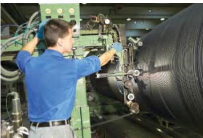
Figure 10.34 Extrusion of rubber cover. (Source: Voith.)
