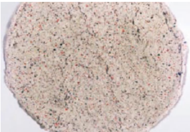
Figure 9.19 Rejects from LC cleaning.
