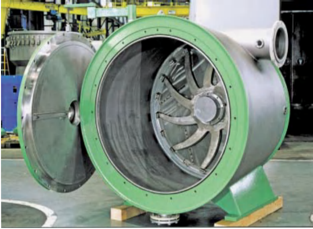
Figure 7.47 Opened disk screen for coarse screening. (Source: Voith.)
