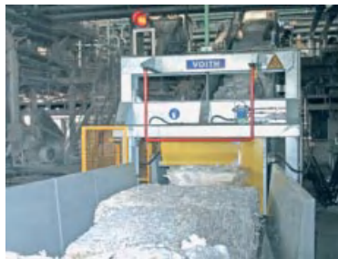
Wire cutting machine for recovered paper bales to feed an LC pulping line
