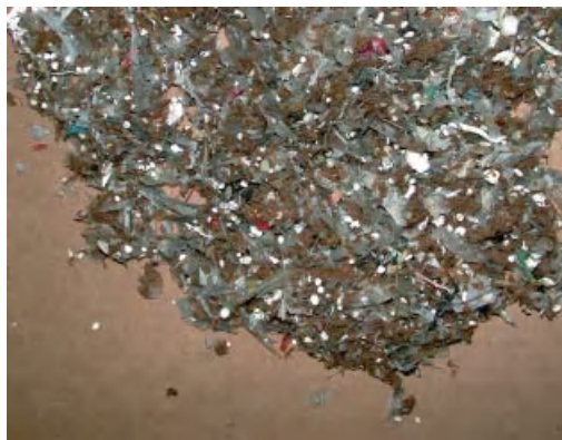
Figure 9.18 Rejects from hole screening.
