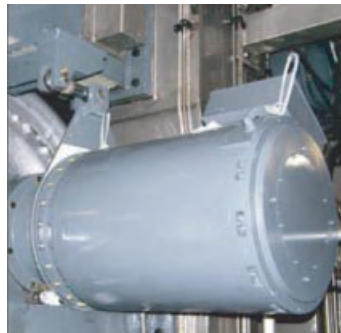
Figure 10.9 Directly coupled drive and the roll shaft. (Source: Voith.)
