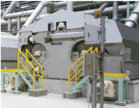
Figure 7.133 Example of a high-speed belt filter with two center rolls. (Source: Voith.)
