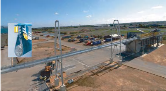
Figure 9.29 Pocket conveyor for long distance pickup at multiple locations allowing complex routing.
