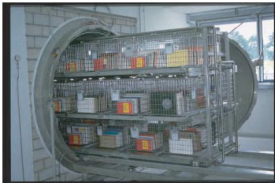
Figure 30.6 Chamber of the Papersave mass deacidification plant with a capacity of 60 t per year.
