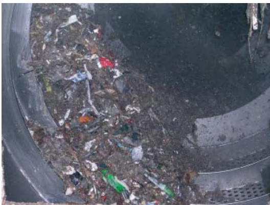
Figure 9.15 Typical rejects from drum pulper.
