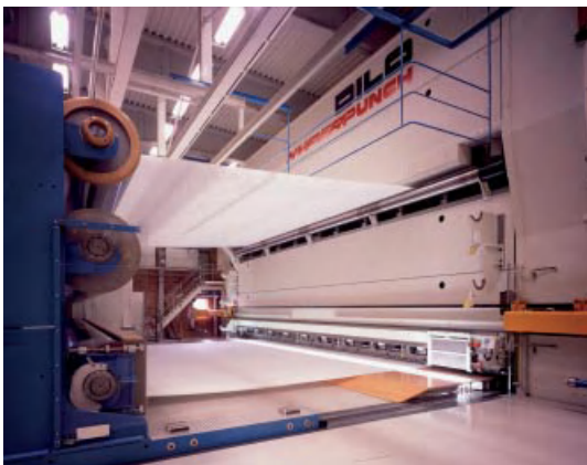
Figure 11.8 Finishing needle machine for press felt production.
