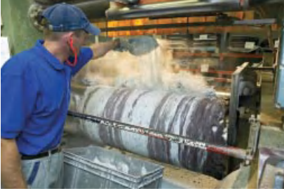
Figure 10.33 Rubber compounding on an open mill. (Source: Voith.)
