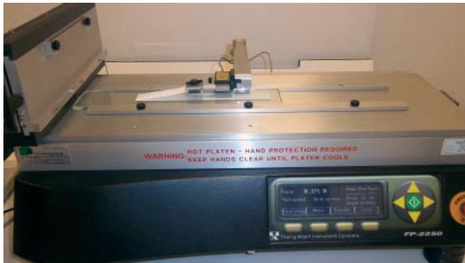
Figure 24.34 Peel adhesion using an equipment of the Thwing-Albert Instrument Company.
