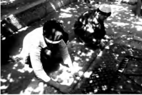
Figure 1.5 Felting: rolling up the mat covered with wetted layers of multicolored wool. Hotan (China), 1993.
