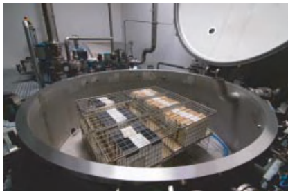
Figure 30.8 Treatment chamber of the ZFB:2 mass deacidification plant (annual capacity ~100t of paper).
