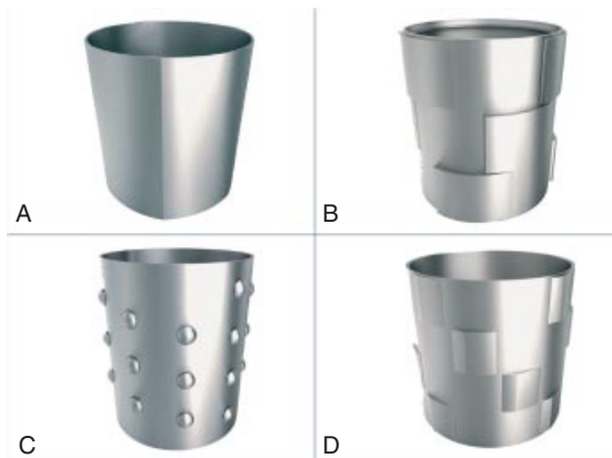
Figure 7.49 Different types of rotors for coarse screening. (Source: Voith.)
