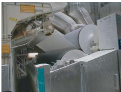
Figure 10.32 Example of film coating. (Source: Voith.)
