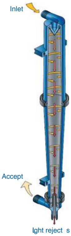
Figure 7.77 Light weight cleaner with unidirectional flow principle. (Source: Voith.)
