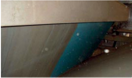
Figure 11.23 Cleaning result of a high water pressure cleaner for dryers. (Source: Voith.) (a) Contaminated and (b) clean fabric with blue color.
