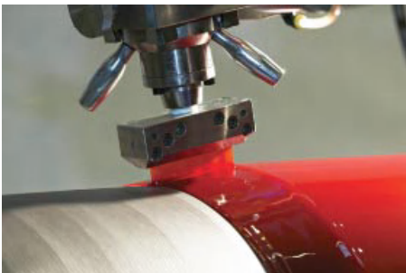
Figure 10.36 Moldless rotational casting of polyurethane cover. (Source: Voith.)
