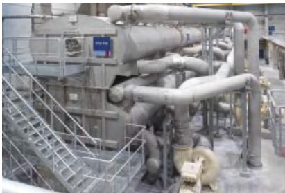
Figure 7.96 Photo of a flotation cell with horizontally arranged cells. (Source: Voith.)
