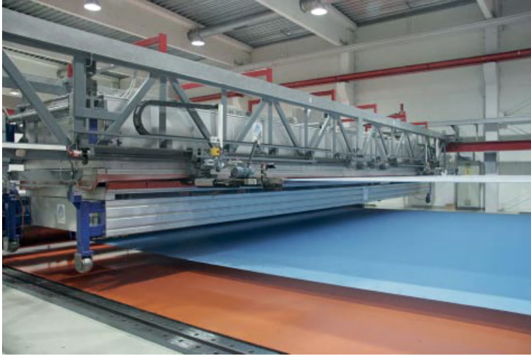
Figure 11.5 Forming fabric heat-setting machine. (Source: Voith.)
