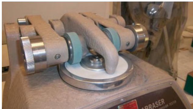
Figure 24.31 Abrasion tests using a Taber equipment.
