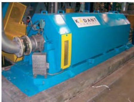
Figure 7.80 Cleaner with rotating housing. (Source: KADANT Inc.)
