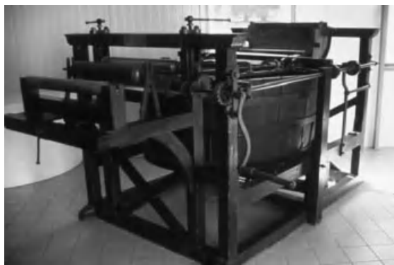
Figure 1.12 The Robert paper machine (reconstruction, University of Grenoble).
