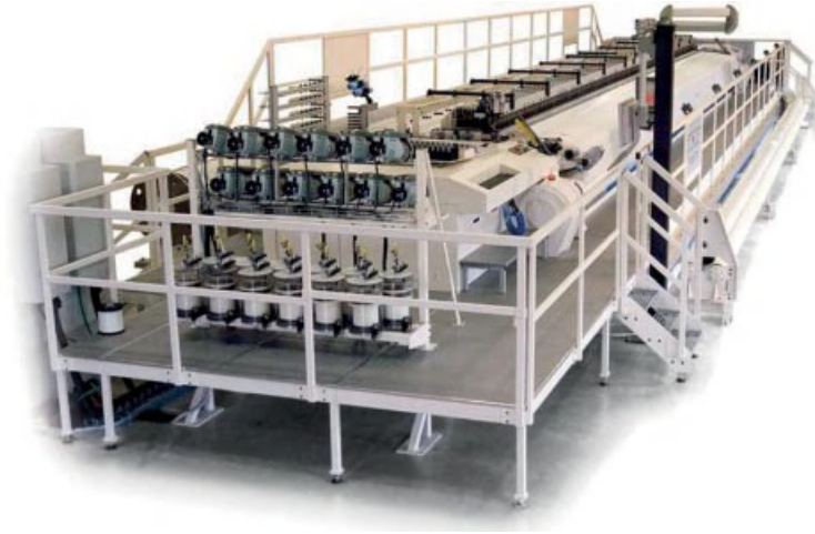
Figure 11.3 TransCent TCR rapier loom. (Source: TEXO AB.)
