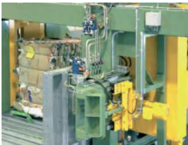
Dewiring machine for recovered paper bales to feed an HC pulping line
