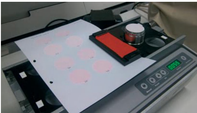
Figure 24.30 Abrasion tests using a Quartant abrasion tester of the company Prüfbau.
