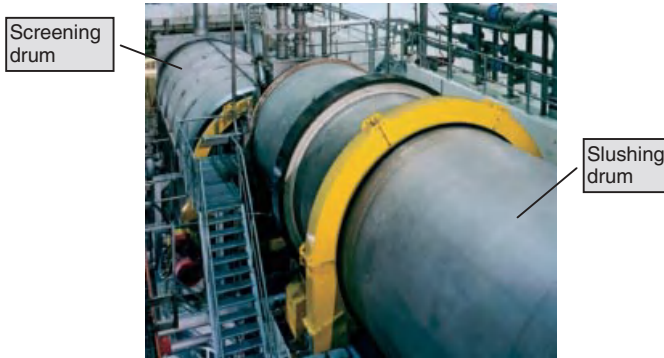
Figure 7.24 Photo of a drum pulper with separate slushing and screening drums. (Source: Voith.)
