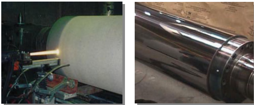
Figure 10.38 Plasma coating of press roll. (Source: Voith.)
