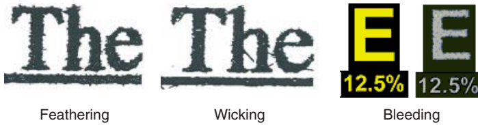
Figure 24.52 Important effects in the assessment of the sharpness in print outlines in inkjet printing – feathering, wicking (according to [34]), and bleeding [35]
