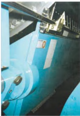
Figure 16.22 Tail threading in single-tier dryer sections by air nozzles installed in the doctor holder. (Source: Voith.)
