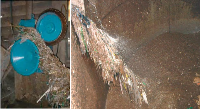
Figure 7.19 Ragger for trash removal and trash tail in an LC pulper. (Source: Voith.)
