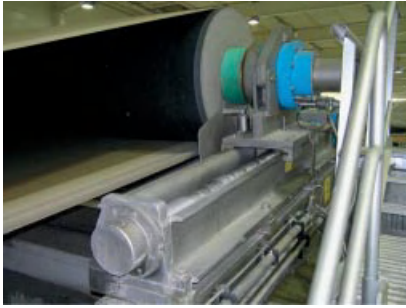
Figure 11.14 Press felt stretcher with stretch roll, spindle, and slide rails. (Source: Voith.)
