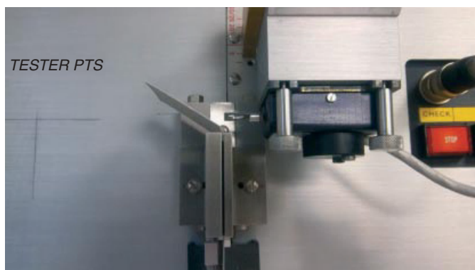
Figure 24.29 Determination of technical quality of creasings using an equipment of the Company Lorentzen & Wettre.
