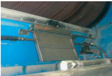
Figure 10.26 Perforated reel drum and device for safe tail threading in a single-tier dryer section. (Source: Voith.)
