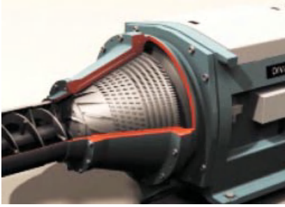
Figure 7.157 Disperser with conical fillings. (Source: Metso.)
