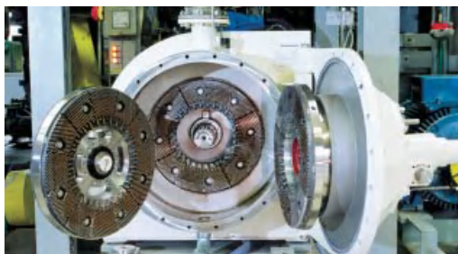
Figure 7.149 Example of a double disc refiner opened showing the fillings. (Source: Voith.)
