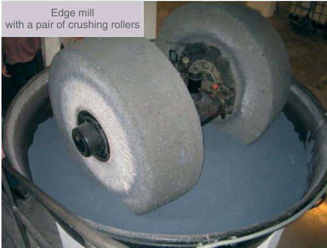
Figure 7.15 Edge mill as an obsolete disintegrating (and fiber beating) machine.
