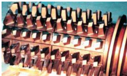
Figure 7.162 Filling of a kneading disperser. (Source: Voith.)
