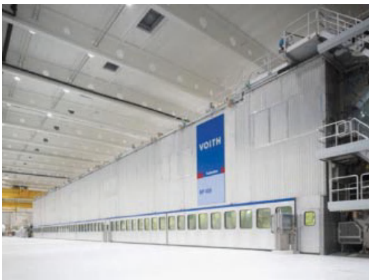
Figure 16.26 View on a closed dryer hood with windows and doors to be opened for inspection. (Source: Voith Krieger.)
