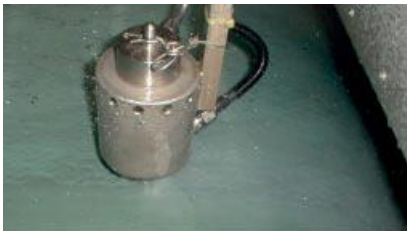
Figure 11.20 Rotating cleaning head for forming fabrics. (DuoCleaner™, Source: Voith.)
