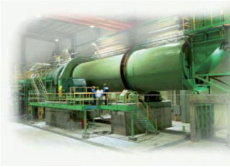
Figure 7.22 Single drum pulper with slushing and coarse screening in one drum body. (Source: Andritz.)
