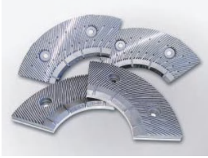
Figure 25.3 Pattern of a refiner filling showing the bars. (Source: Voith.)
