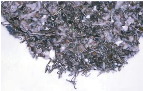
Figure 9.17 Rejects from HC cleaning.
