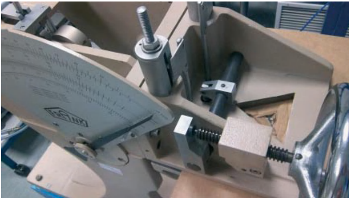
Figure 24.33 Overhead view of puncture energy test for corrugated board using an equipment of the Frank Company. (view to the clamped tested sample.)
