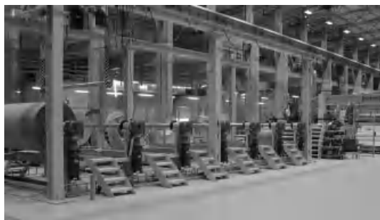
Figure 21.10 Conventional roll wrapping machine.
