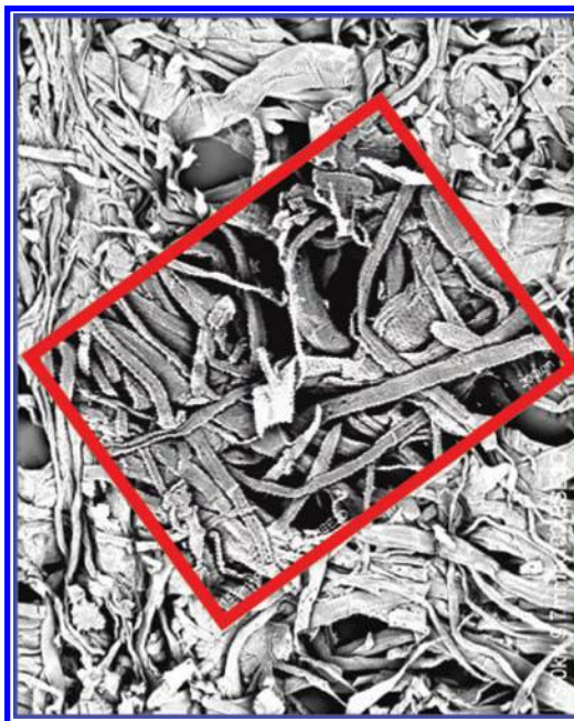
FIGURE 1.1 Paper structure by electronic microscopy (magnification \times 35 and \times 80 in red frame).
