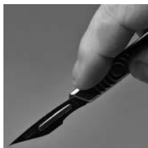
A scalpel is here shown held in the standard position for cutting. For safety reasons, be sure to always keep your non-cutting hand topside of your cutting hand.
