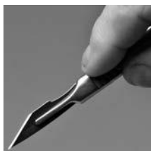
A craft knife makes an excellent tool with which to create a fold. Held upside down against the edge of a ruler, it does not cut the card along the length of the fold line, but compresses it.
