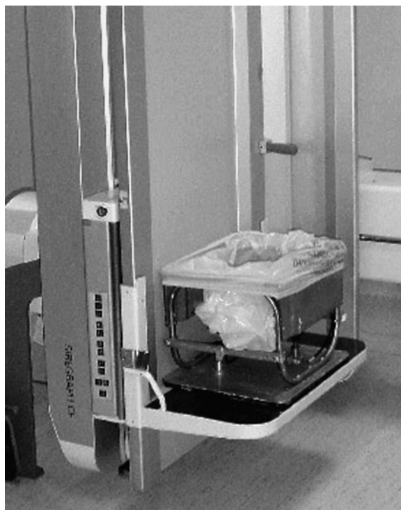
Fig. 4.1.1. The proctography commode placed on the footrest of the upright fluoroscopy table. Note the copper sheet immediately subadjacent to the seat, in order to balance radiographic contrast
