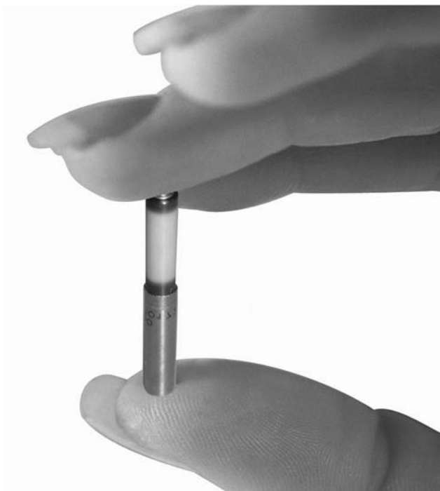
Fig. 4. The bion microstimulator.
