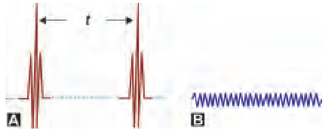
Figures 1.1A and B: Two types of diagnostic ultrasound waves. (A) Pulse wave (PW): 1/t is repetition frequency; (B) Continuous wave (CW)
