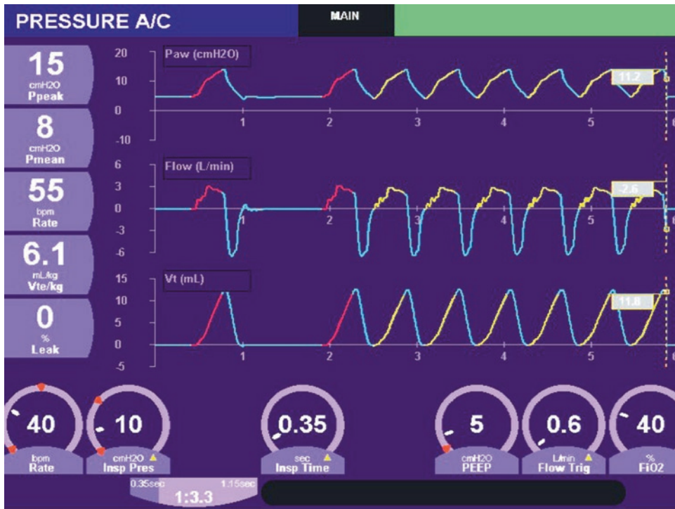
Fig. 22.9 Assist/control. Red shows a time-cycled machine delivered breath during apnea, yellow shows patient-initiated breaths
