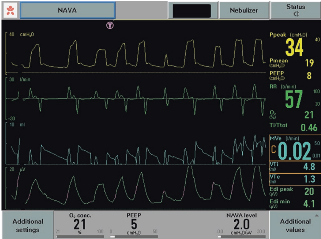
Fig. 50.11 Time tracings obtained during NAVA. From top to bottom : Airway pressure (yellow), flow (green), volume (blue), and electrical activity of the diaphragm (green)
