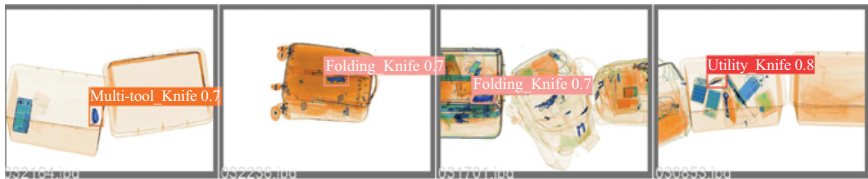
Figure 4.19 Results of DL tasks applied to X-ray baggage screening, the detection is performed with YOLOv5 on the GDXray dataset
