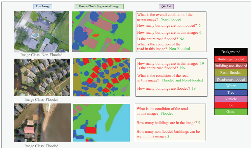
Figure 8.17 Three tasks (i.e. image classification, semantic segmentation and visual question answering (VQA)) included in the FloodNet dataset in [59]
