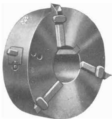
(a) Three roughing and one adjustable finishing tool
