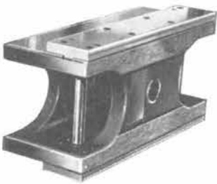
(a) Sine bar fixture for checking taper gauges
