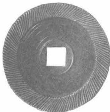
Fig. 129 A side and face cutter of 125 years ago
