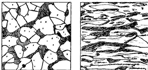
(a) Normal structure of a mild steel (0.17% C)
