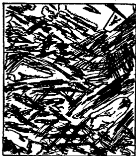
Fig. 29 Representing the needle-like structure of martensite in quenched carbon-steel. The white background is austenite \times 1000 approx
