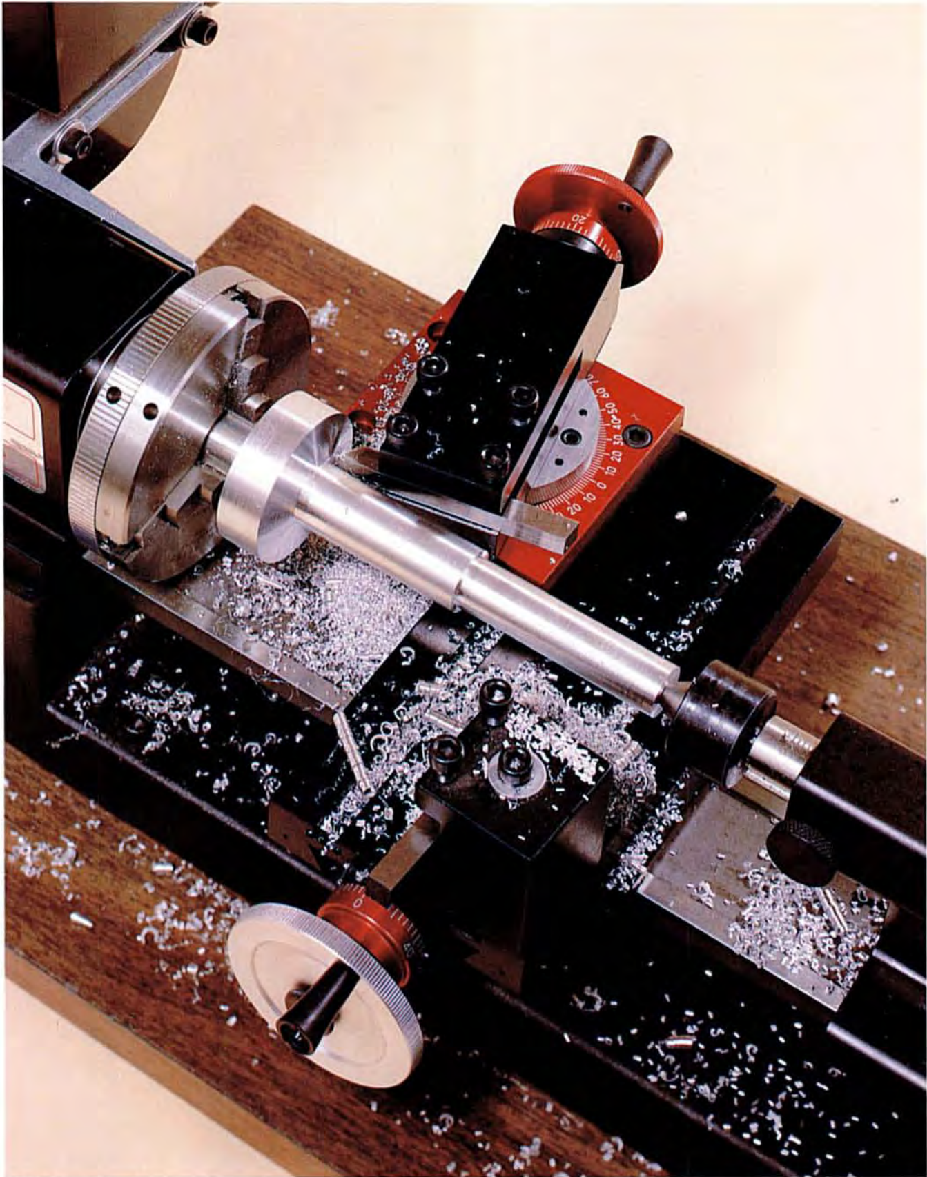
FIGURE 11—In this setup, the compound slide is suspended out from the table and a cut is being made close to the chuck. The length of the part would have made this taper difficult to cut using the usual method of offsetting the headstock.
