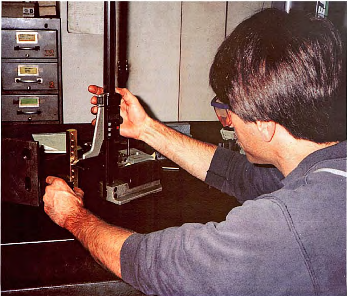
Measuring a part using a height gage on a surface plate.
