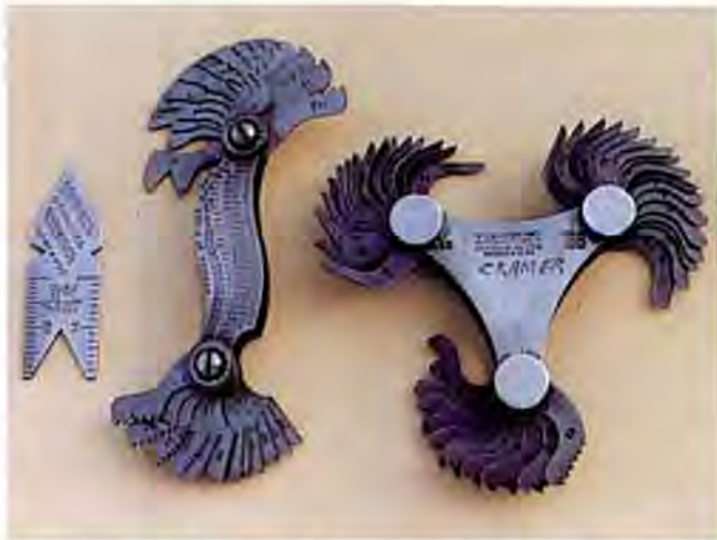
Two types of gages for measuring the number of threads per inch on an existing thread. The flat tool has a thread count scale as well as a 60° point and grooves for checking thread and tool shapes.
