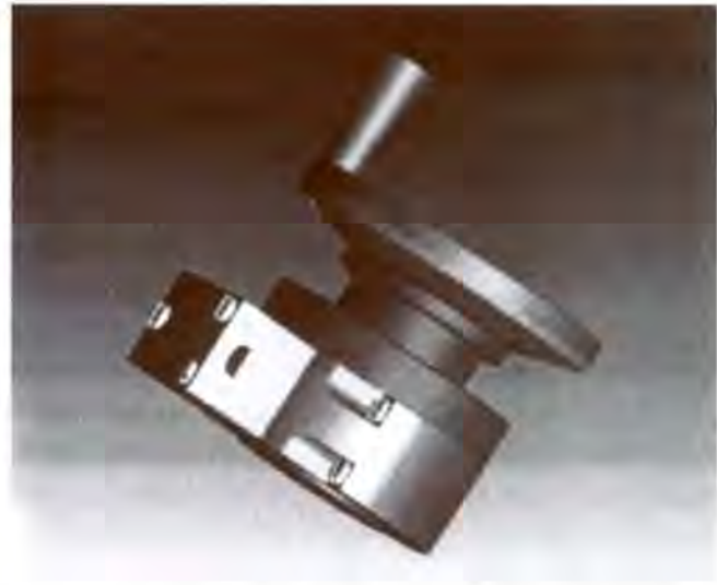
FIGURE 4—This 3-D drawing of a handwheel and sensor assembly is typical of what can be done in modern 3-D programs. This is a black and white laser print, but the drawing can be viewed in color on the screen and printed in color as well if you have a color printer.
