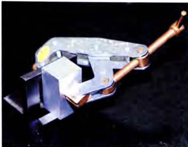
A part clamped to a right angle plate is held perpendicular to the table for milling.
