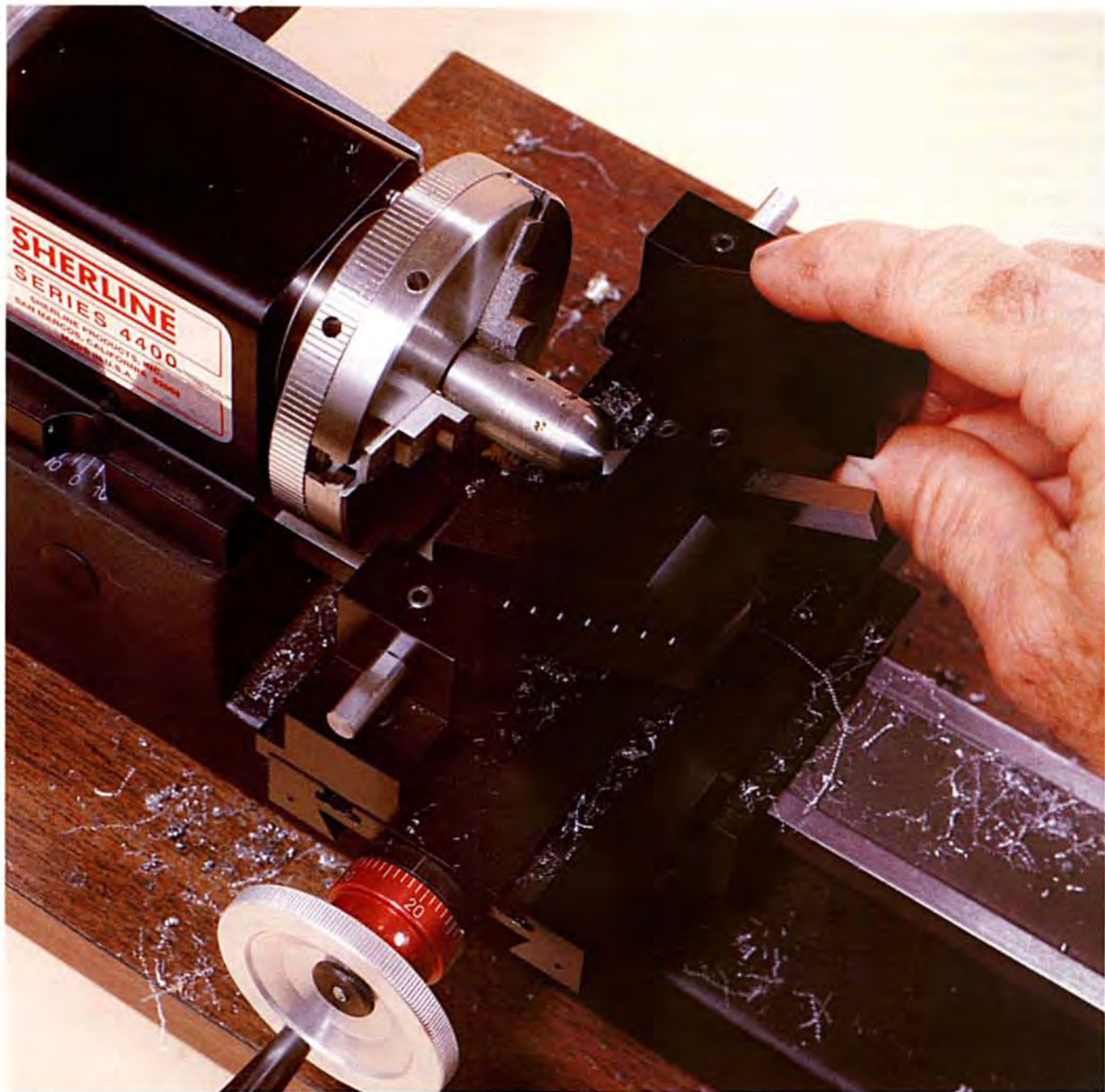
FIGURE 19—The radius cutting attachment required some original thinking. Once you realize that lathe tools don't necessarily have to move horizontally, coming up with a workable design was a lot easier.
