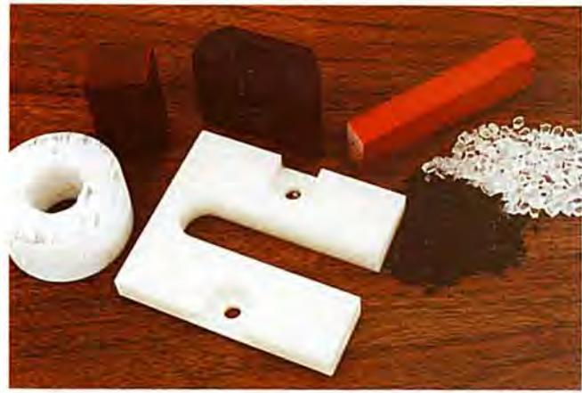
A selection of plastic raw materials. The dark brown block in the upper left is phenolic. Next to it is black Delrin. The red block is fiberglass. At the far left is a piece of white Delrin and next to it is a block of white Nylon. The two piles are new clear beads and recycled black chips used for injection molding.
