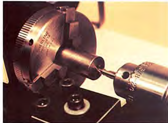
A center drill being used to find the center of a piece of stock. The 60° angle will locate the point of the tailstock center for turning between centers. The smaller hole will serve as a reservoir for lubricant if a live center is not to be used.
