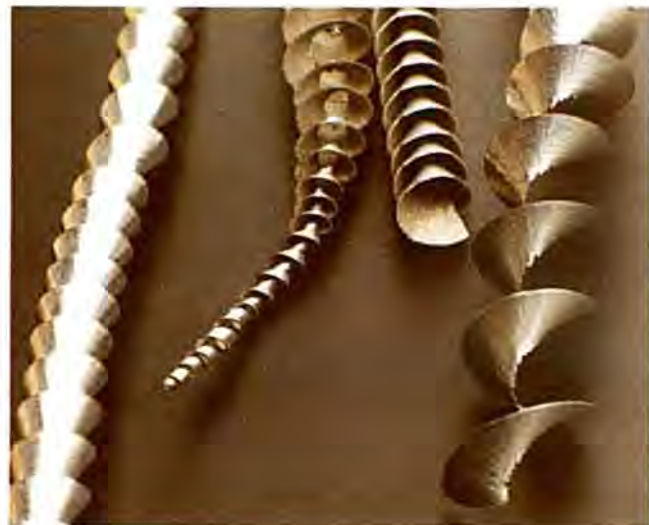
FIGURE 23 —If the metal is coming off like it is being peeled from a roll, the speed and feed settings are correct. If there is a screeching or chattering sound, you need to adjust speed and feed rates. Above are some aluminum chips that show the cutter was peeling a continuous strip of metal off the stock.
