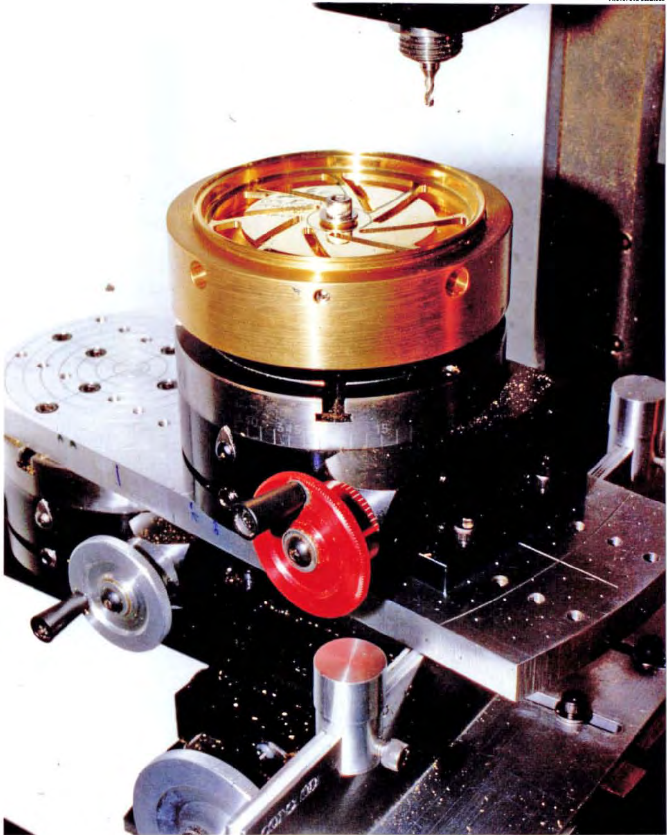
A custom made double rotary table setup by Bob Beslauer of Ft. Lauderdale, Florida allows for some very sophisticated rotary movements. Bob designed and machined the plate which mounts on one rotary table and then holds another rotary table. He used this setup in the mill to machine spiral spoke patterns on miniature custom automotive wheels.
