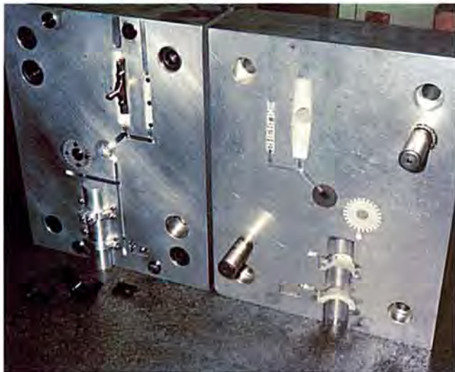
A plastic mold used to make a housing for the new digital readout for a Sherline mill. It can take a very expensive mold to produce what looks like a simple part. The longer the machine runs, however, the cheaper the parts become.
