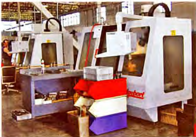
Designed for production jobs, these two Bridgeport TC3's are relatively compact but cost about $50,000 each and fit into the third category above.
