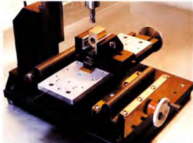
A tooling plate mounted to the mill table offers several ways to hold parts while also protecting the table from accidental damage. Here, a mill vise is used to hold a part. Notice Tim has custom-designed his own shield to keep chips off the leadscrew.
