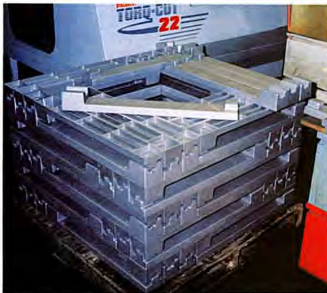
Die cast lathe bases as they come from the foundry and before they are machined. Proper draft angles and shrink rates must be considered in the design so that the parts will release from the mold and end up the right size.
