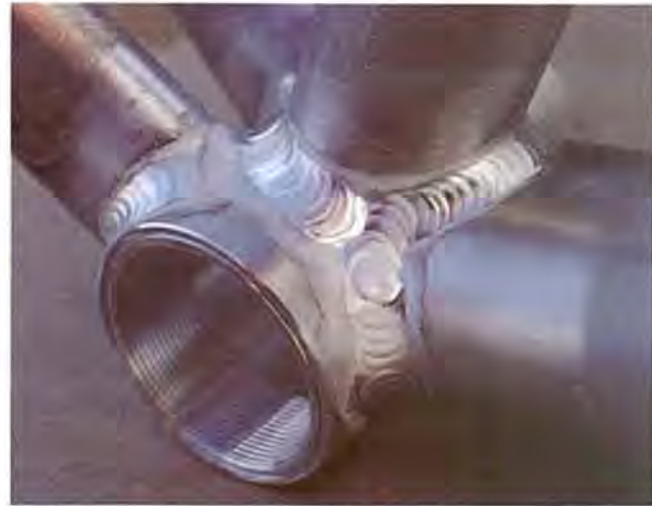
A close-up of an expert weld in aluminum shows a good, even bead with proper penetration. Like all skills, welding takes a lot of practice and a good knowledge of your tools and materials to get good results. Being able to do some basic welding is probably one of the more useful skills you can obtain. Though not often used in miniature machining, it can come in handy for many other construction and repair projects you will run across.
