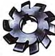
A typical involute gear cutter
