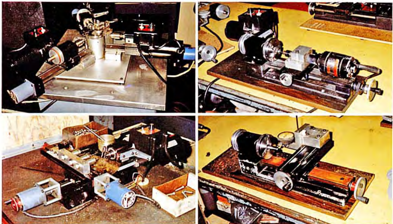
Sherline uses some of their own tools for small jobs in their production line. Shown here are a number of special tools used for making chucks and collets. Clockwise from top left: Drilling tommy bar holes, grinding inside of chuck jaws, checking chuck runout and a setup to center drill, drill, ream and face collets.
