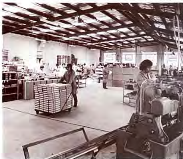
The Australian factory of Ron Sher Pty. Ltd. where the first Sherline machines were produced. Loose production tolerances of the early machines caused assembly to be a time consuming "mix and match" process.
