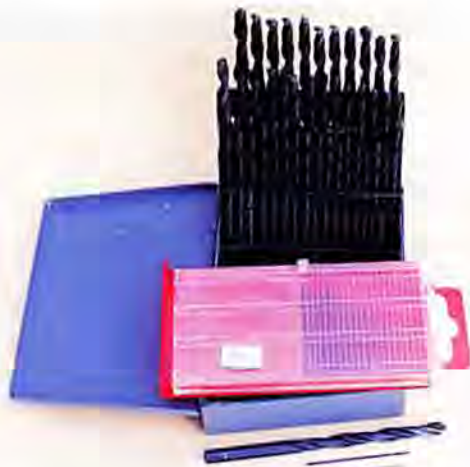
The metal box holds a set of drill bits sized from number 1 through 60. The red plastic box holds a selection of very small bits from number 61 through 80. In the foreground are #1, #60 and #80 sizes.
