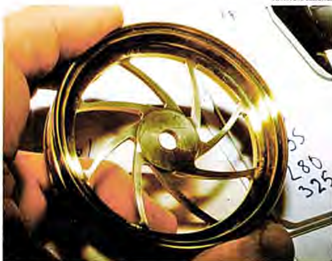
A beautiful eight spoke brass wheel made on Bob Breslauer's special double rotary table setup. A lot of careful thought went into this design.
