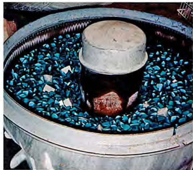
A commercial "tumbler" uses abrasive particles to remove rough edges from machined parts.
