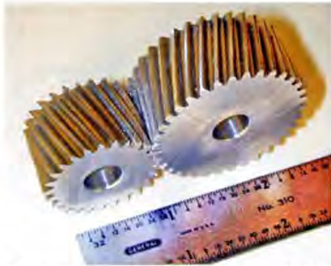
These small helical gears were cut using the X, Y and A axis on a CNC Sherline mill. The 25T and 34T gears were cut to full .089" depth in one pass.
