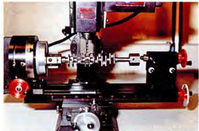
Here is a setup devised by Pete Weiss to machine the crankshaft for a running 1/6 scale Porsche air cooled engine he is building.
