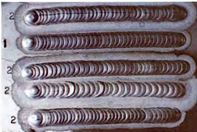
Some sample aluminum welds. Controlling the puddle of molten metal is the key to a good weld.
