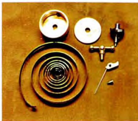
Mainspring, barrel, key and components of the winding mechanism.
