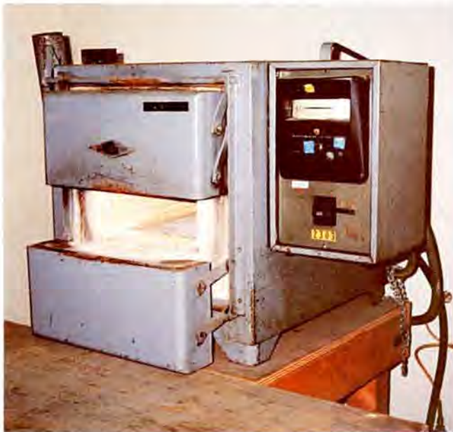
A heat treating oven heats items to be hardened almost to their melting points making temperature control critical.
