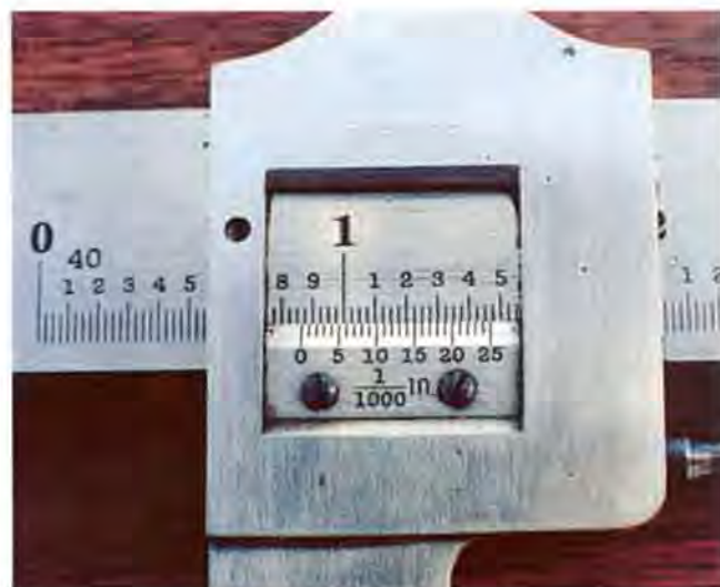
Vernier scales use a clever method to come up with a scale that reads to high levels of accuracy without requiring a division on the main scale for every increment. The reading on this scale is .867
