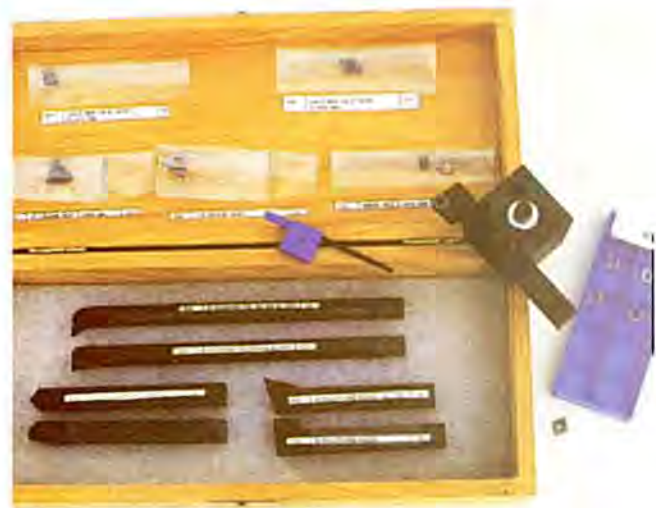
FIGURE 16—An inserted tip tool in its holder. The blue box contains additional replacement tips. In the wooden box are various tools and tips.
