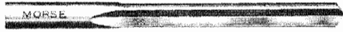
Figure 4-6 Straight-flute drill for free-machining brass, bronze, or other soft materials, particularly on screw machines. Also suitable for drilling thin sheet material, because of lack of tendency to “hog.” (Courtesy Morse Twist Drill and Machine Co.)
