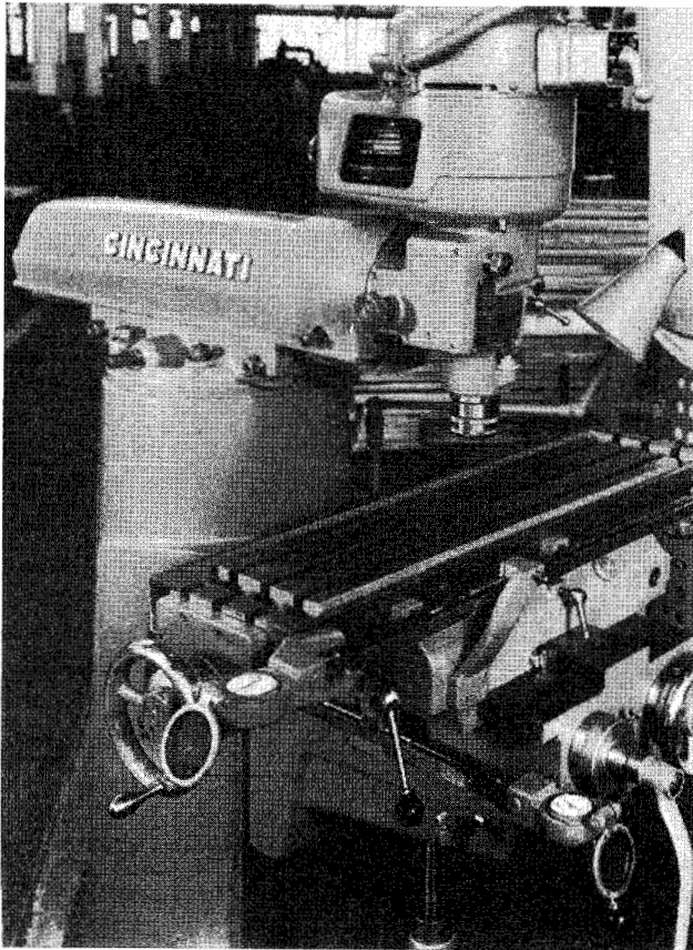
Figure 12-14 Milling a dovetail with the vertical milling attachment and swivel vise. (Courtesy Cincinnati Milacron Co.)
