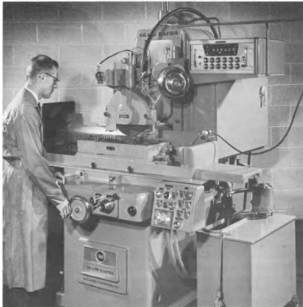
Fig. 13-2. Modern surface grinding machine equipped with digital readout of the wheel head.
