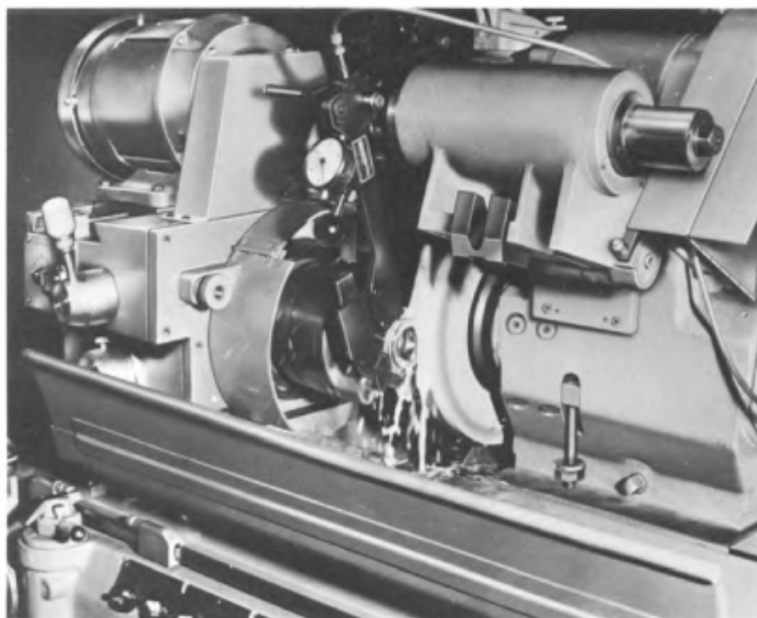
Fig. 12-20. A hand caliper gage for continuously measuring the diameter of the workpiece as it is being ground.
