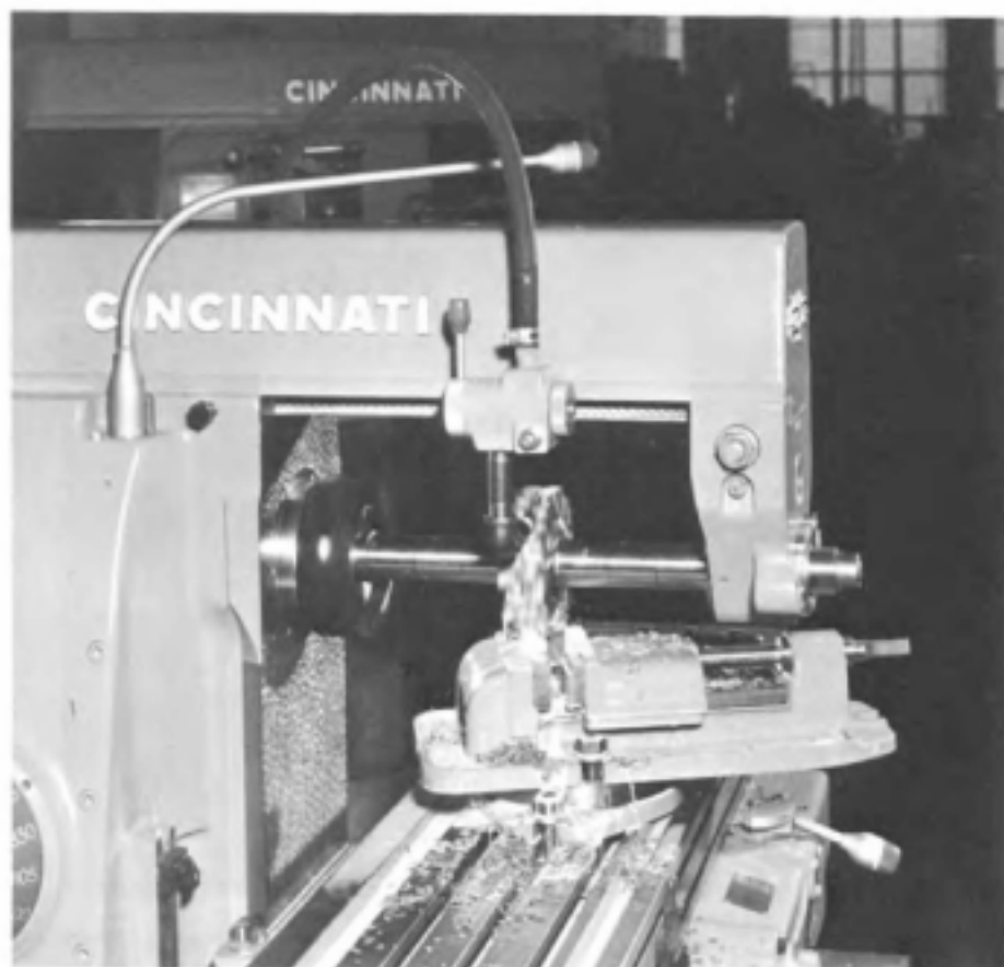
Fig. 6-25. Using a swivel vise for angular straddle milling.
