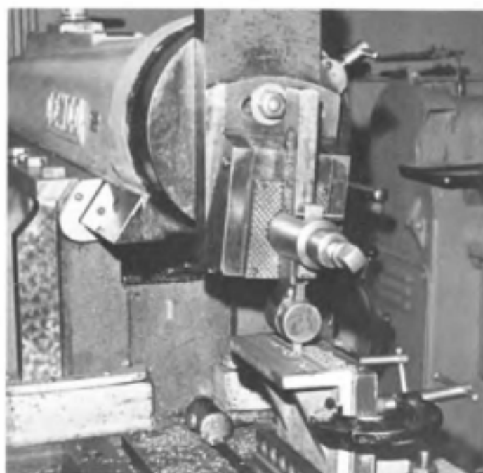
Fig. 2-17. Setup for finish-machining angle plate by clamping to another angle plate. Broad nose cast iron finishing tool used to finish surface of angle plate.
