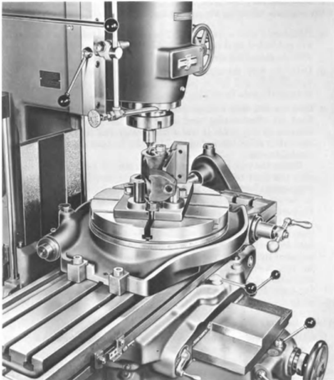
Fig. 6-36. End milling a circular slot in a part held by a milling machine fixture that is clamped on the circular table.
