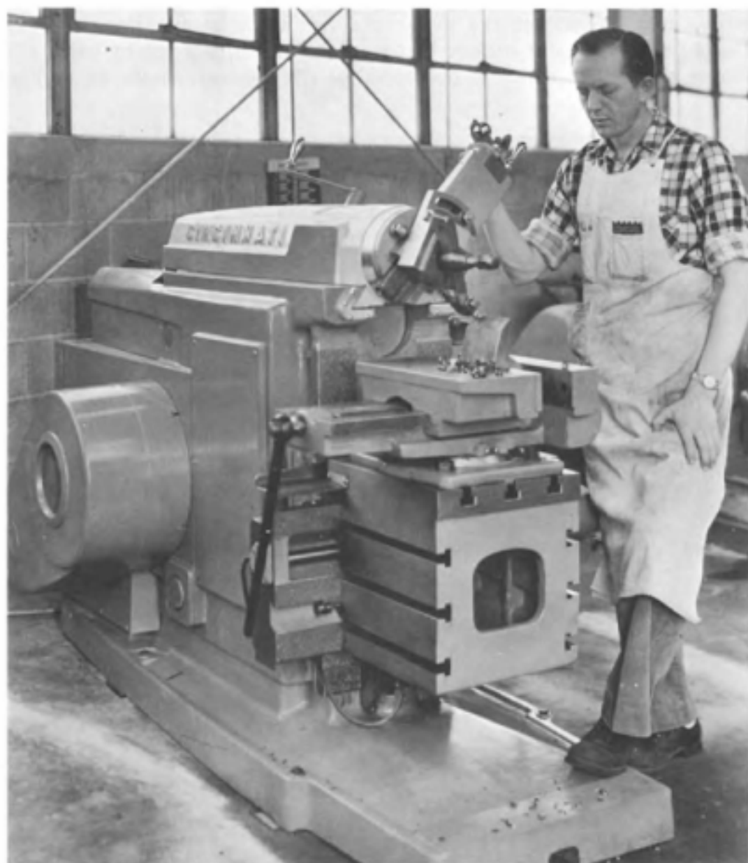
Fig. 2-20. Shaping an angular surface on a press brake forming die.
