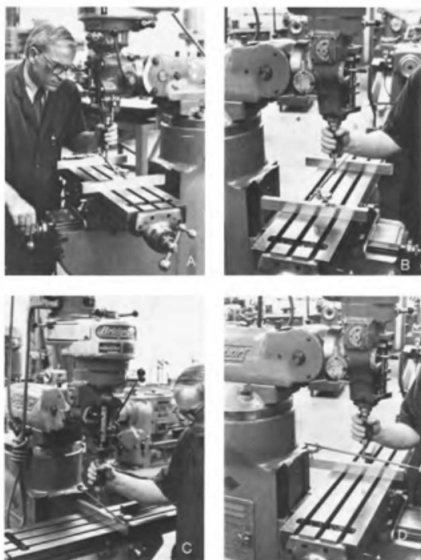
Fig. 6-29. Procedure for trammingspindle of toolroom milling machine.
