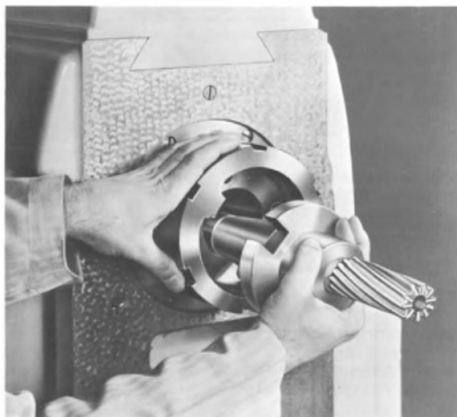
Fig. 4-20. The Cincinnati Arbor-Loc® spindle-nose arrangement for providing a rapid change of tooling.
