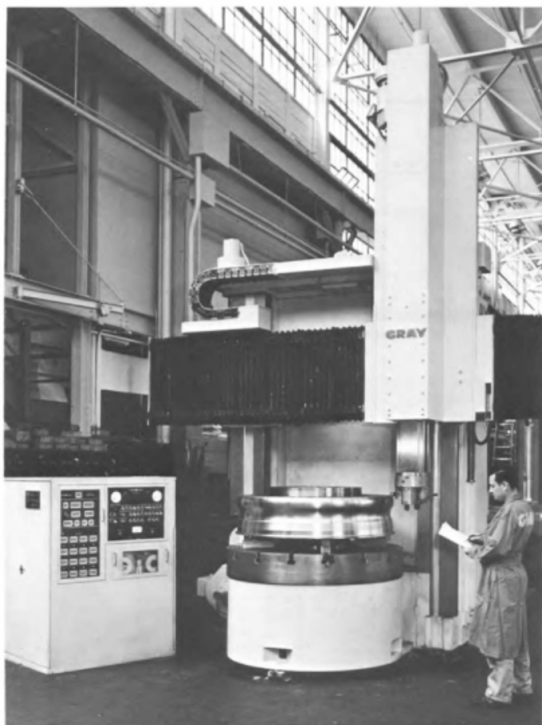
Fig. 15-22. Vertical boring machine equipped with a continuous path numerical control system.
