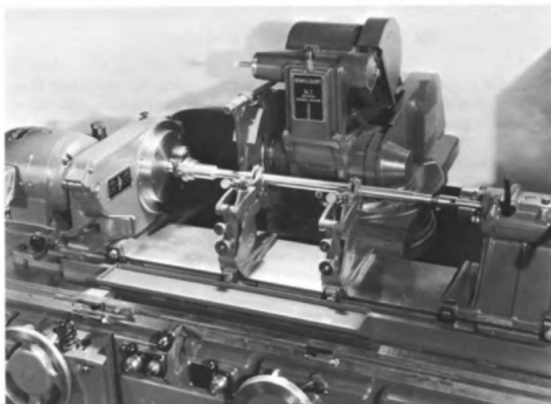
Fig. 12-5. Universal cylindrical grinding machine set up for traverse grinding.
