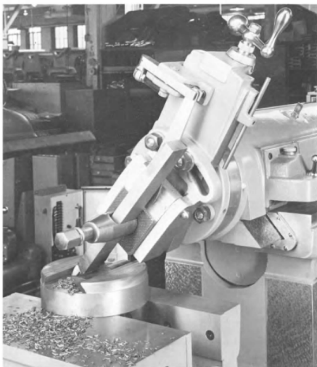
Fig. 2-21. Shaping a shaper head dovetail. Angular surface cut using feed of shaper head slide. Note correct setting of the clapper box.
