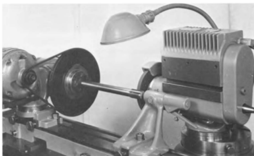
Fig. 14-30. Cylindrical grinding of a reamer on a cutter and tool grinding machine.
