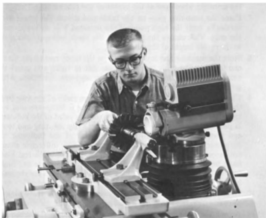
Fig. 14-15. Sharpening the peripheral teeth on a staggered-tooth side milling cutter.
