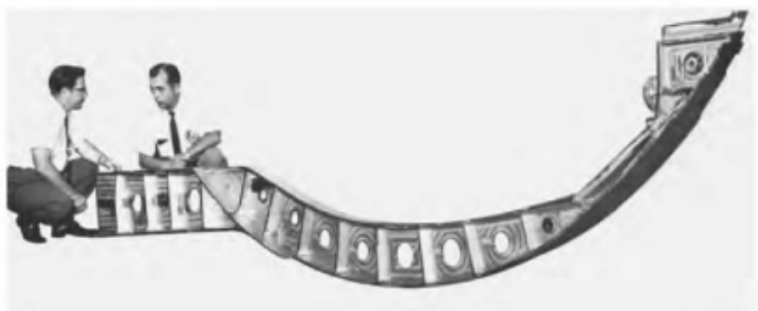
Fig. 15-4. Aircraft fuselage ring section produced on five axis profile milling machine in two setups—one for each side.
