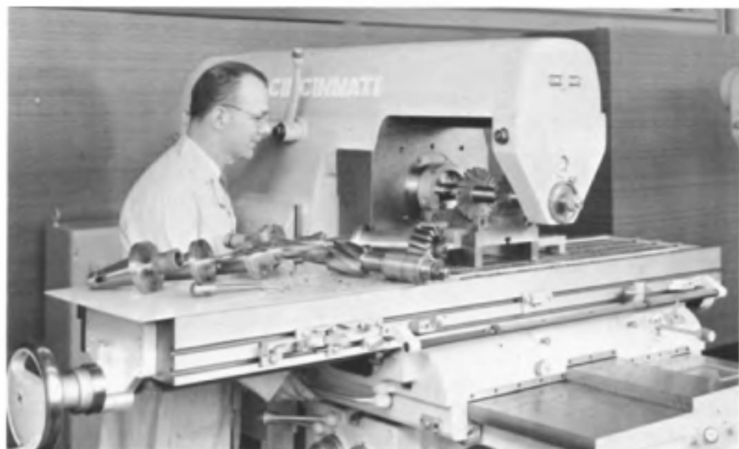
Fig. 6-1. Straddle milling the inside face of a casting. Tools for other milling operations are placed on a board to protect the milling machine and the cutting edges from damage.
