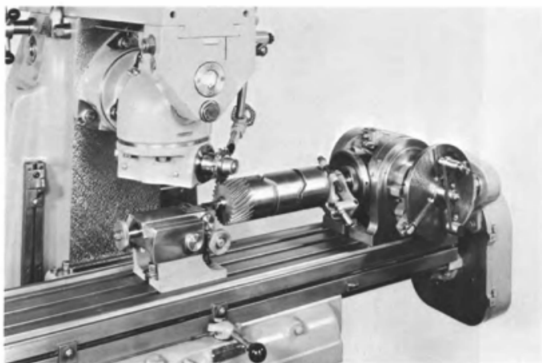
Fig. 9-18. Milling a helical gear on a plain knee and column milling machine using a universal milling attachment.
