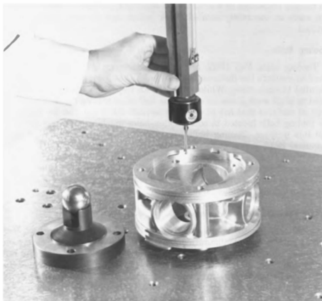
Fig. 16-24. Setup for measuring part on a coordinate measuring machine. Tooling ball is the reference point for measurements to the part surfaces.
