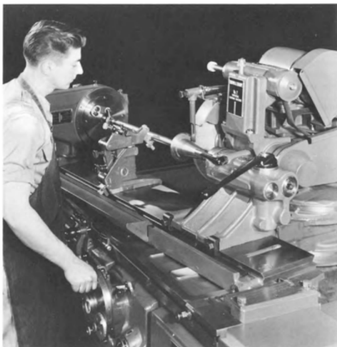
Fig. 12-9. Grinding a taper on a milling-machine arbor by offsetting the swivel table.
