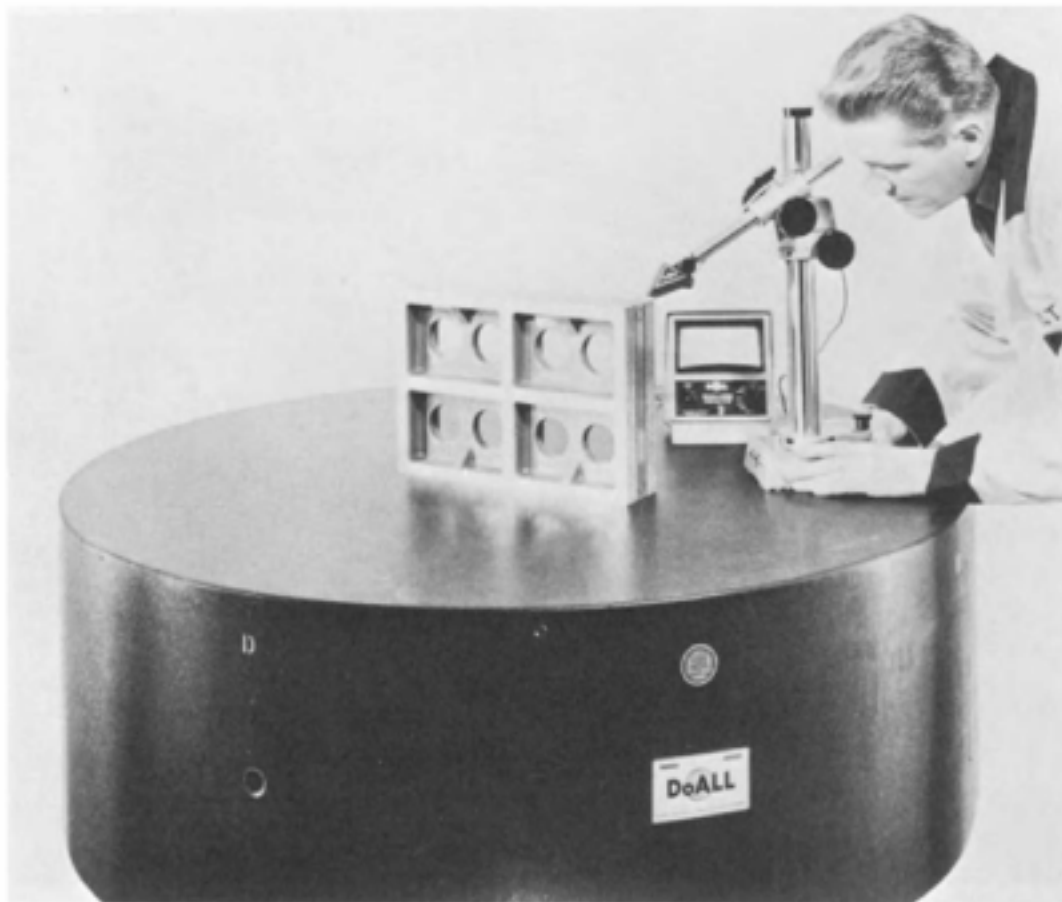
Fig. 16-4. Checking a master-grade box parallel for parallelism.
