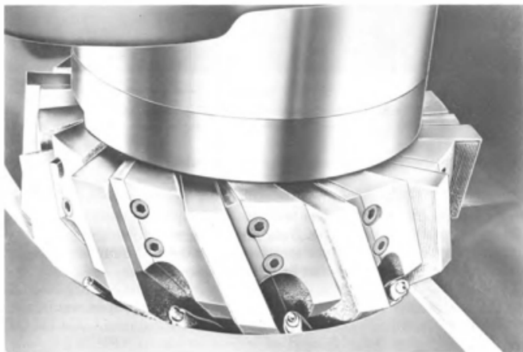
Fig. 5-24. High-speed steel, blade type, face milling cutter.
