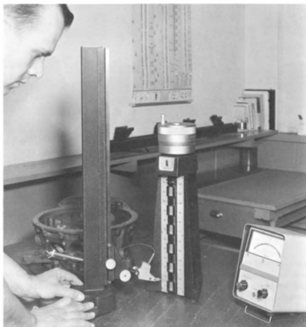
Fig. 16-10. Checking the height of a boss on a jet engine part with an electronic height gage and a micrometer height gage.
