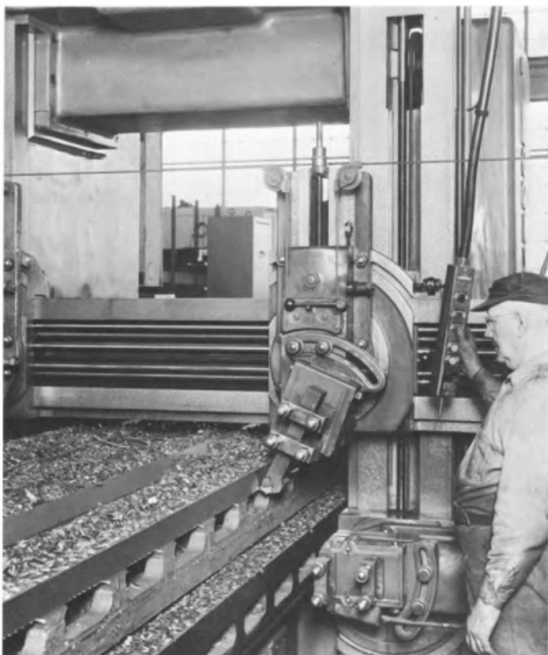
Fig. 3-13. Taking a vertical cut when planing the side of a planer table on a planer.
