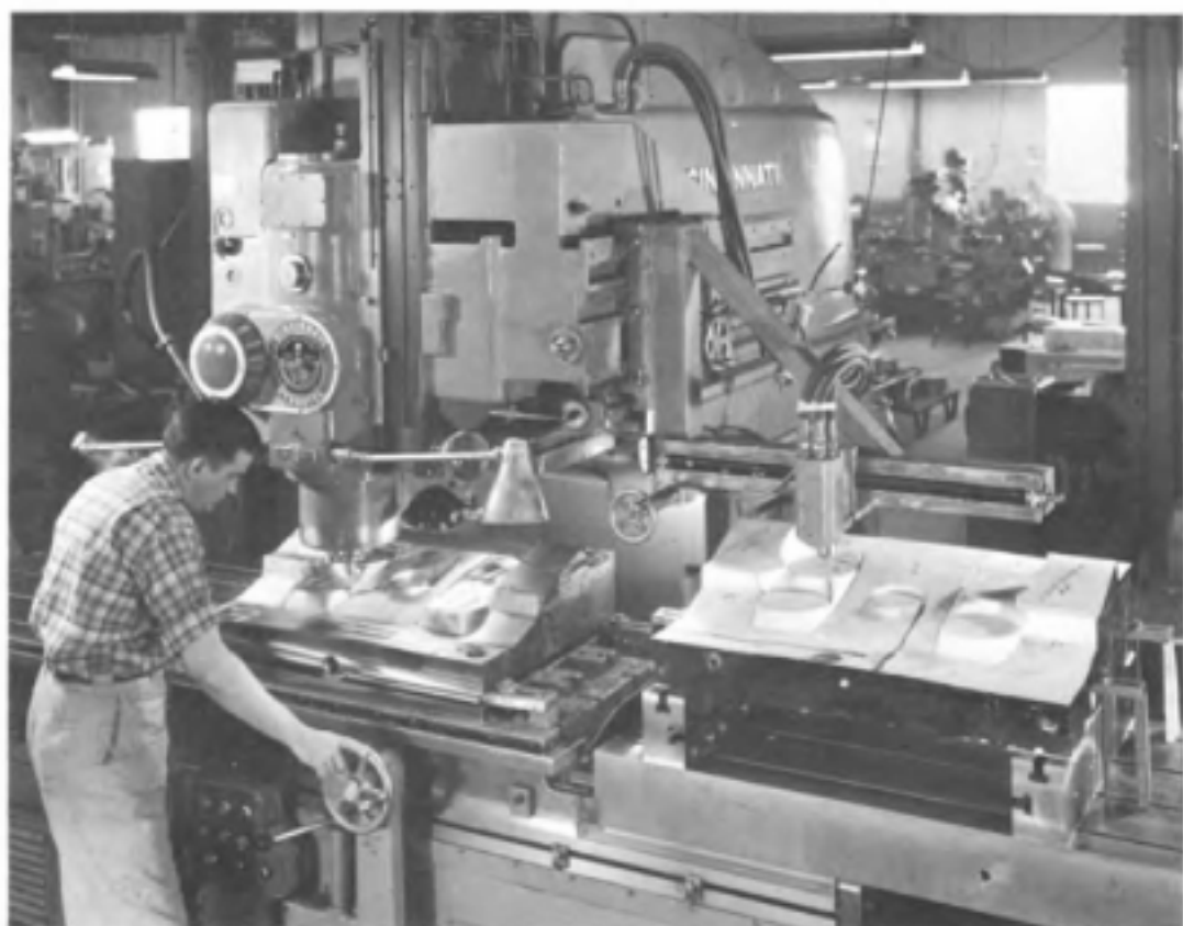
Fig. 4-14. Reproducing the contour of a plaster of Paris master onto a section of a drawing die.
