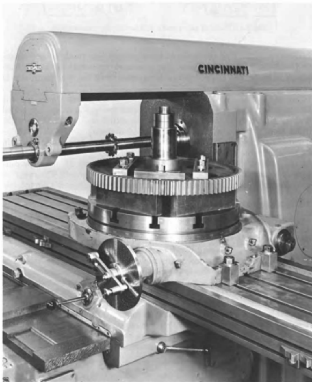
Fig. 8-6. Milling a large spur gear using a circular table equipped with an index plate.
