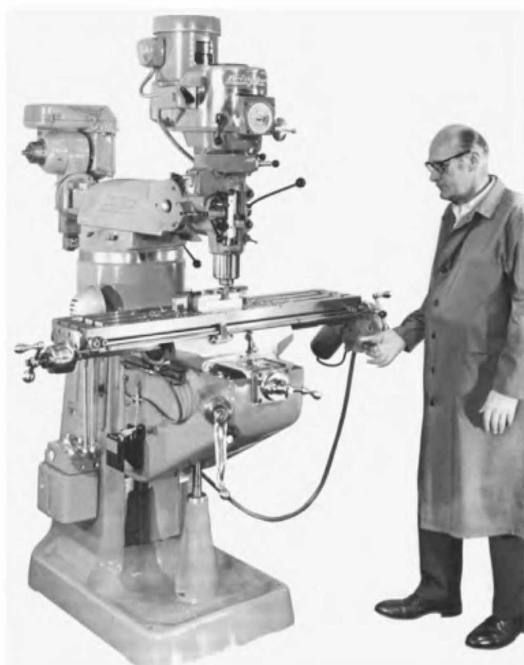
Fig. 4-10. Toolroom-type vertical milling machine equipped with a milling head and a vertical shaping head.
