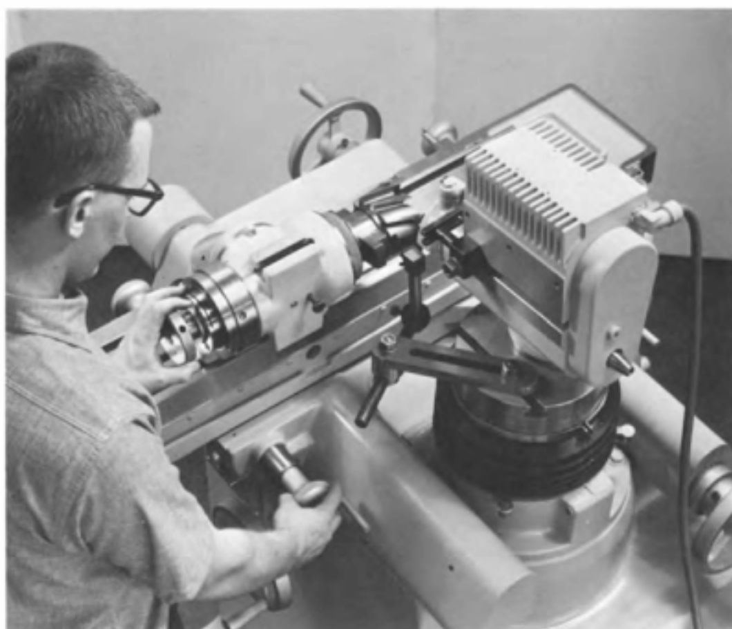
Fig. 14-13. Sharpening the peripheral teeth of a shell end mill.
