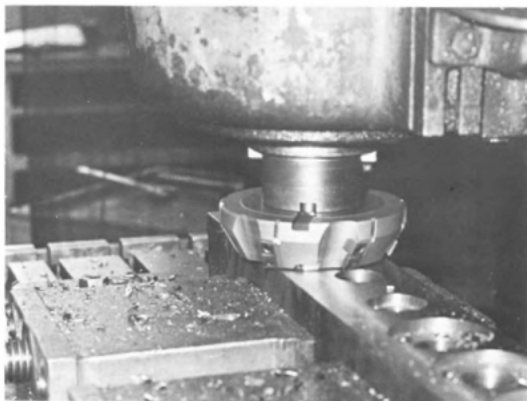
Fig. 6-17. Taking a finishing cut on a surface with a face milling cutter having finishing teeth on face to produce a smooth surface.
