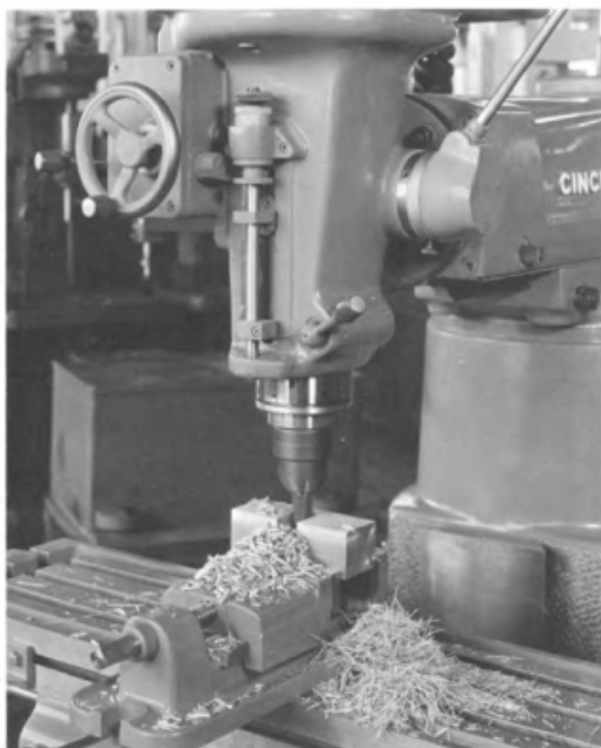
Fig. 6-20. Milling a slot with an end milling cutter.
