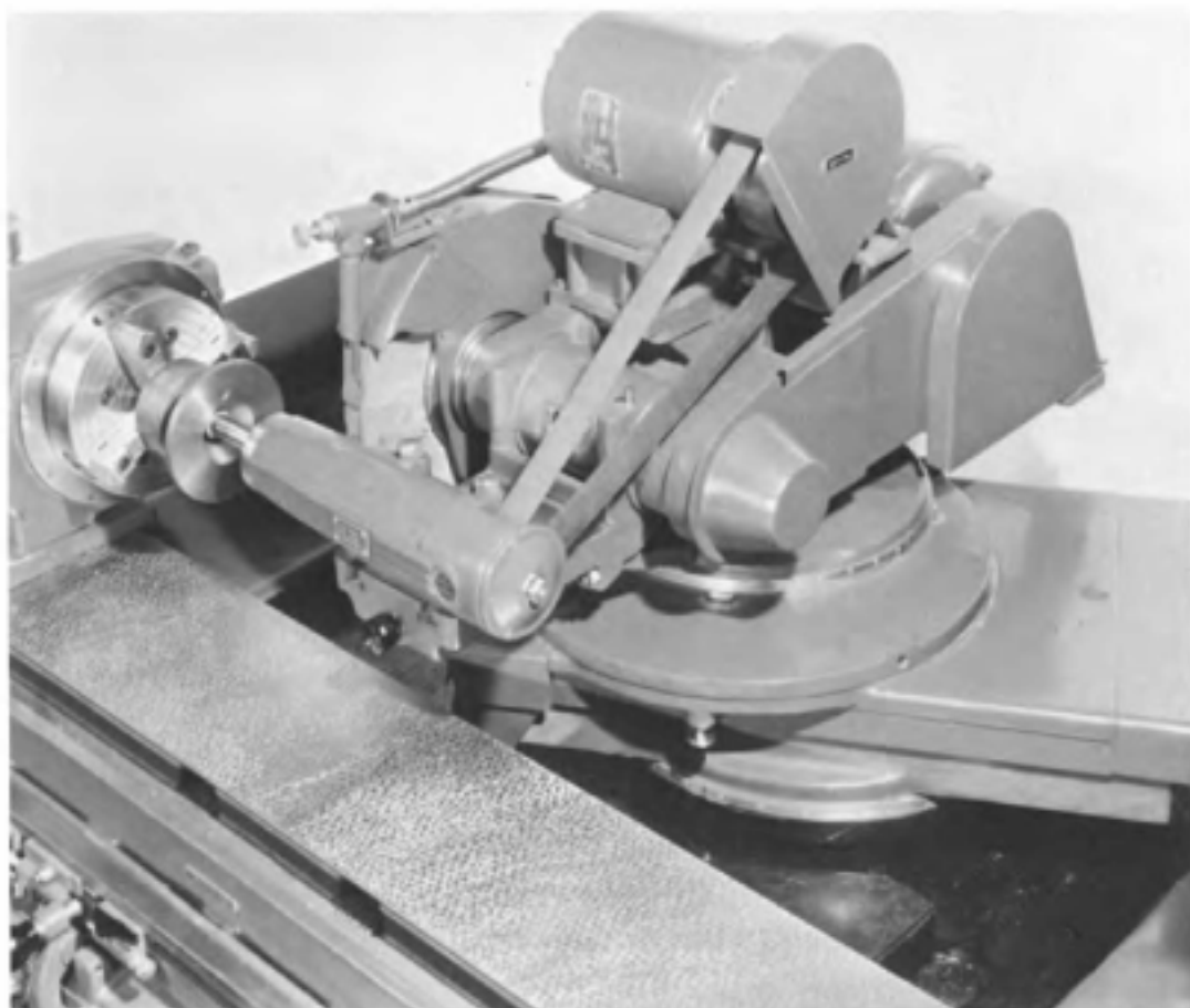
Fig. 12-17. Internal grinding a straight and tapered hole in one setup.
