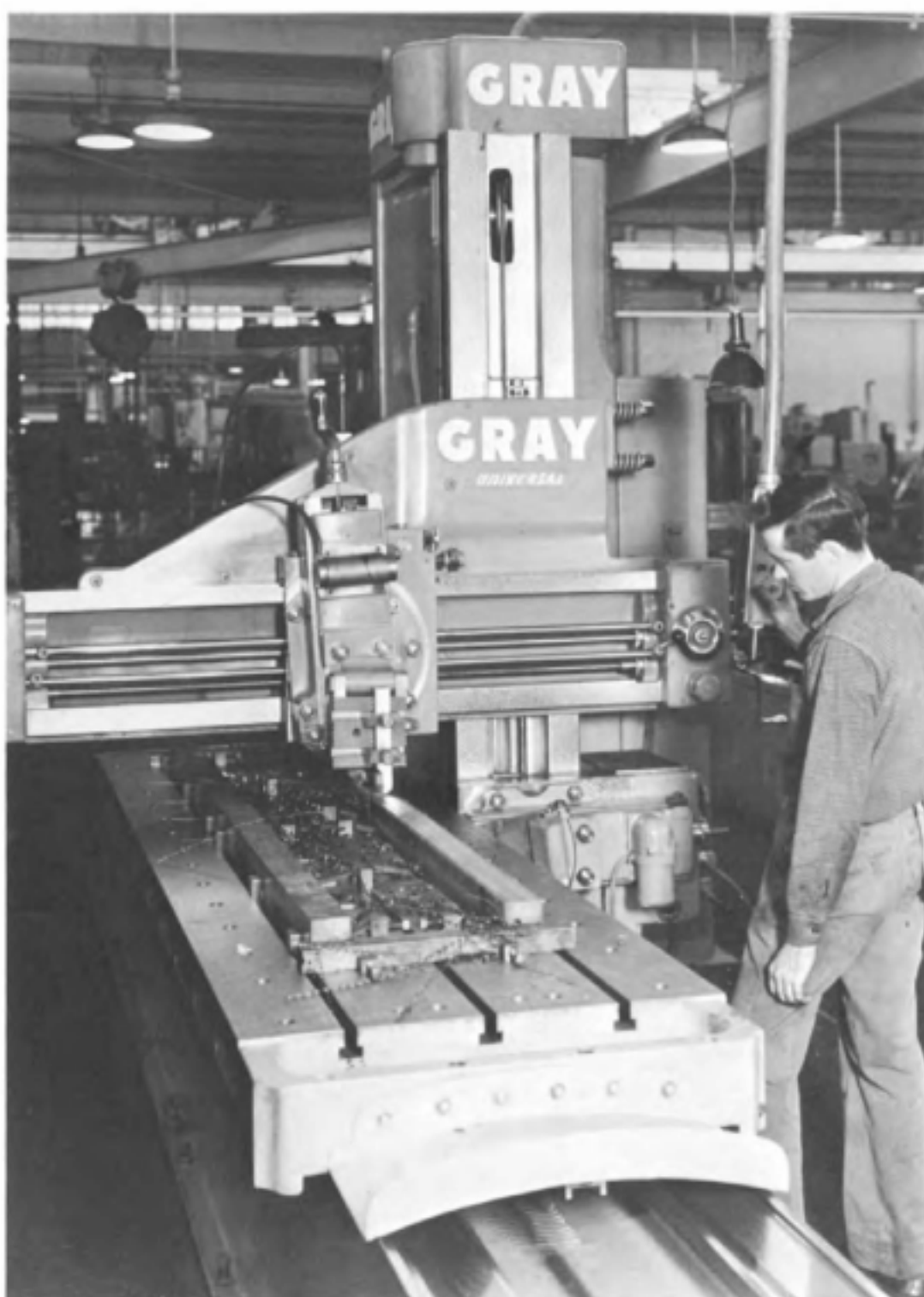
Fig. 3-17. Rough and finish planing steel bars simultaneously with a double cutting head.
