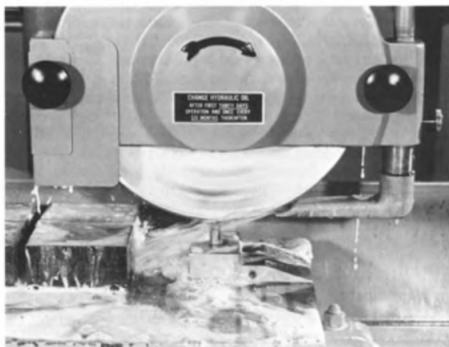
Fig. 11-12. Truing a Borazon ® grinding wheel on a surface grinder, using a steel bonded, diamond-impregnated tool. The traverse speed should be 3 to 5 fpm and the infeed .0005 in. per pass.
