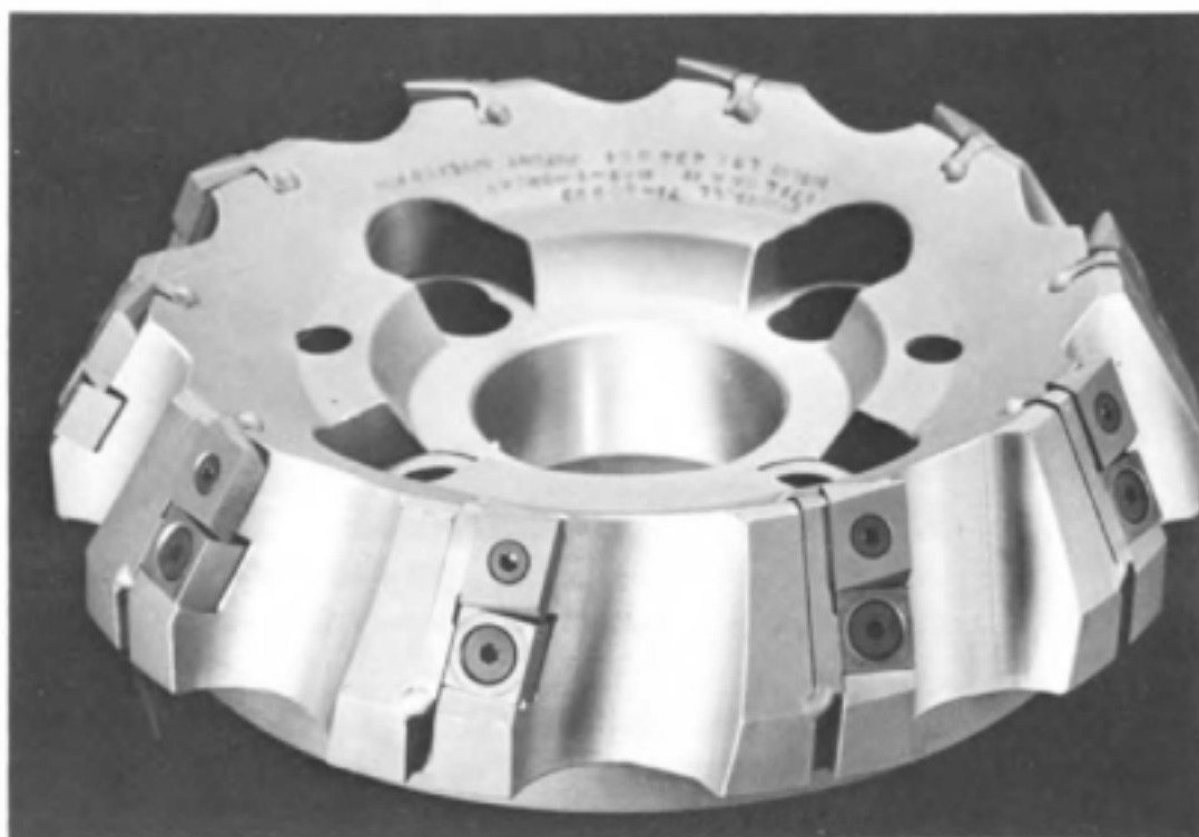
Fig. 5-18. Indexable insert cemented carbide face milling cutter.
