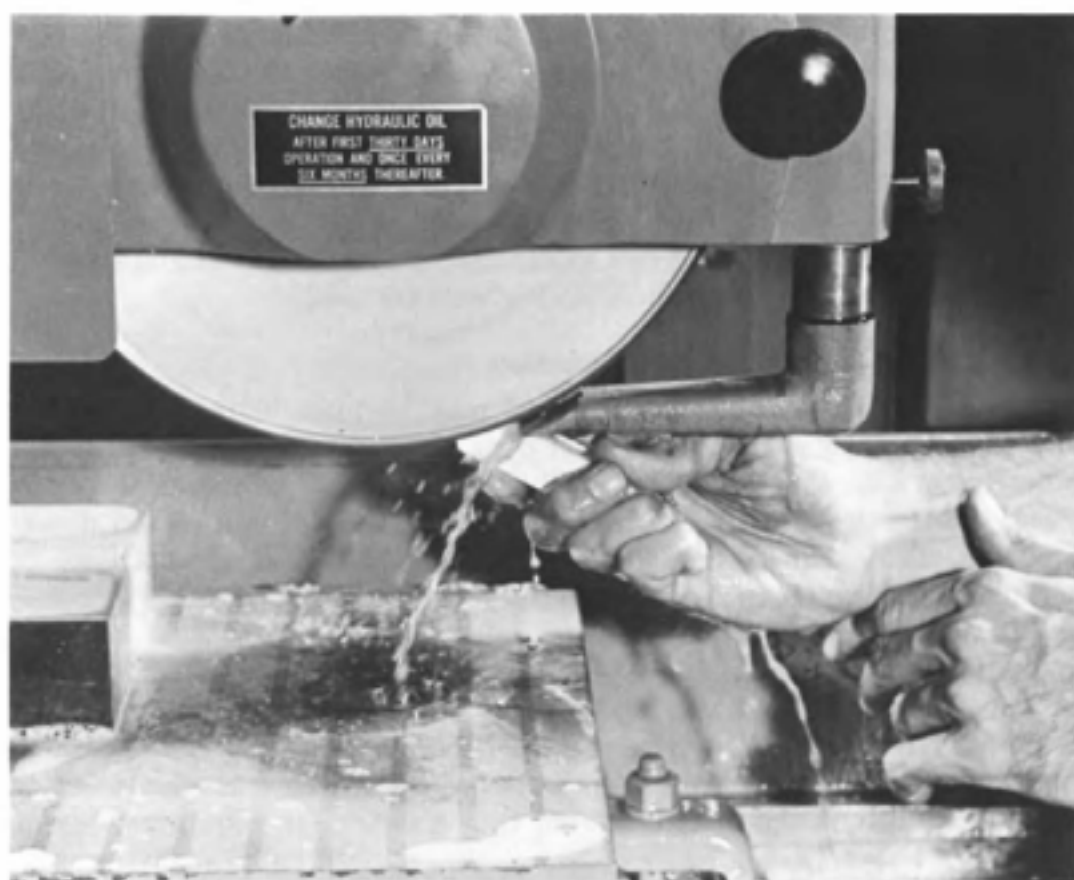
Fig. 11-13. Dressing a Borazon \text{B}_4\text{C} grinding wheel by hand, using a 220 grit, or finer (G hardness), aluminum oxide dressing stick.
