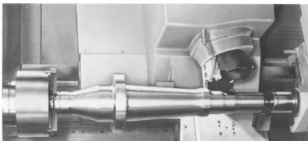
Fig. 15-27. Shaft type slant-bed NC turning center turning a shaft that is held on centers. A universal floating jaw chuck drives the workpiece without exerting a force on the headstock center.
