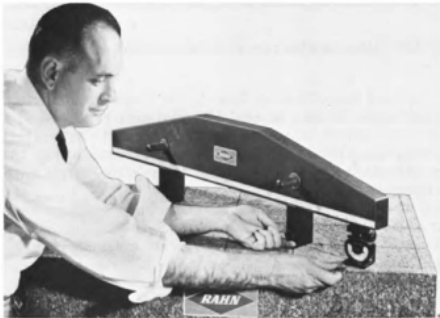
Fig. 16-2. Calibrating a surface plate with a Planekator ™ and a sensitive .000020 in. indicator.
