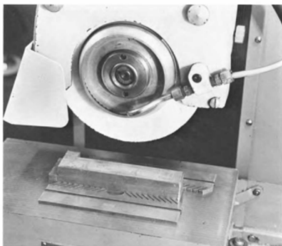
Fig. 13-16. Magna-Lock clamps used to hold thin part on a magnetic chuck.
