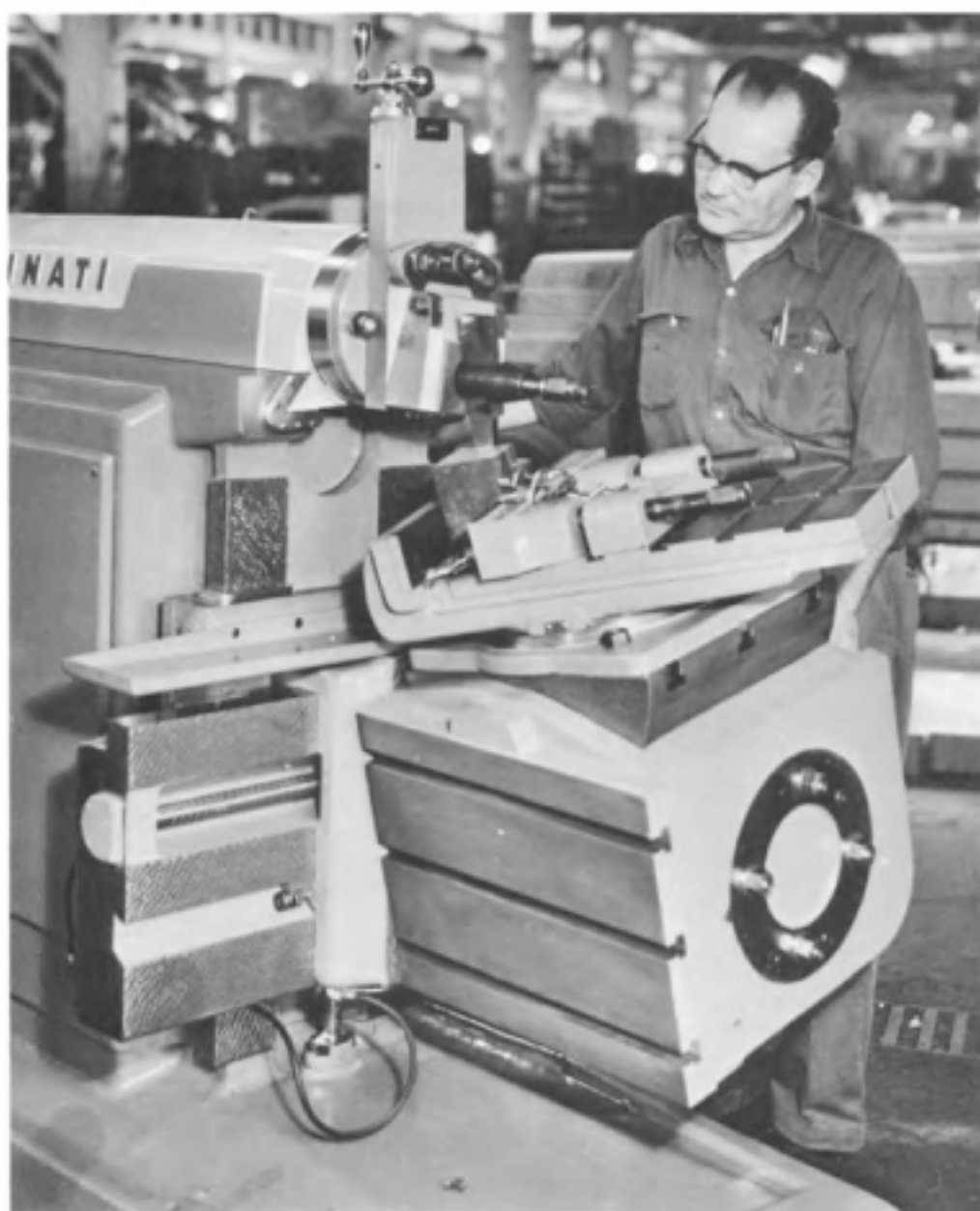
Fig. 2-22. Shaping a compound angle on a shaper equipped with a universal table.
