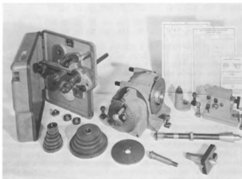
Fig. 7-3. The Brown & Sharpe Universal Spiral Index Head.
