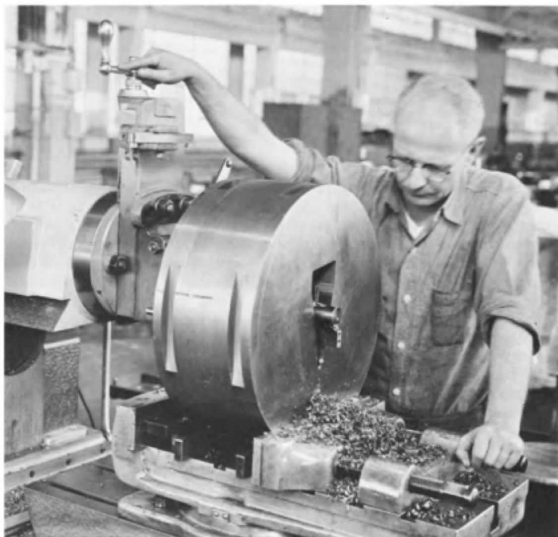
Fig. 2-23. Internal shaping of a large extrusion die using a shaper bar to hold the cutting tool.
