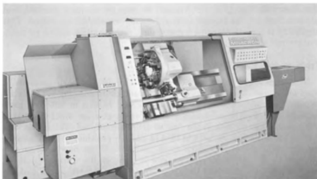
Fig. 15-2. CNC slant-bed universal turning center for chucking and for turning on centers. In order to show tooling turrets, protective window shields have been removed. Slant bed design allows chips to fall into chip conveyor for removal.
