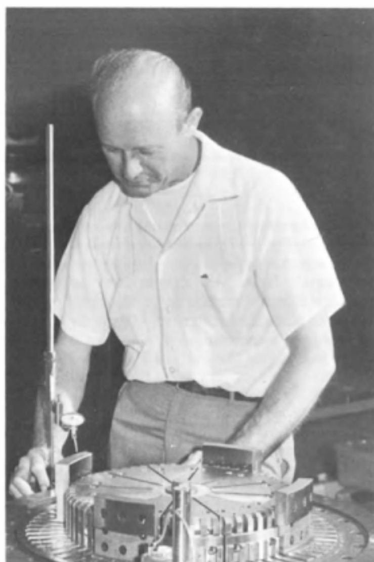
Fig. 16-7. Measuring the height of a pad attached to the disc using a vernier height gage.
