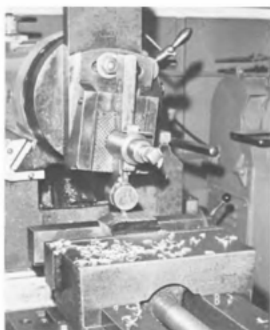
Fig. 2-18. A. Aligning workpiece with a surface gage in angular position in vise. B. Shaping the angular surface to the layout line.
