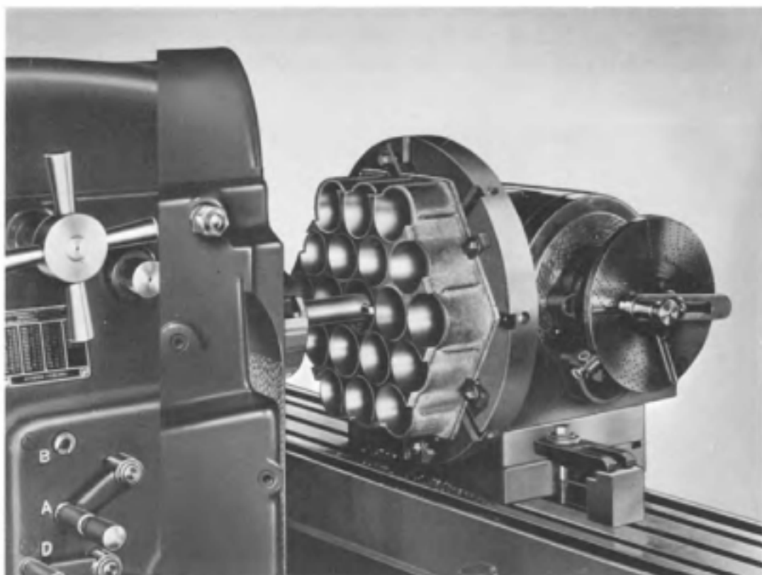
Fig. 8-24. Boring 19 holes in a cast iron plate.
