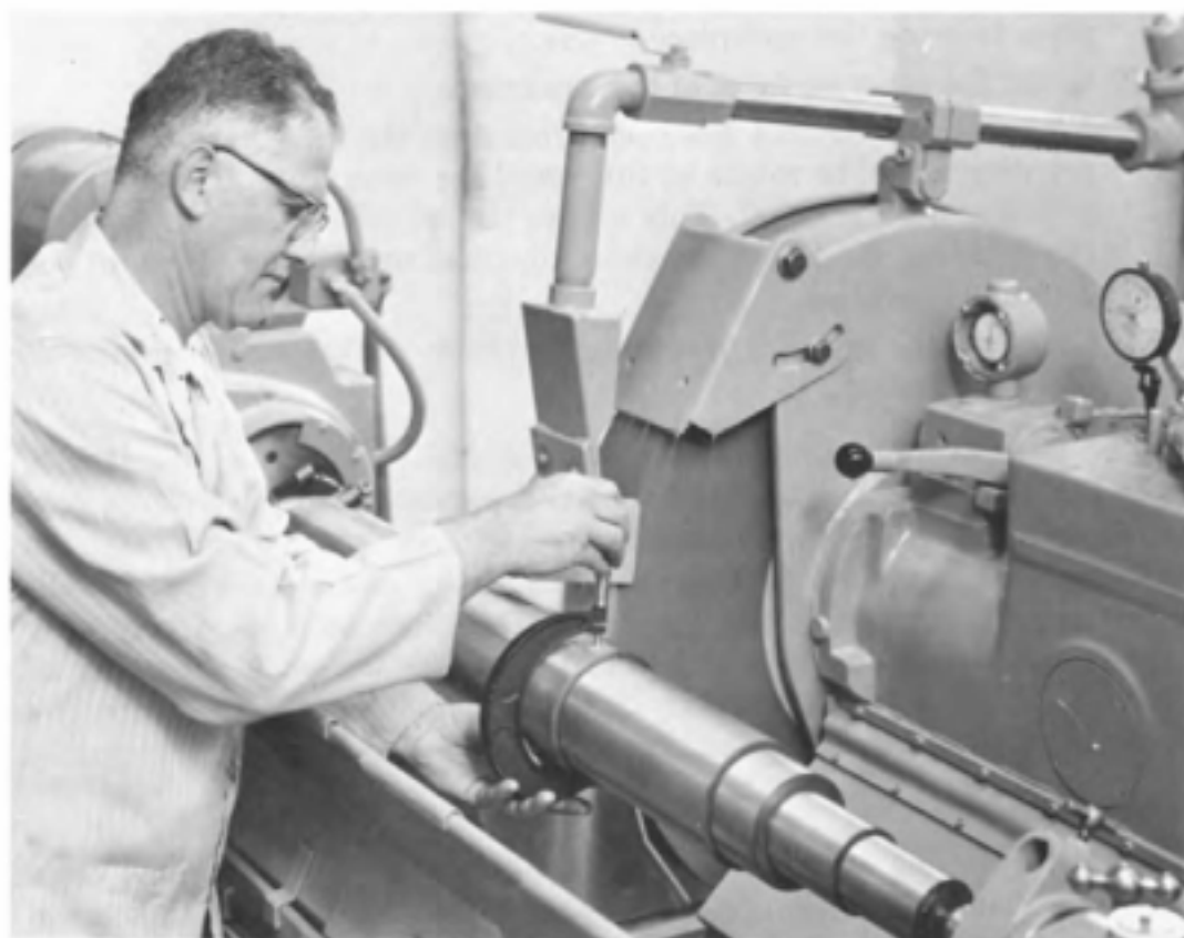
Fig. 12-6. Measuring the diameter of a surface on a plain cylindrical grinding machine.
