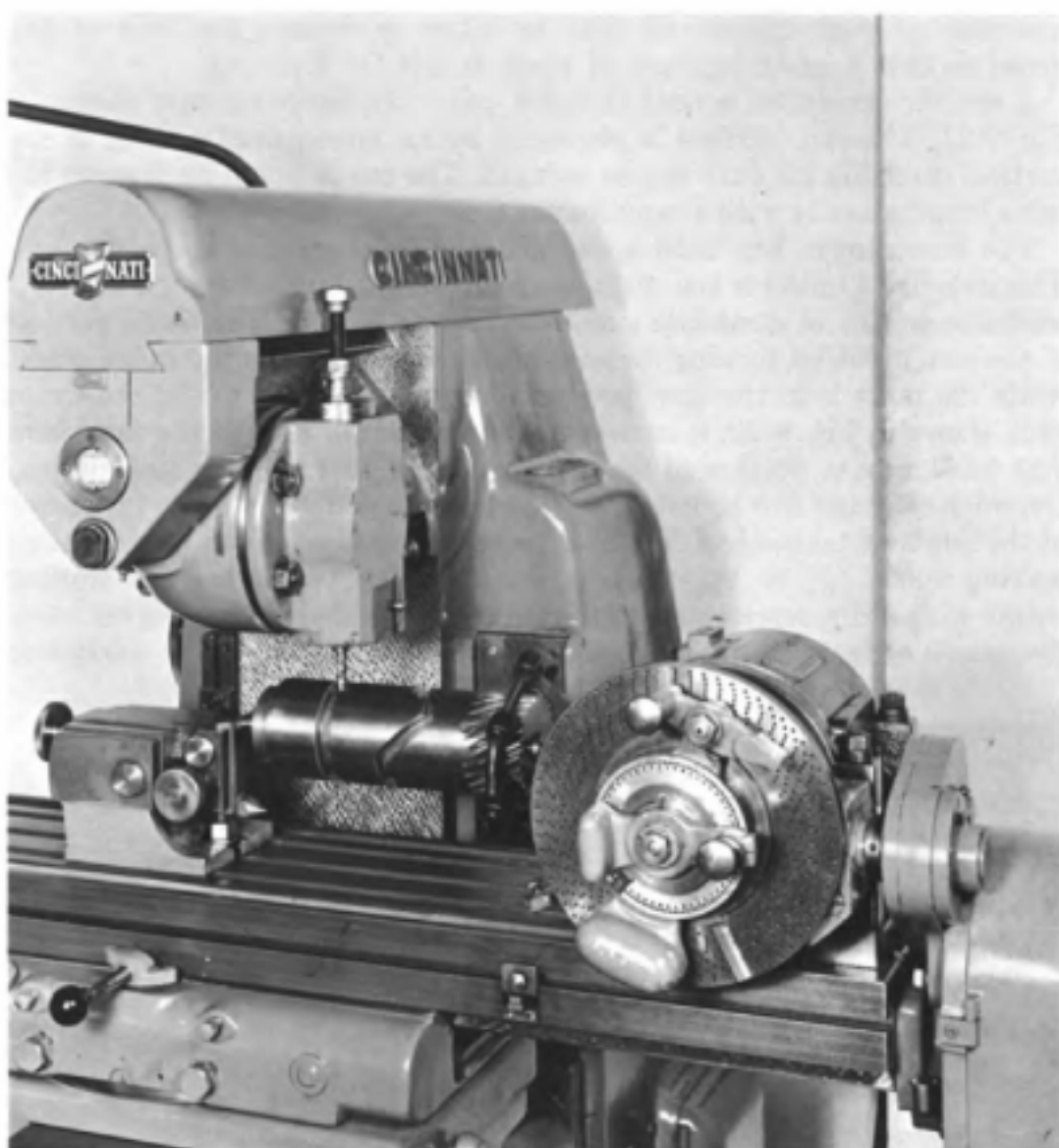
Fig. 9-29. Setup for milling a drum cam.
