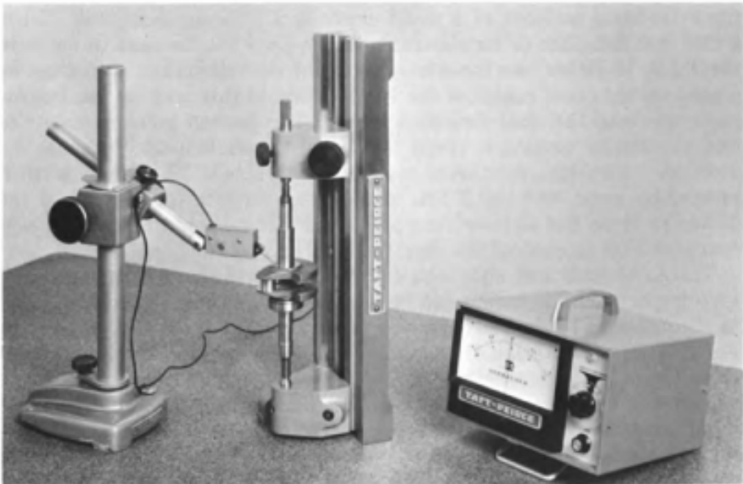
Fig. 16-14. Measuring the concentricity of a small crankshaft on precision bench center.
