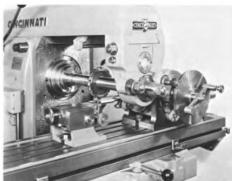
Fig. 8-11. Milling flutes in a tap using a form milling cutter.
