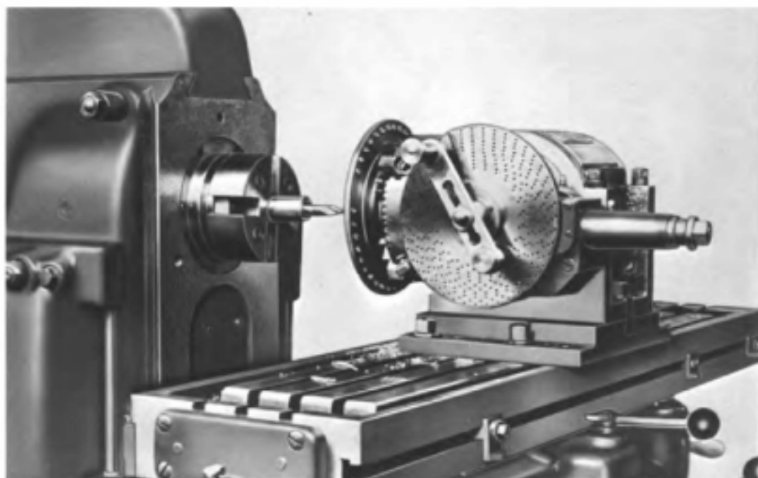
Fig. 8-25. Drilling holes around a hole circle in a flanged cap.
