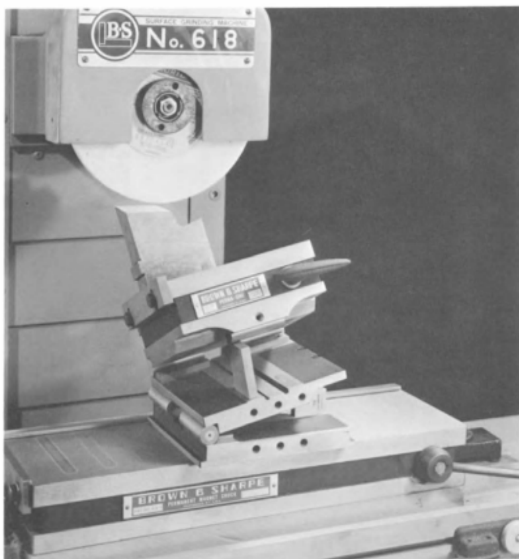
Fig. 13-14. Compound sine plate with permanent magnet chuck on work-holding surface.
