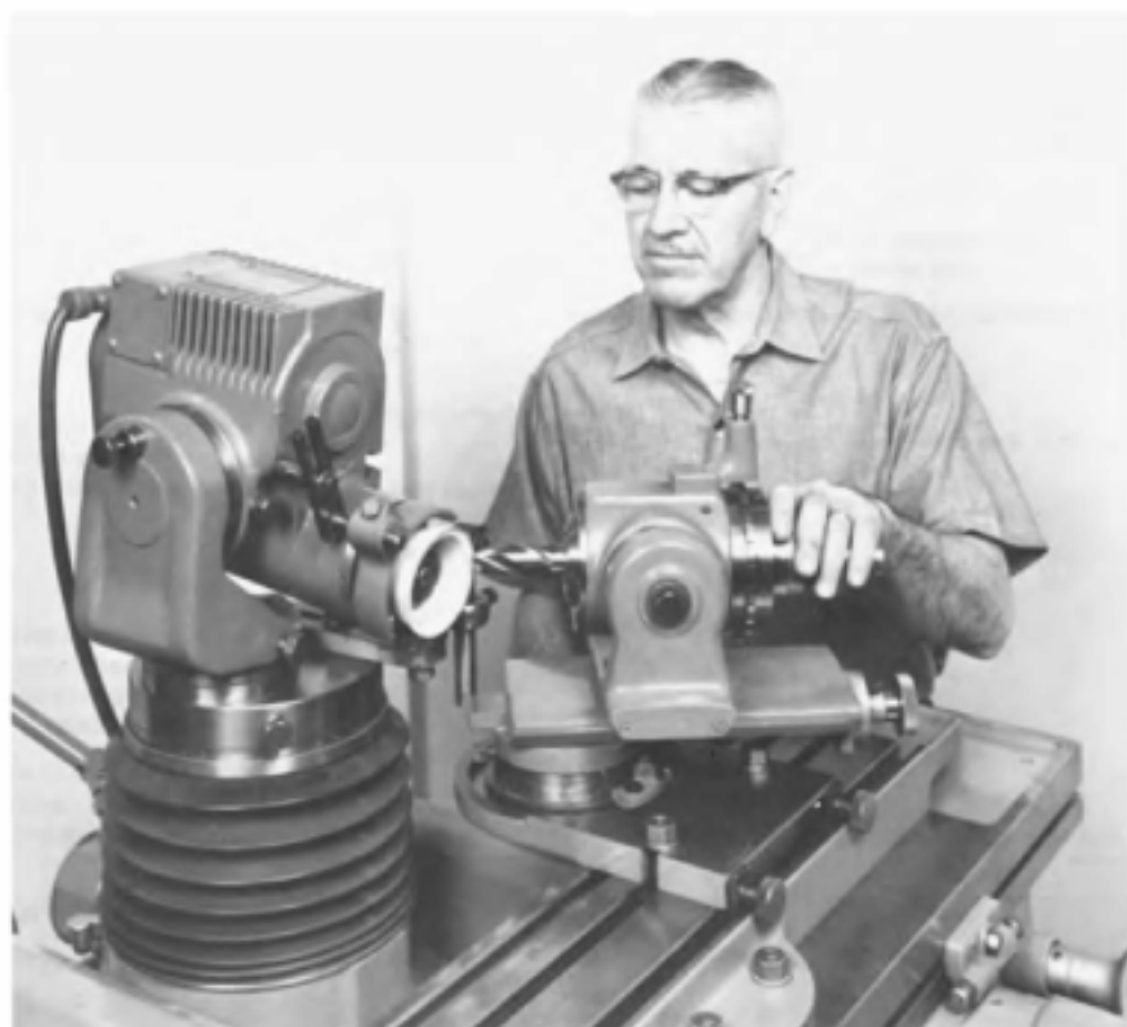
Fig. 14-28. Radius grinding attachment set up to grind the end teeth on a ball-nose end mill. Also used to grind other radii on milling cutters.
