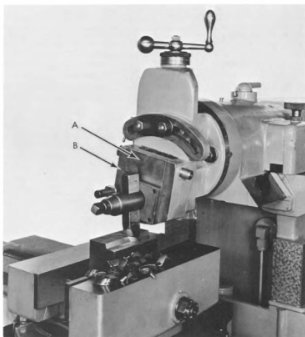
Fig. 1-7. A shaper taking a cut showing the shaper head and the clapper box (B) tilted. Clapper block is shown at A.
