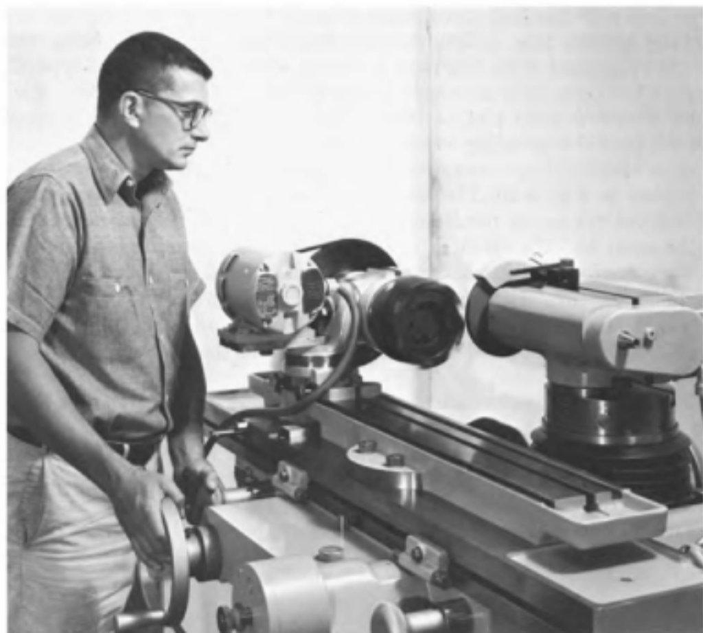
Fig. 14-18. Spin or circle grinding a face milling cutter.
