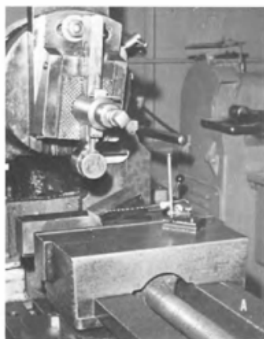
Fig. 2-18. A. Aligning workpiece with a surface gage in angular position in vise. B. Shaping the angular surface to the layout line.
