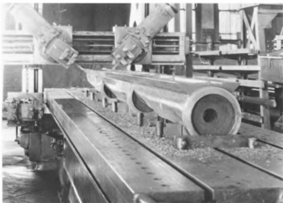
Fig. 3-19. Two angular cuts taken simultaneously by the cross rail heads on three castings "strung up" in tandem fashion.
