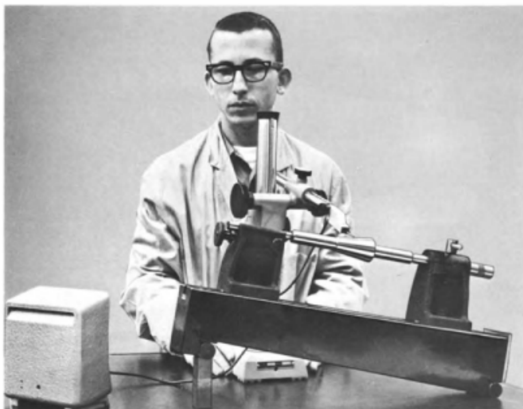
Fig. 16-21. Measuring the angle of a taper using a master grade granite 20-inch sine bar with metal T-slot containing a set of matched bench centers.
