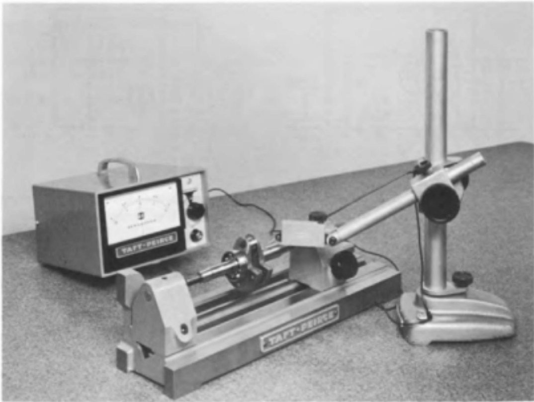
Fig. 16-14. Measuring the concentricity of a small crankshaft on precision bench center.
