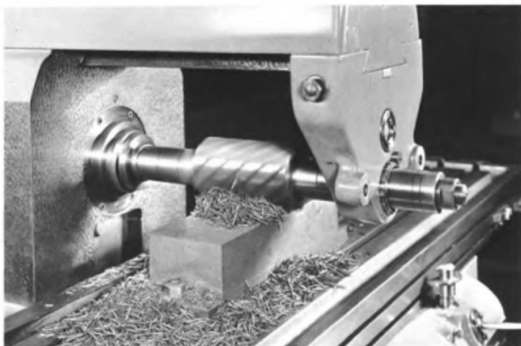
Fig. 6-9. Slab milling with workpiece clamped directly to the milling-machine table.
