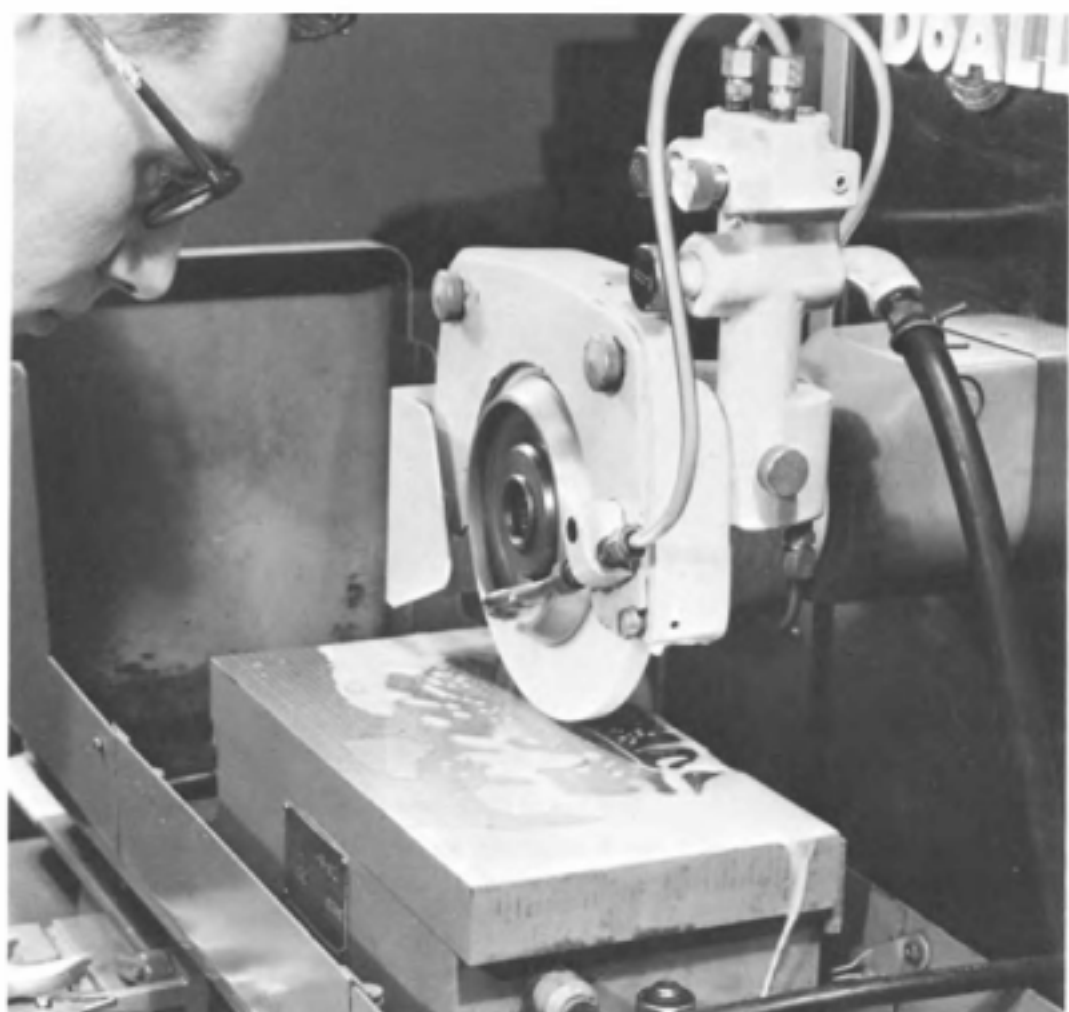
Fig. 13-6. Grinding the top surface of a magnetic chuck true.
