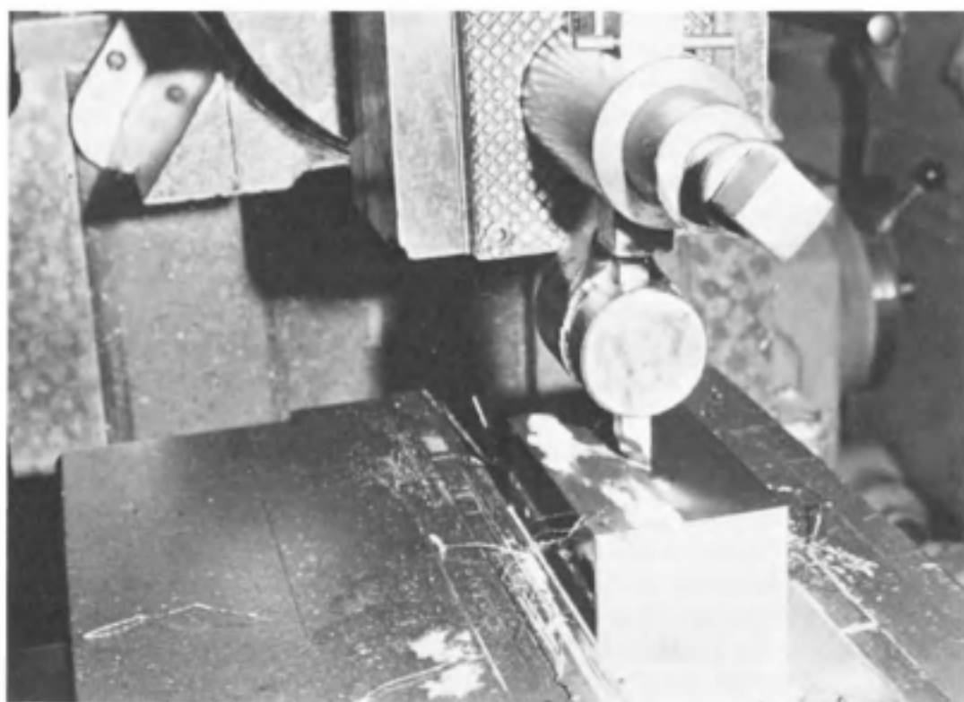
Fig. 1-13. Steel finishing tool in operation.
