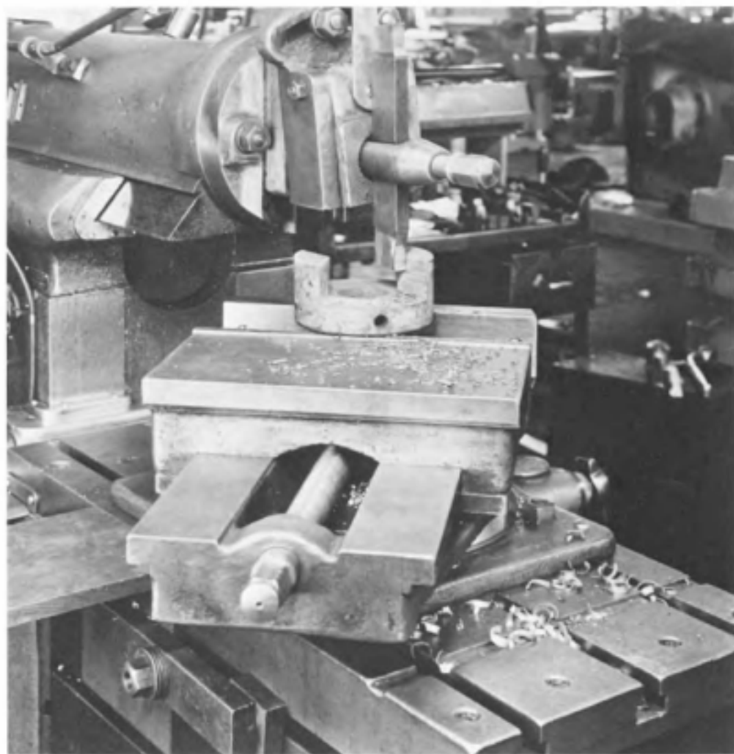
Fig. 2-19. Shaper vise positioned at an angle to shape angular surface.
