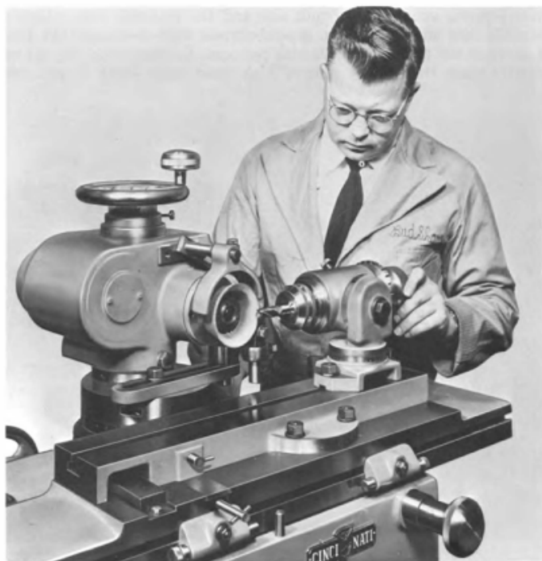
Fig. 14-19. Setup for sharpening the peripheral teeth of an end milling cutter.
