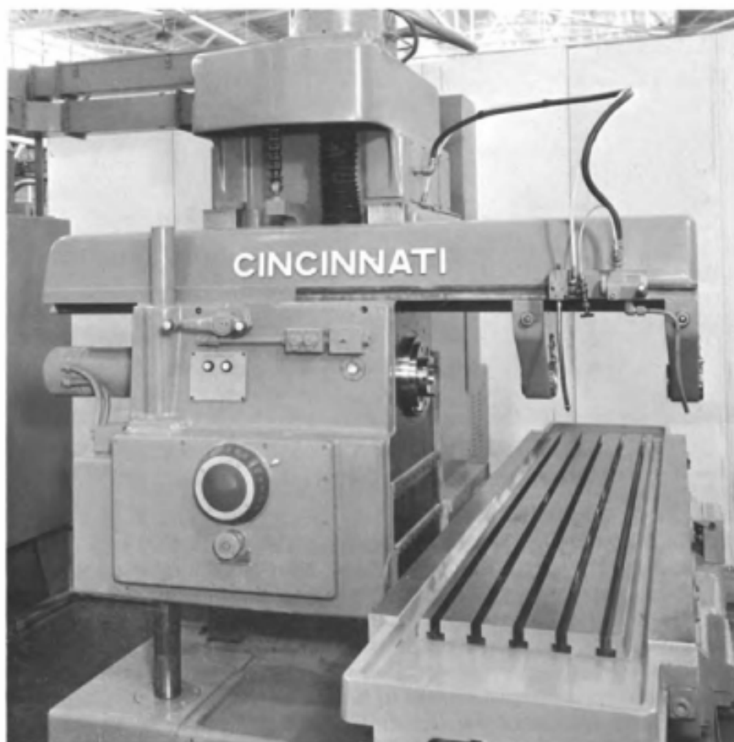
Fig. 4-12. Spindle carrier of fixed-bed milling machine.
