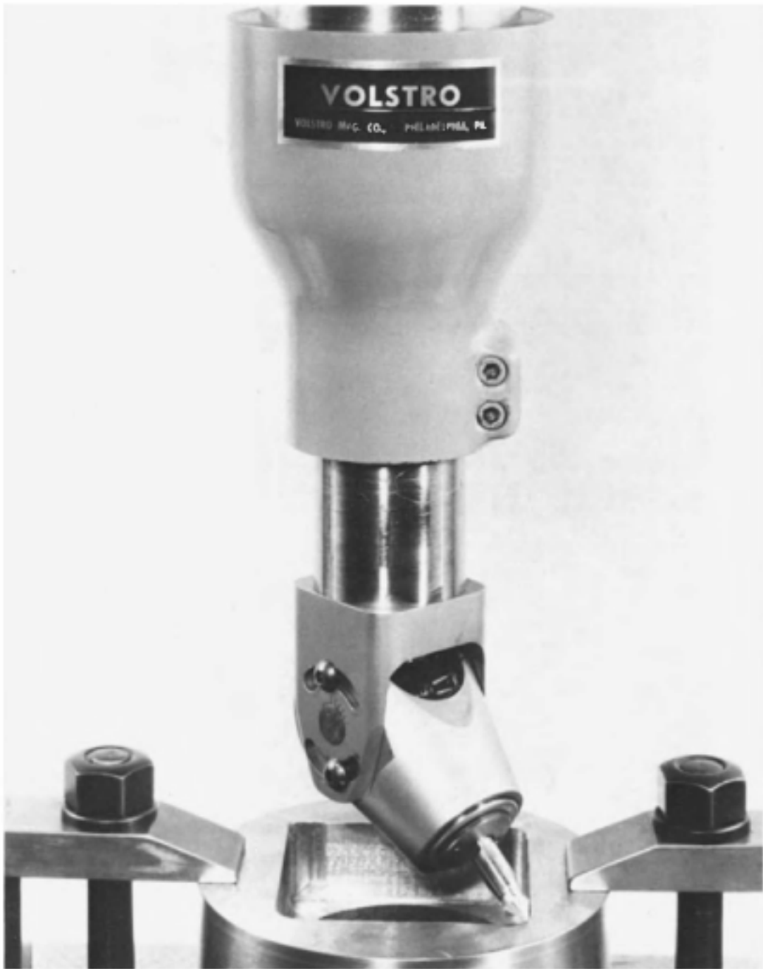
Fig. 4-27. Multi-angle milling head milling a sharp 90-degree internal corner.
