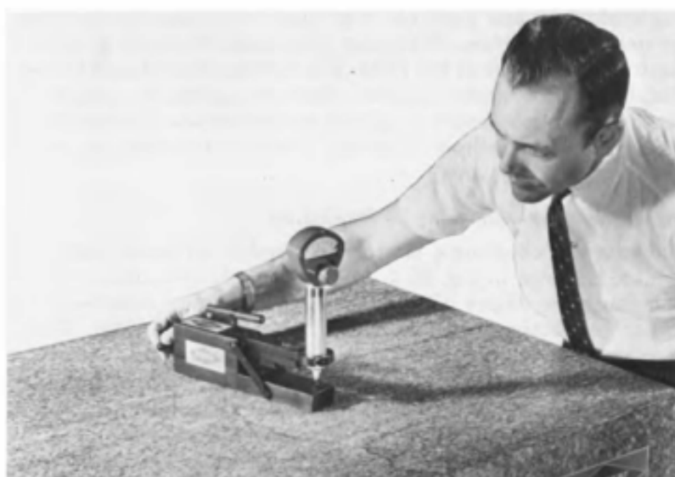
Fig. 16-3. Checking the repeat measurement accuracy of a surface plate with a Repeat-O-Meter.
