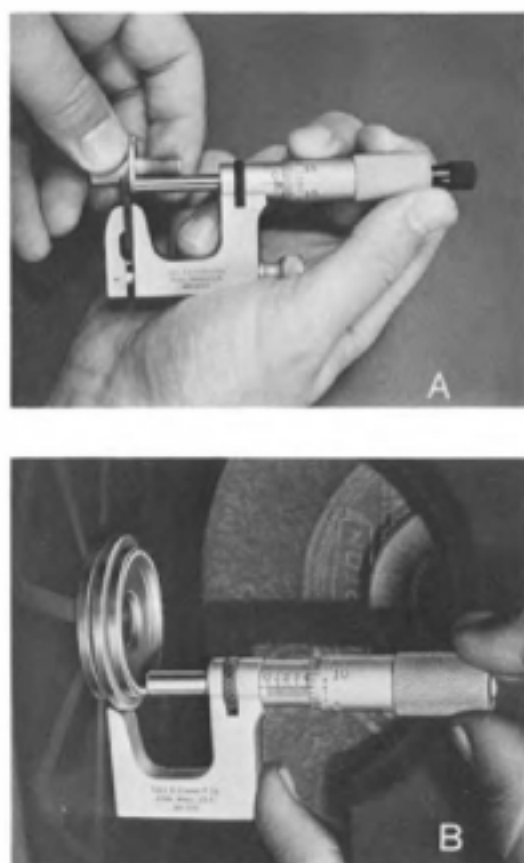
Fig. 2-25. Starrett Multi-T-Anvil micrometer caliper. A. Used as a micrometer caliper. B. Used as a height gage to measure part on surface grinder.
