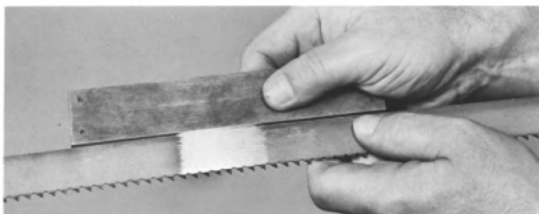
Fig. 16-14. Example of a perfect hand-saw-blade weld.
