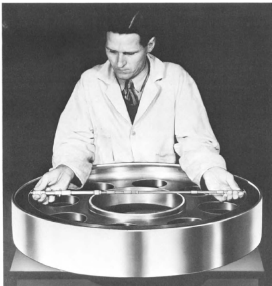
Fig. 2-23. The use of inside-micrometer calipers in measuring a large bore.
