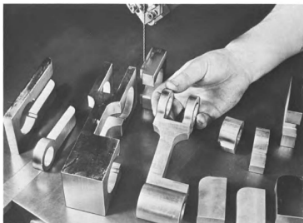
Fig. 16-23. Combining various shaping cuts in several planes enables the vertical-contour band saw to produce very complicated parts.
