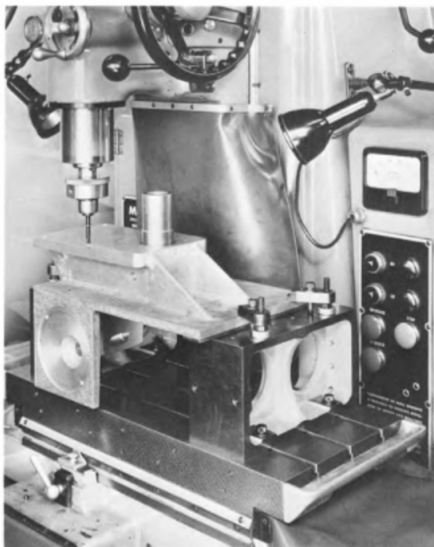
Fig. 15-34. Precision box parallels used to elevate and clamp work above table-top.
