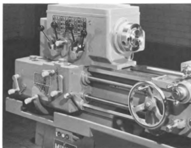
Fig. 6-9. Geared type headstock with quick-change gearbox.
