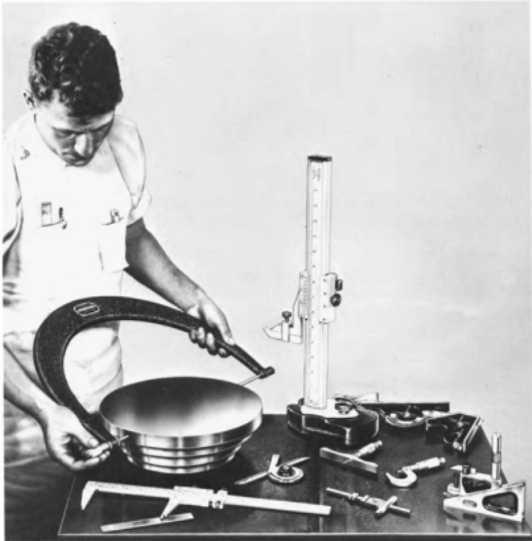
Fig. 2-1. Basic machinists' measuring tools including a precision surface-plate.
