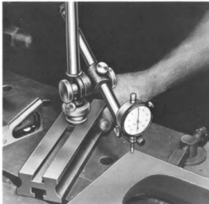
Fig. 2-26. Dial test indicator and planer gage—shown in background—are used to check the size of a machined surface on a planer.
