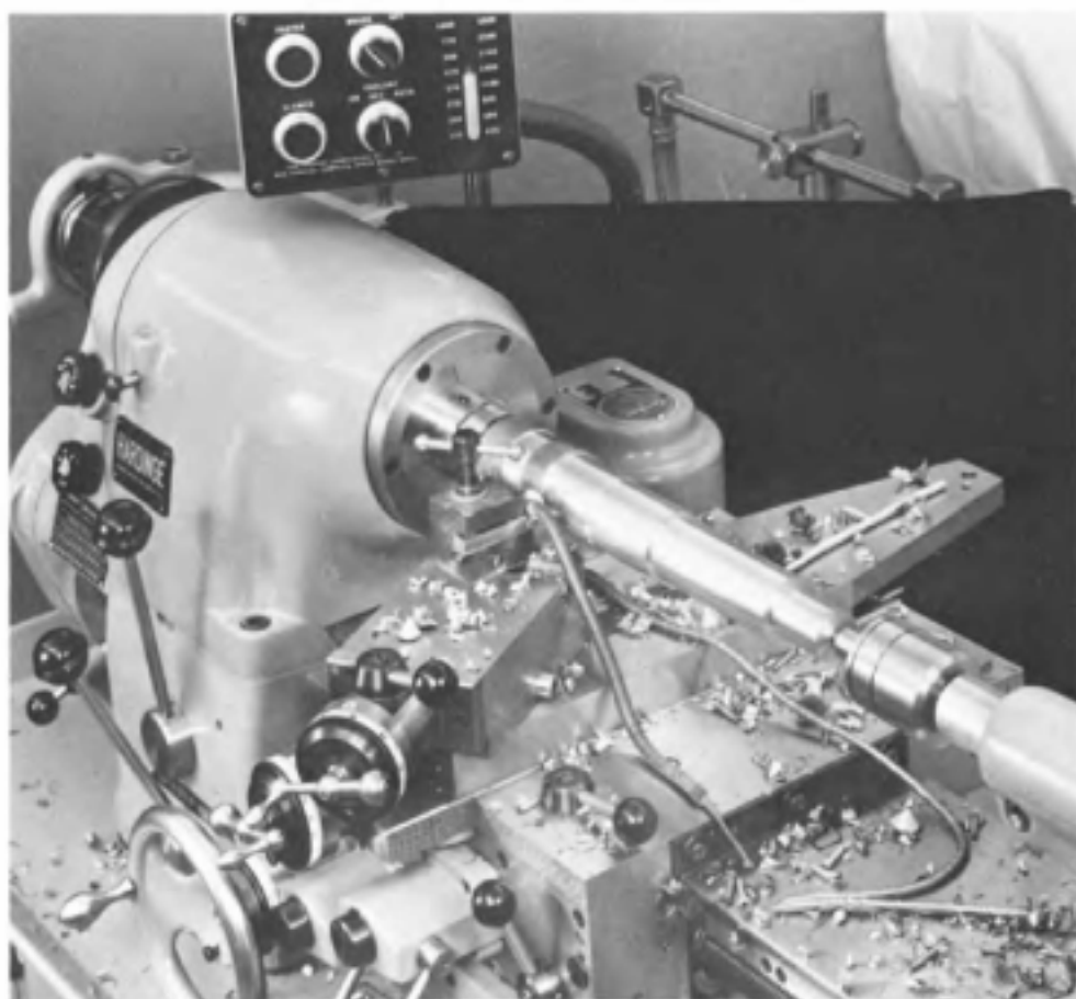
Fig. 8-3. Turning with workpiece mounted on the tailstock center and in a collet chuck.
