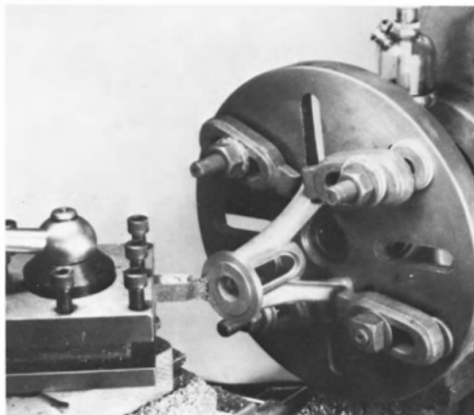
Fig. 11-17. Facing a model steam-engine trunk-column casting.
