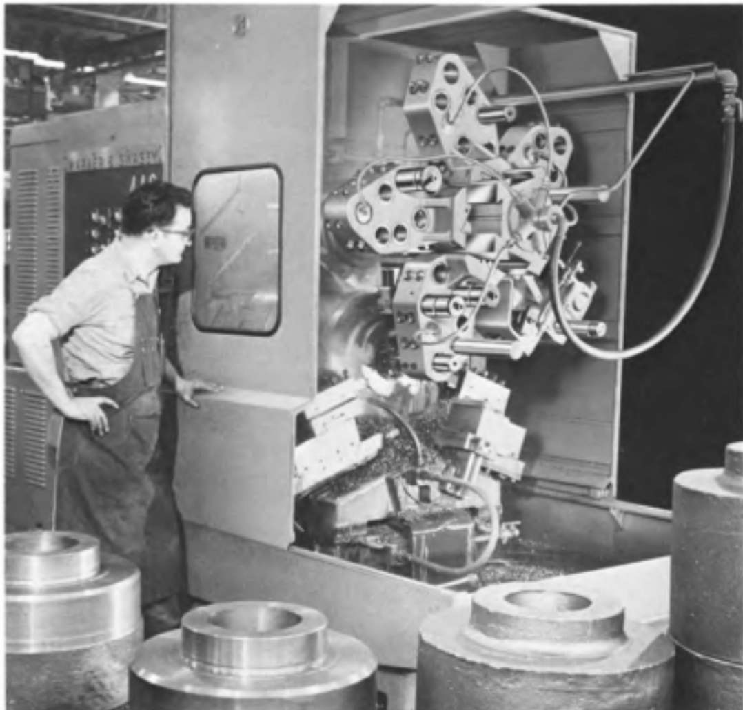
Fig. 14-20. Machining heavy castings in an automatic chucker.
