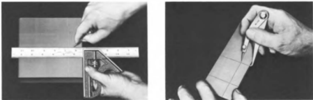
Fig. 3-3. (Left) Using combination square and scribe to lay out plate. (Right) Using hermaphrodite calipers to lay out plate.
