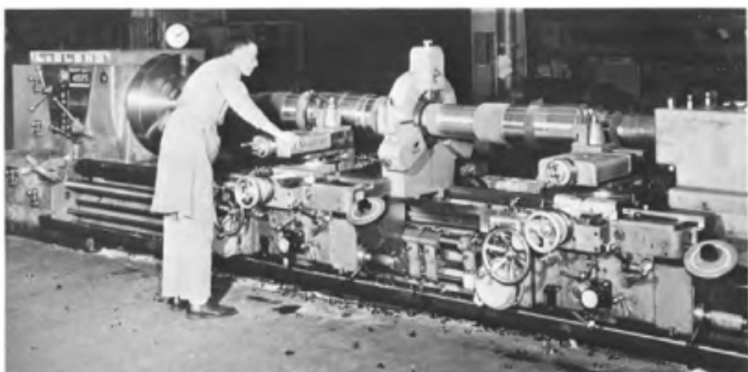
Fig. 8-28. Large steadyrest used to support long workpiece held in a chuck and between centers on a lathe having two carriages.
