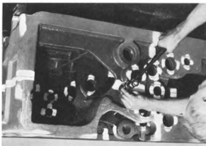
Fig. 3-11. Prick punching the first setup line.
