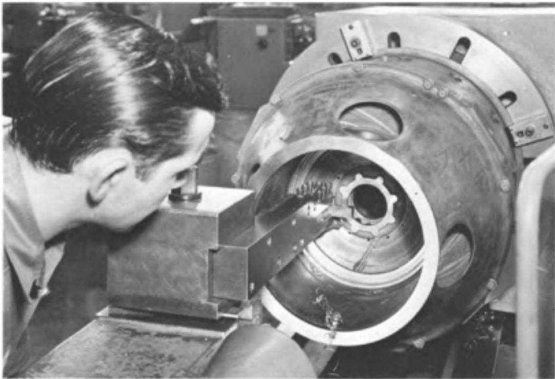
Fig. 11-4. Boring and facing operations performed on an assembly of parts that are clamped directly to a faceplate.
