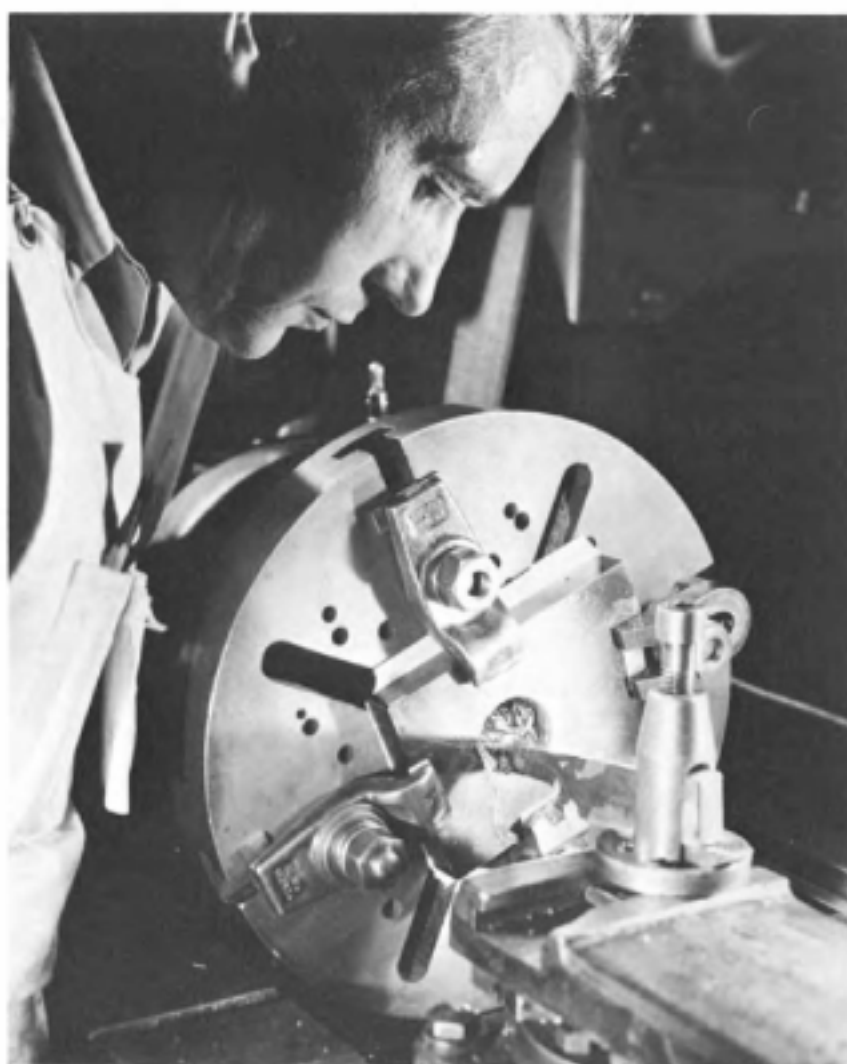
Fig. 15-10. Boring the hole in the lathe with the work mounted on a faceplate.
