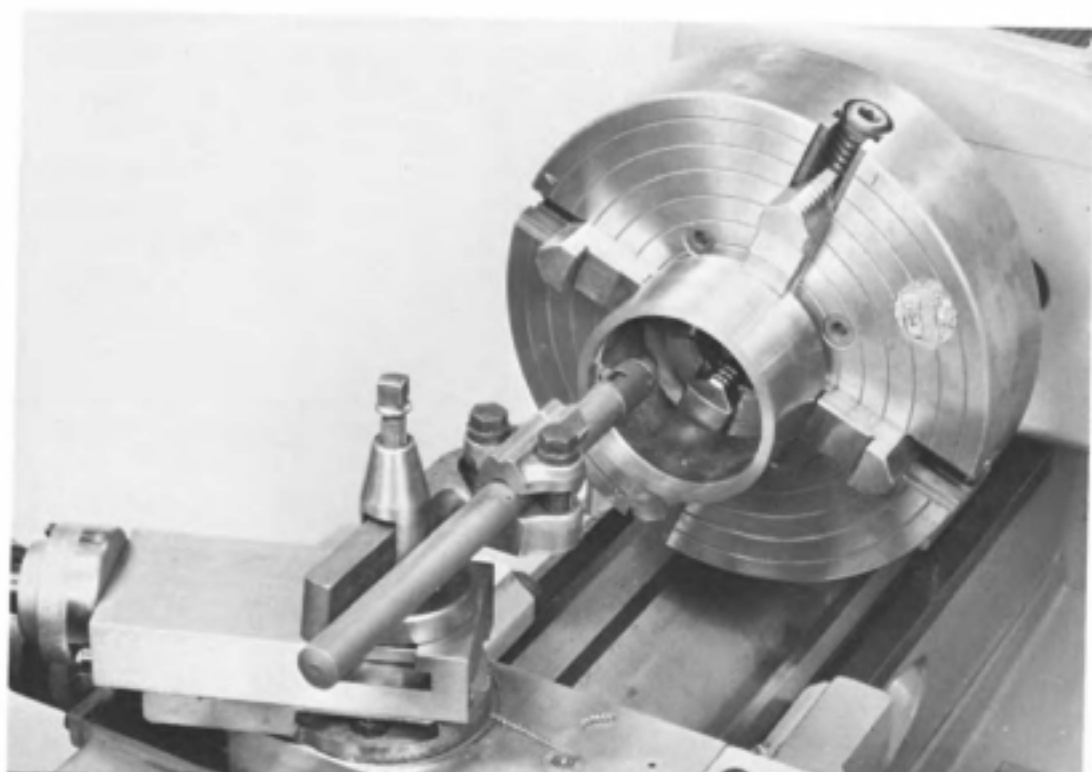
Fig. 9-24. Boring a hole on an engine lathe.
