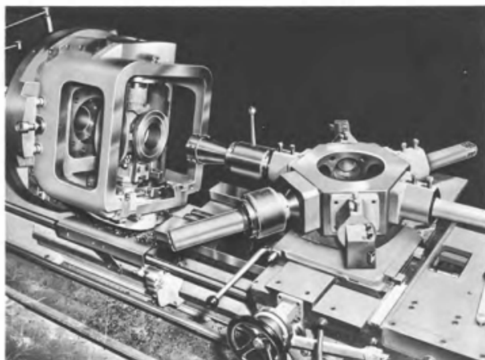
Fig. 14-17. Machining steel gate-valve bodies held in an indexing fixture on a saddle type turret lathe having a cross-sliding turret.
