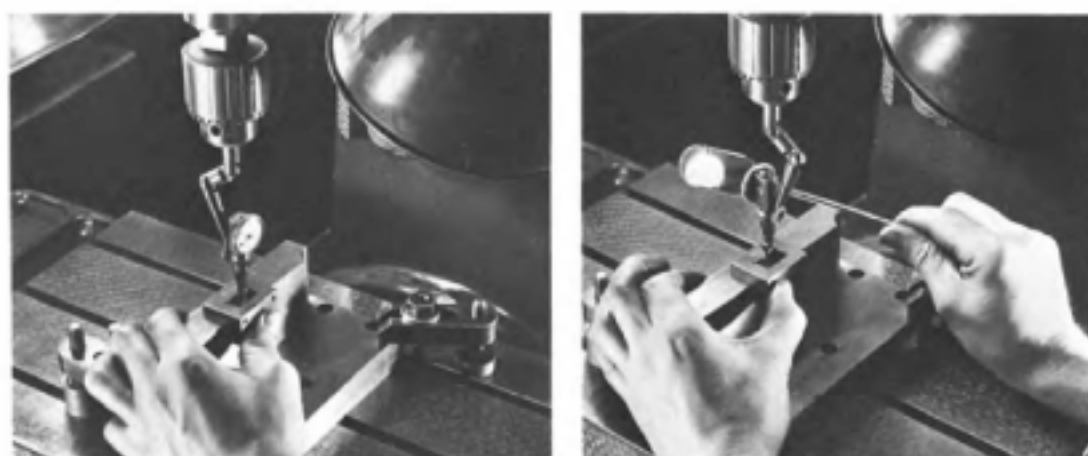
Fig. 15-23. Procedure for picking up the edge of a workpiece using a Moore Edge Finder.
