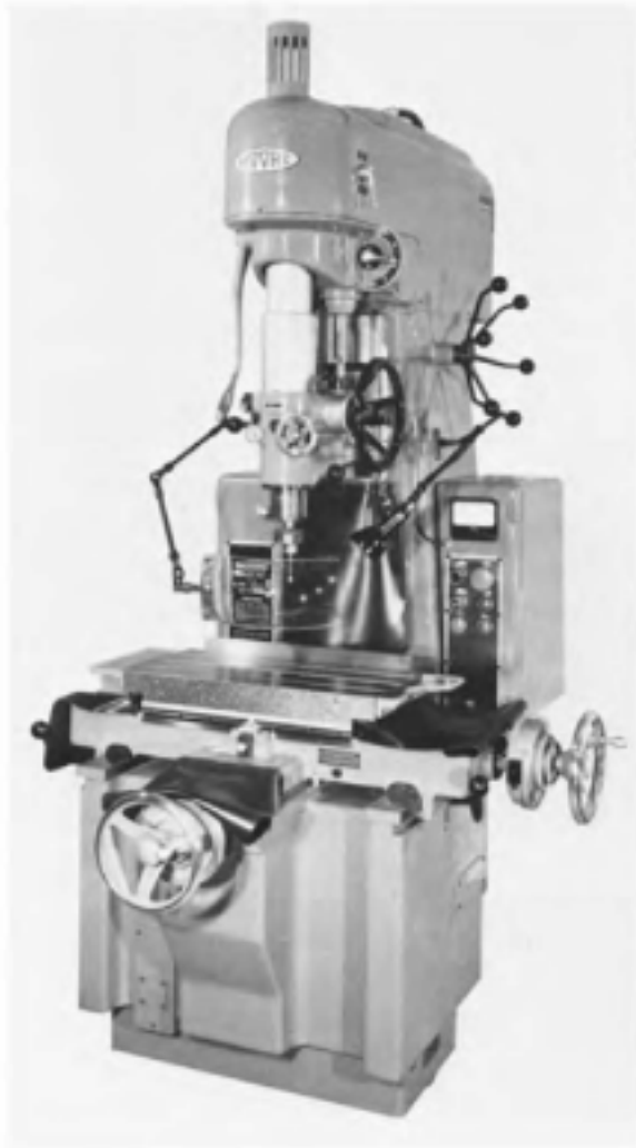
Fig. 15-14. Moore precision jig-borer having ultra-precision lead screws to make precise coordinate table positionings.
