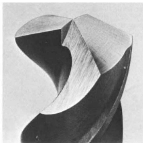
Fig. 4-8. Standard split-point drill grind. Web replaced by two secondary cutting edges.
