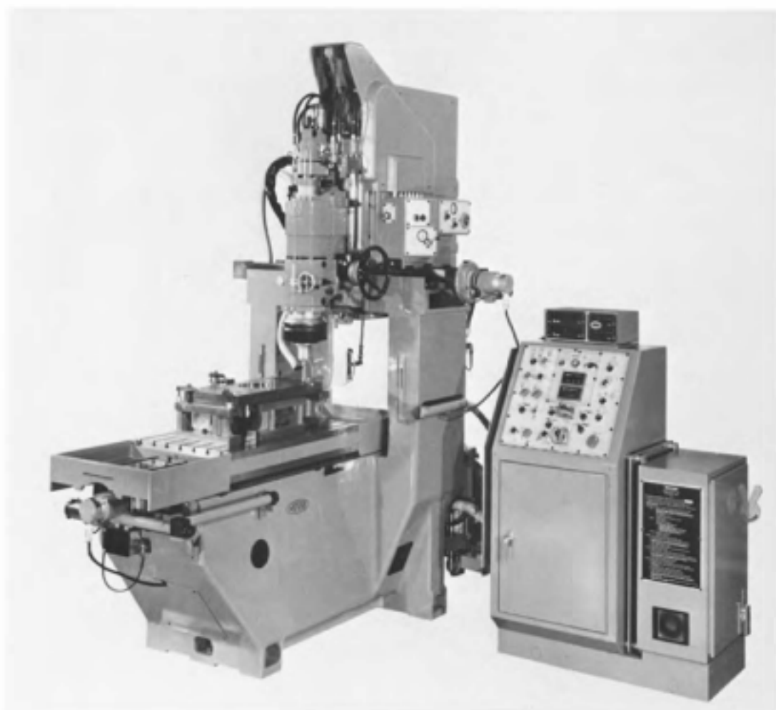
Fig. 15-41. Fixed bridge type jig-grinder equipped with inch-metric preselect and readout systems.
