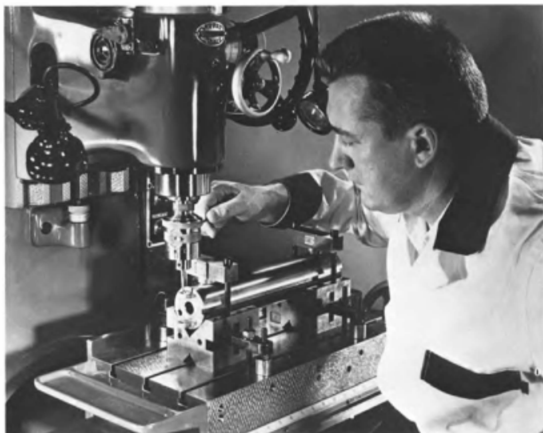
Fig. 15-32. Cylindrical workpiece set up on precision V-blocks for jig-boring.
