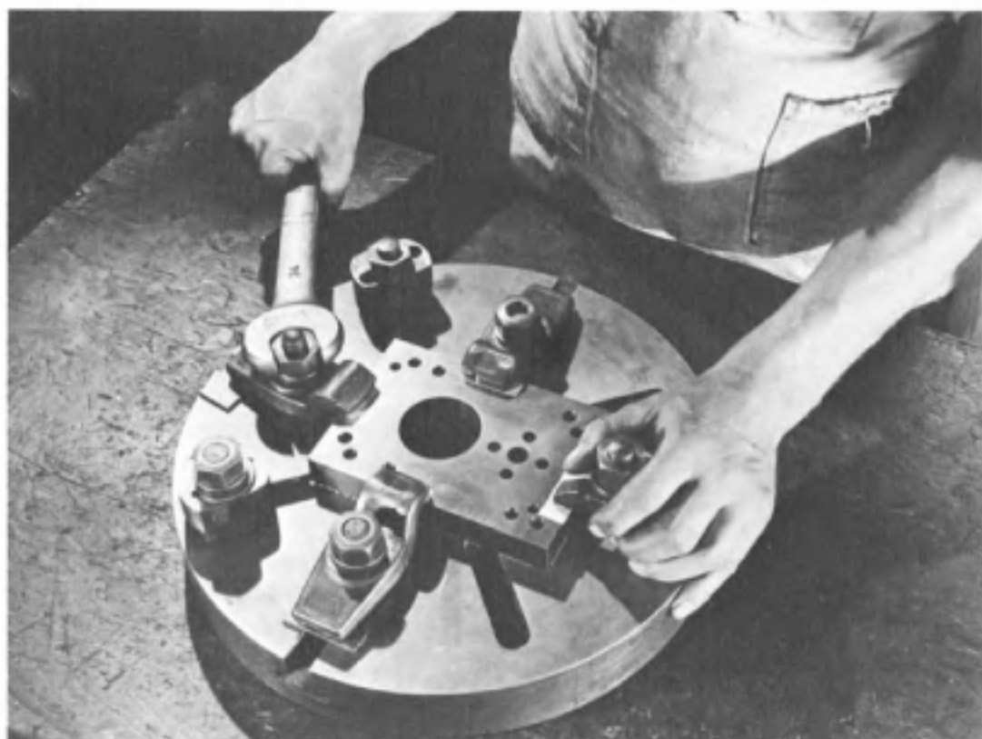
Fig. 15-37. Clamping the workpiece to a lathe faceplate. The faceplate is removed from the lathe spindle to make this job easier.
