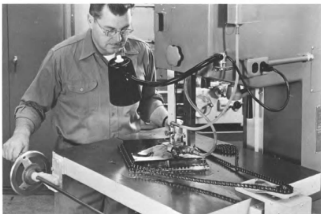
Fig. 16-22. Combining the hydraulic table-feed and servo-contour directional feed-control for cutting straight lines and contours.
