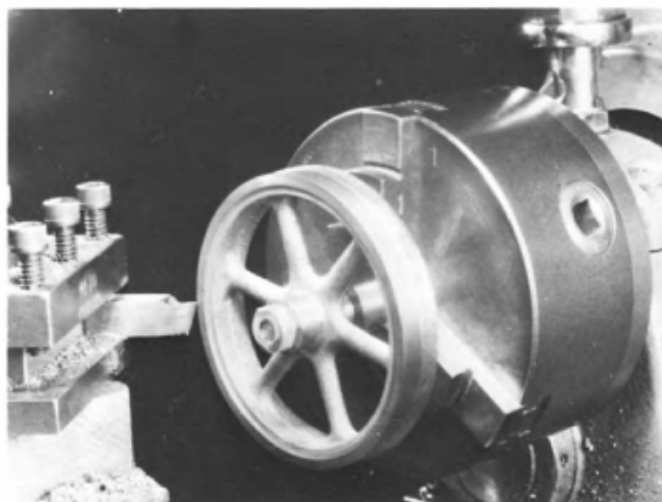
Fig. 9-31. Stub mandrel used to align bore of workpiece with axis of lathe to insure concentricity and perpendicularity of turned surface with bore.
