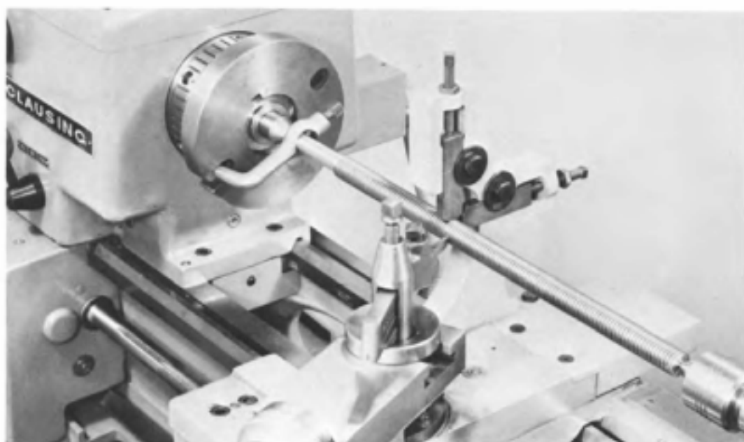
Fig. 13-26. Cutting an Acme thread for a lead screw.
