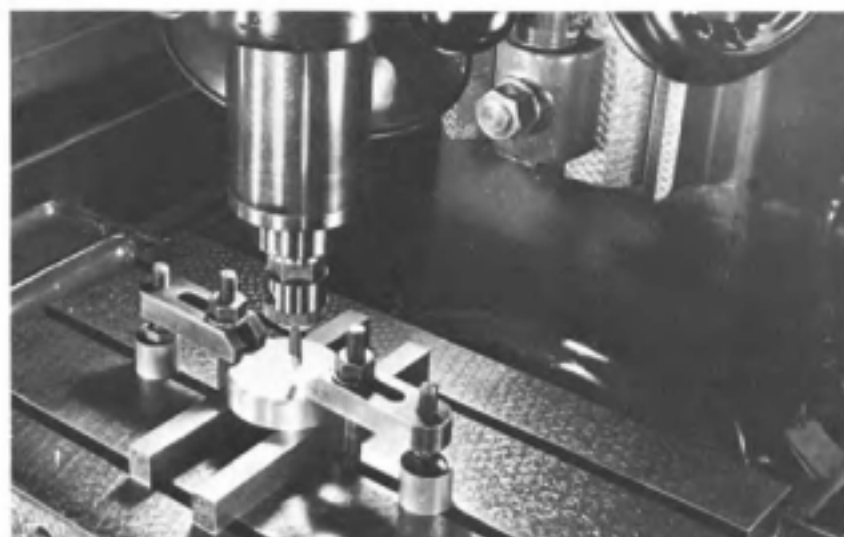
Fig. 15-27. Spot drilling for producing very small holes using a spotting drill. (Right) Special spotting drill.
