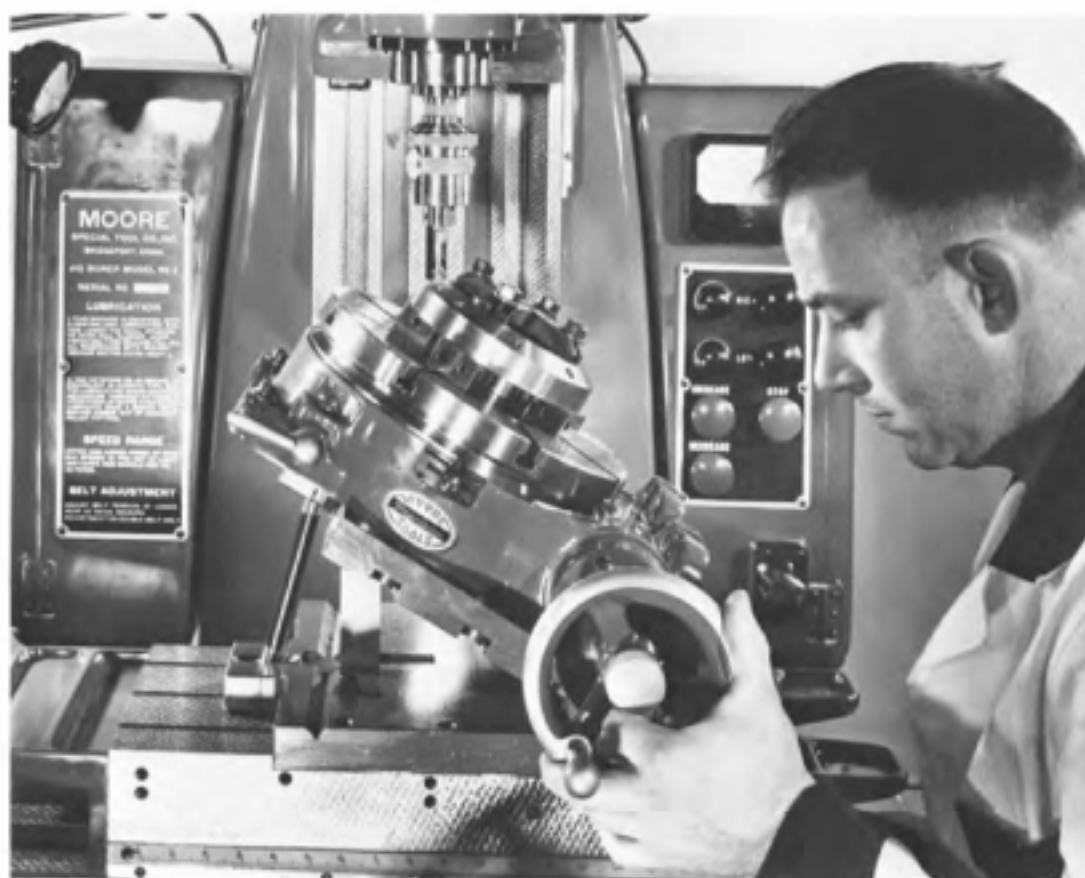
Fig. 15-31. Jig-boring holes at an angle and equally spaced in a circular pattern around a common center. The work is mounted on a rotary table which is clamped to a sine table.
