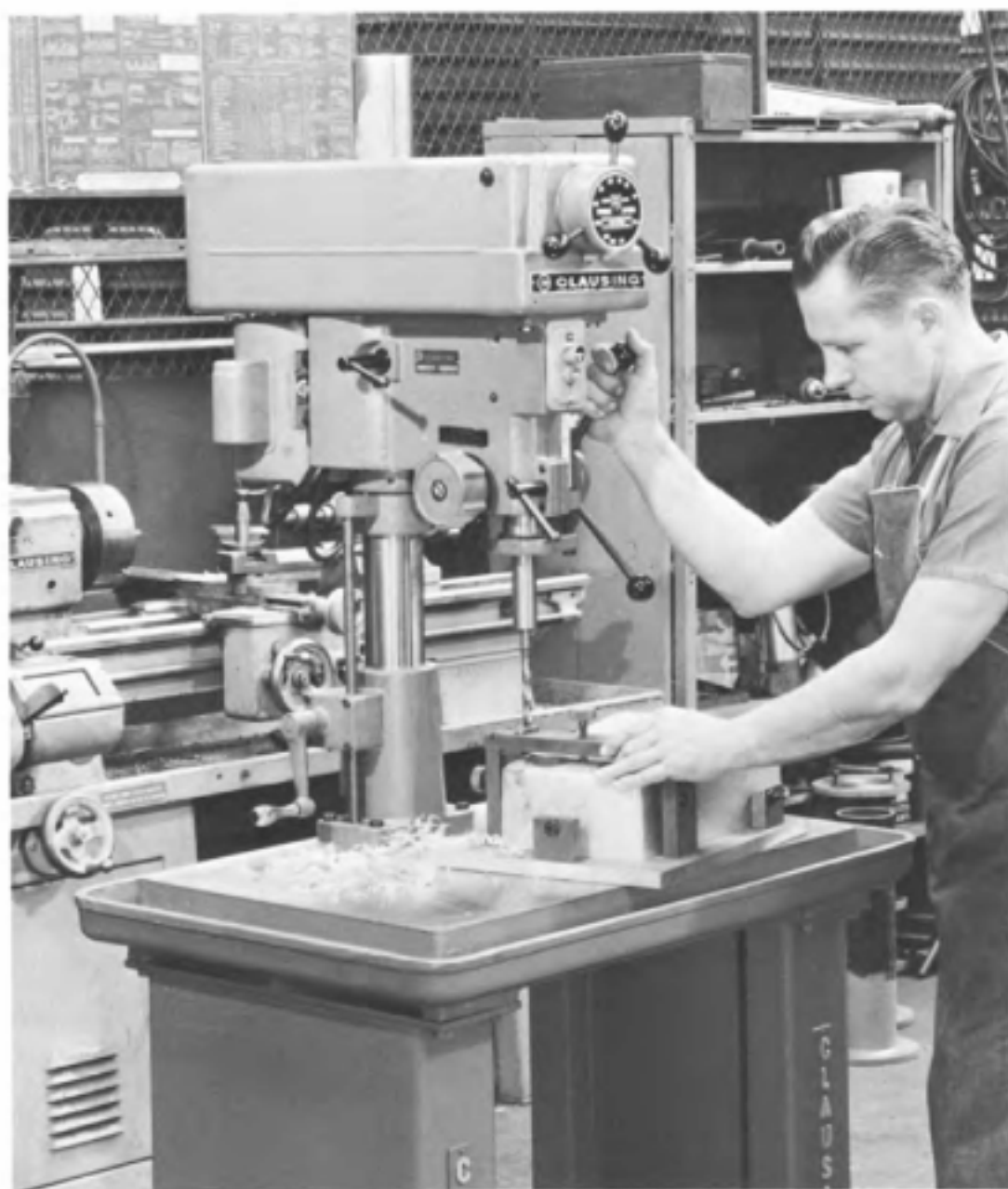
Fig. 5-20. Casting held in a drill jig for drilling operation. Note that the part is held to the table manually.
