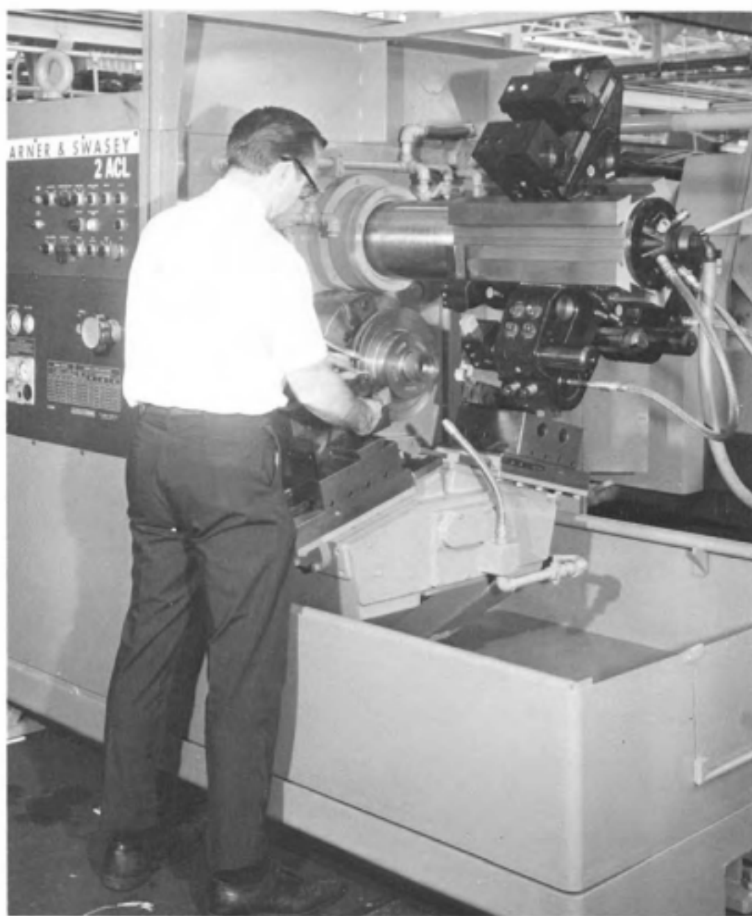
Fig. 14-19. Changing a tool in an automatic chucker.
