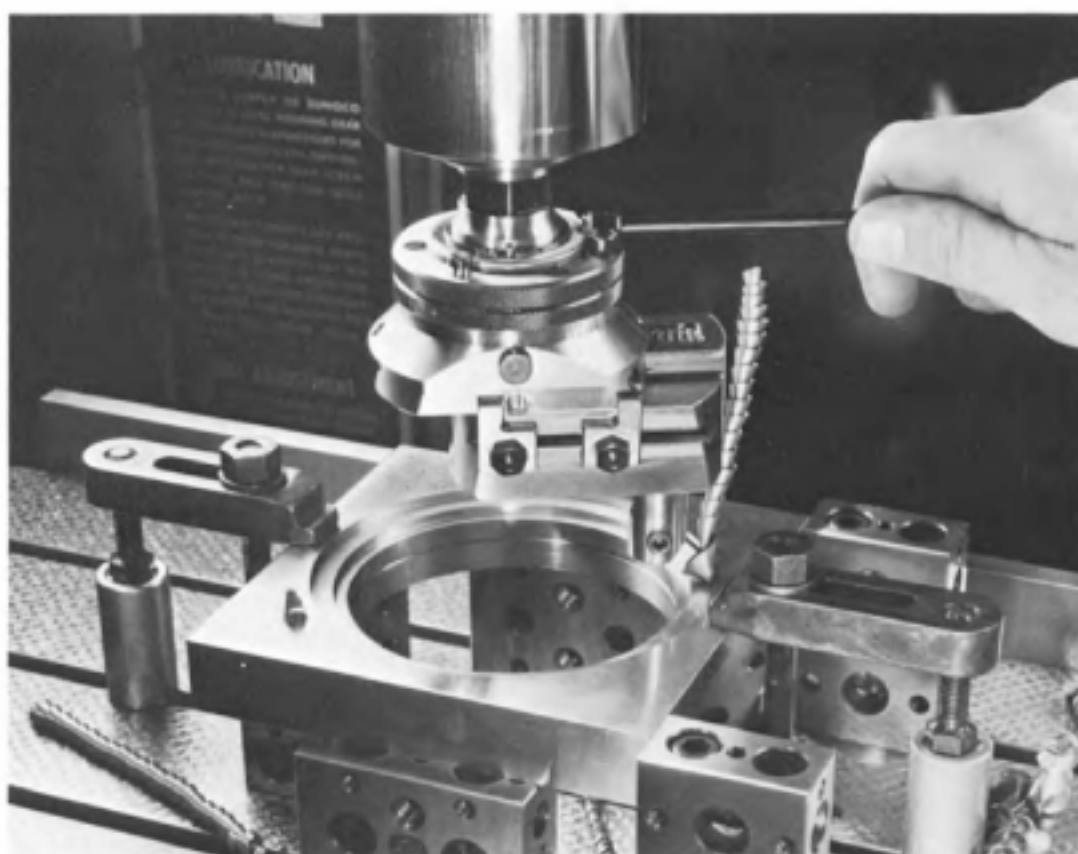
Fig. 15-33. Universal offset boring and facing head shown taking a facing cut.
