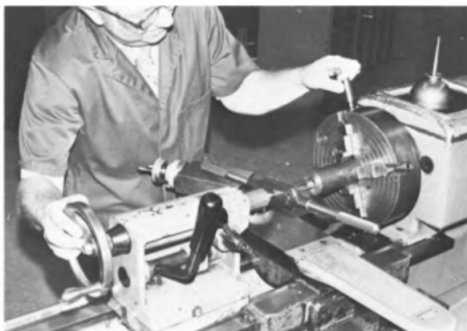
Fig. 13-25. Setup and procedure for tapping a thread on an engine lathe.
