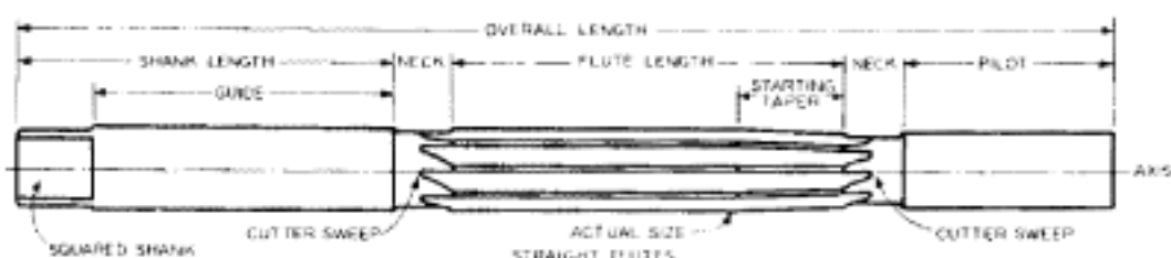
HAND REAMER, PILOT AND GUIDE
