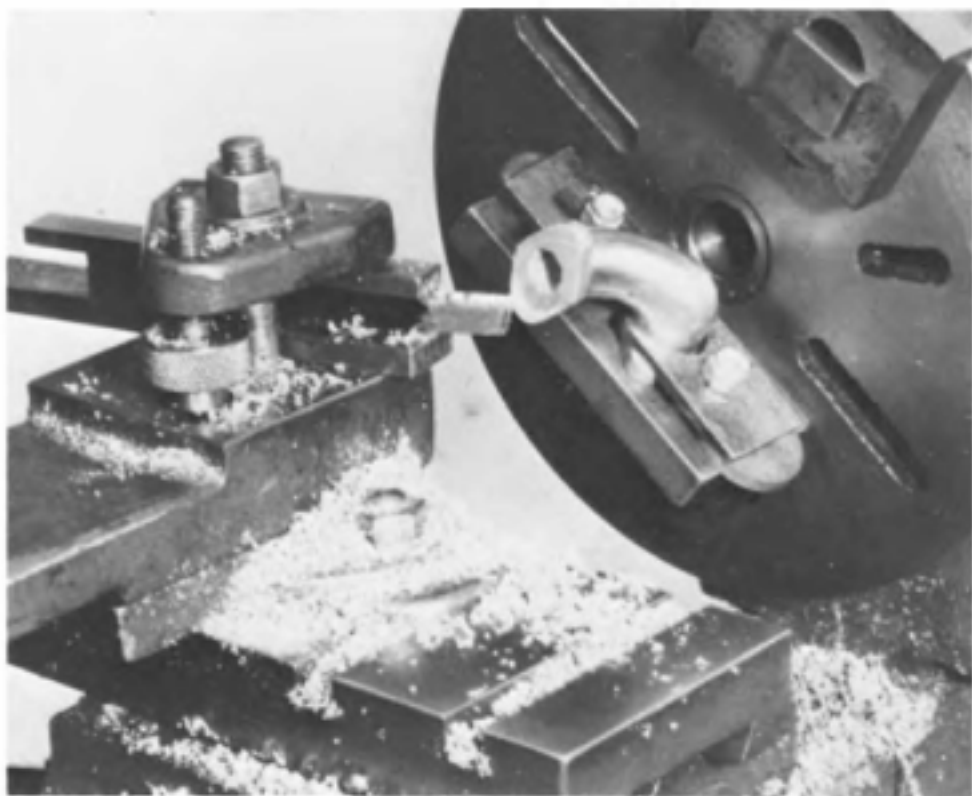
Fig. 11-18. Facing the flange of a curved pipe which is clamped to an angle plate mounted on a faceplate.
