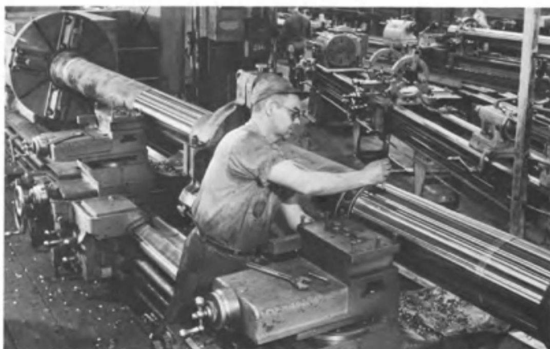
Fig. 8-5. Measuring the diameter of a workpiece in a lathe. The part is held by faceplate jaws at the headstock end.
