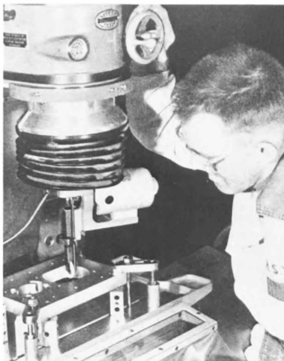
Fig. 15-45. Grinding internal profile of the blanking station of the lamination die using a slot-grinding attachment on a jig-grinder.
