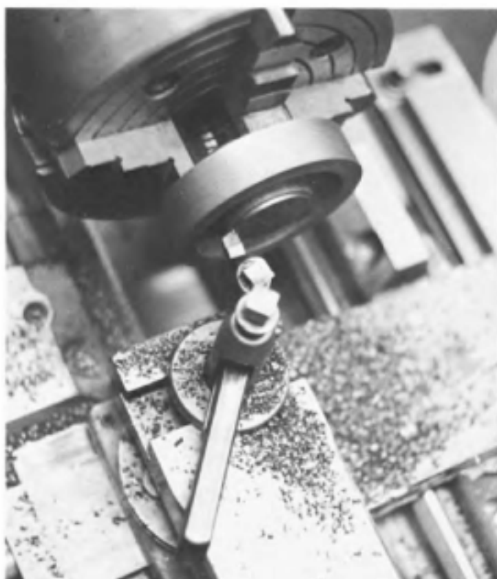
Fig. 9-17. Taking a facing cut on a gear blank.
