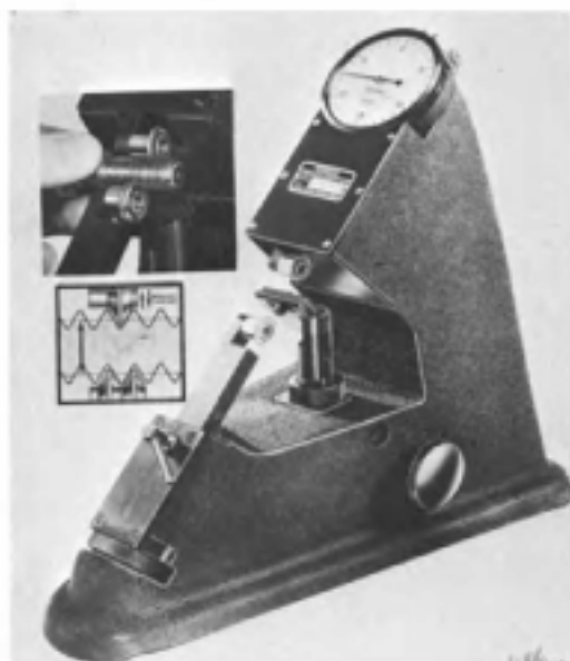
Fig. 12-12. Indicating-type thread comparator for inspecting external thread pitch-diameters. Initial setting established with a setting plug.
