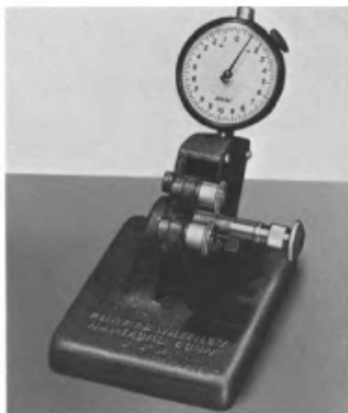
Fig. 12-12. Indicating-type thread comparator for inspecting external thread pitch-diameters. Initial setting established with a setting plug.
