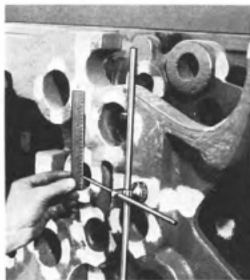
Fig. 3-8. Checking starting reference point of layout with a surface-gage and a ruler.
