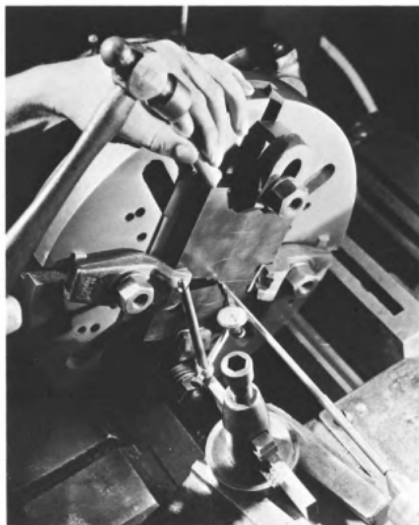
Fig. 15-8. Aligning the work with the axis of rotation of the lathe using a pump center and an indicator.
