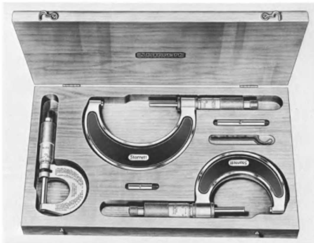
Fig. 2-18. Outside micrometer caliper set including length standards.
