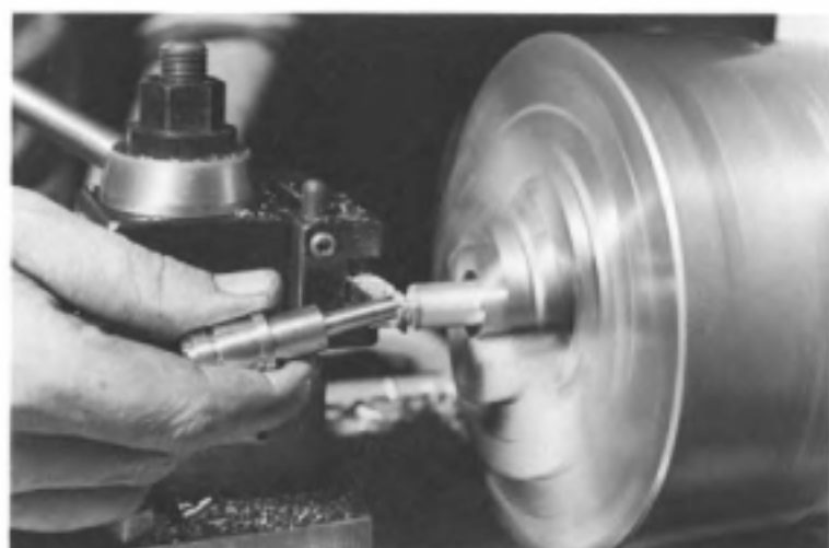
Fig. 9-27. Cutting off a finished part in an engine lathe.
