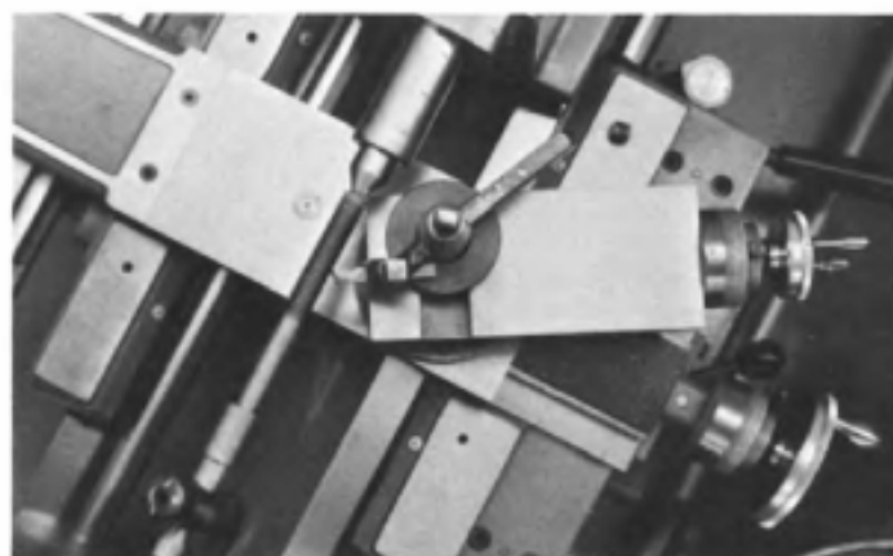
Fig. 13-16. Cutting an American Standard Unified thread with the workpiece held between two centers.
