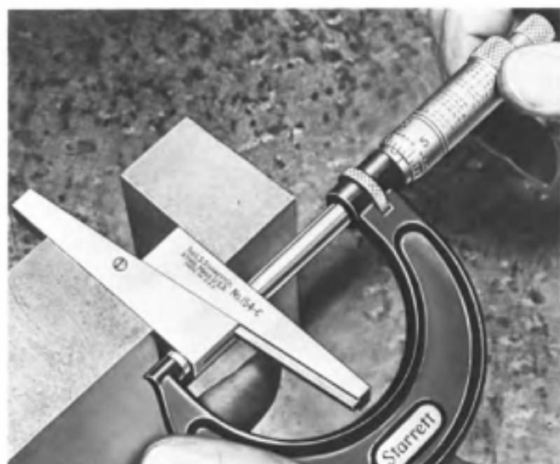
Fig. 2-31. Measuring the width of a slot using adjustable parallels and micrometer calipers.
