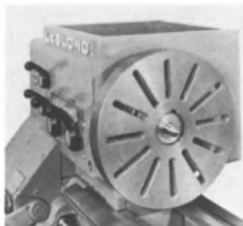
Fig. 6-22. Large faceplate for holding workpieces that cannot conveniently be held by other methods.
