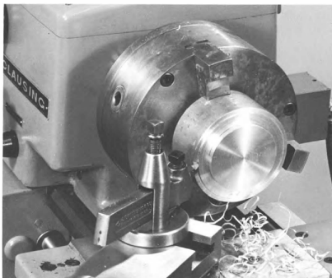
Fig. 9-16. Turning a part that is held in a 3-jaw universal chuck.
