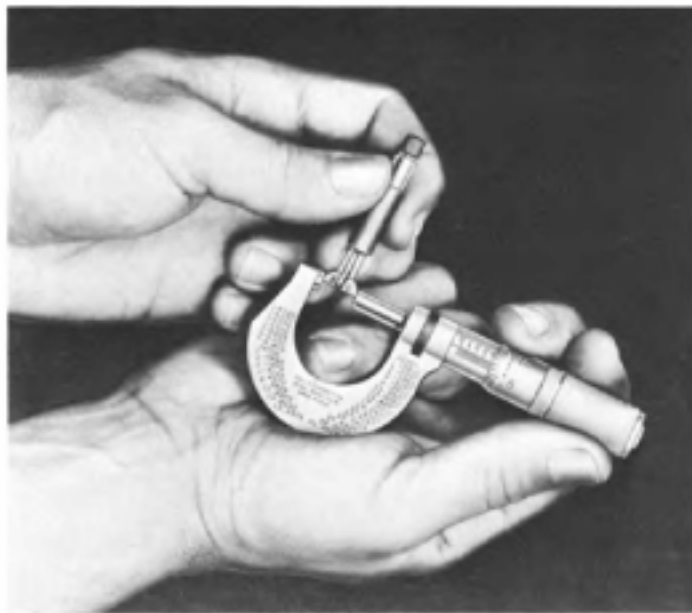
Fig. 2-7. Small hole gage-setting measured by outside-micrometer caliper.
