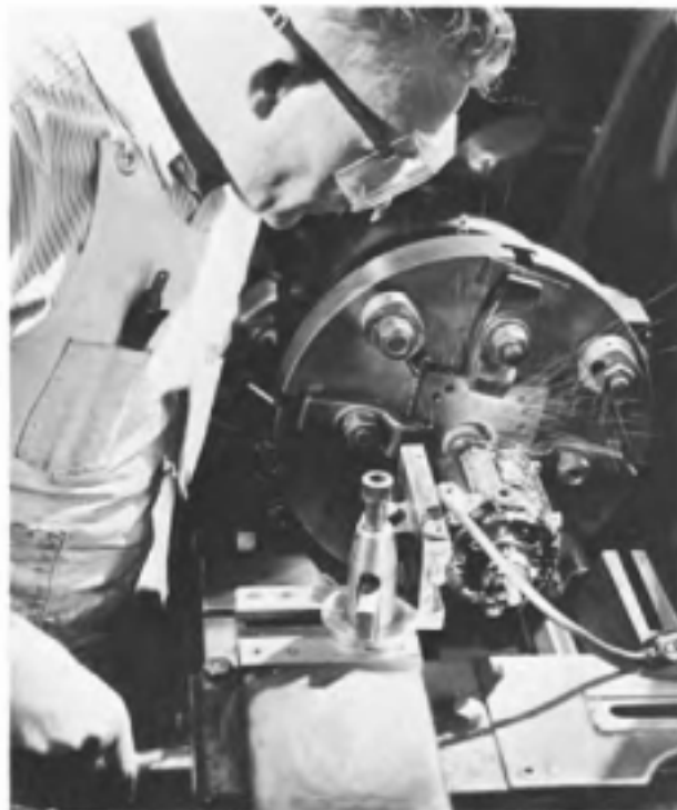
Fig. 15-39. Locating a hole in a hardened die by mounting it on a faceplate and grinding it in a lathe using a toolpost grinding attachment.
