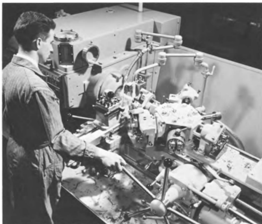
Fig. 14-16. Ram type turret lathe setup for bar work.
