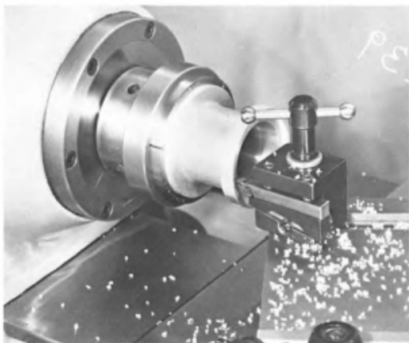
Fig. 9-13. Step chuck holding workpiece to perform turning, facing, boring, and counterboring operations.
