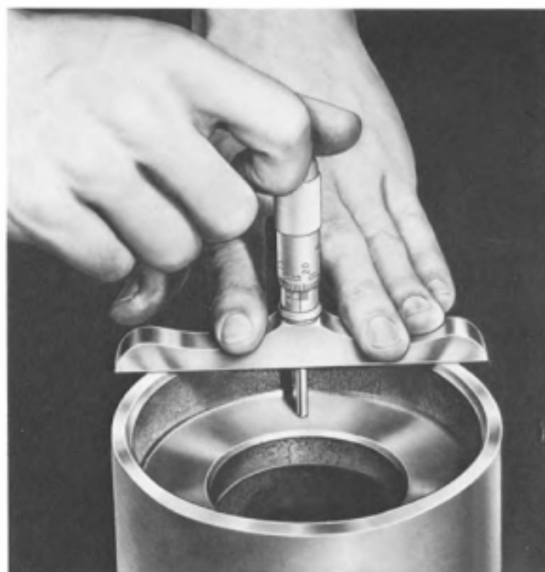
Fig. 2-24. Using depth micrometers to measure shoulder depth.
