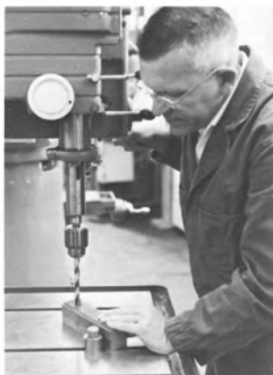
Fig. 5-4. Using a bolt clamped to the table to resist the drill torque while holding the workpiece against the table by hand.
