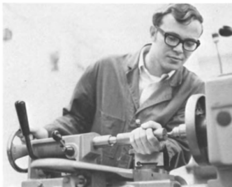
Fig. 8-7. Drilling center holes in the ends of a cylindrical workpiece.
