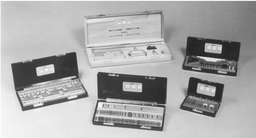
Figure 1.1. Rectangular and square gage blocks and their accessories. A micrometer gage block check set is at the lower right corner. (Courtesy of DoAll.)
