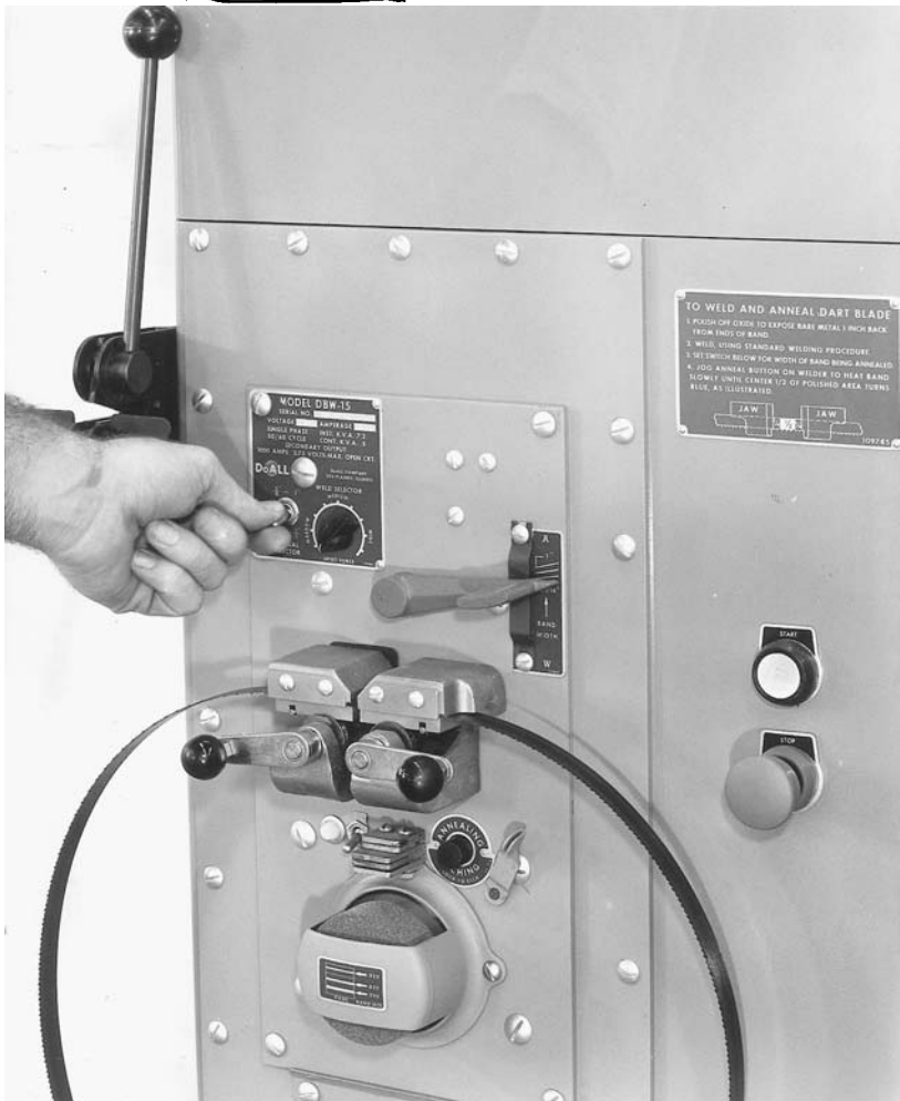
Figure 2.5. Contour saw. Most contour band saws have a welder that permits making internal cuts by drilling a hole in a segment of the portion of stock to be removed, inserting the ends of the blade through the hole, and welding them into a band.
