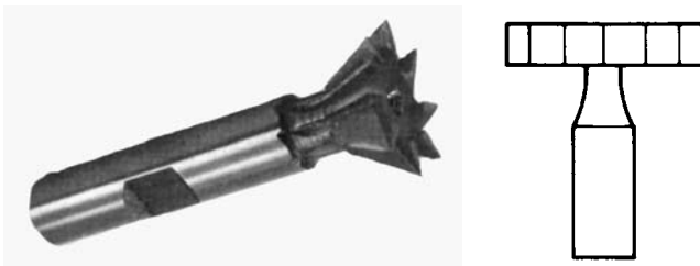
Figure 4.5. A dovetail cutter (a), used for cutting angles, and a Woodruff key cutter (b), used for keys inserted in shafts.
