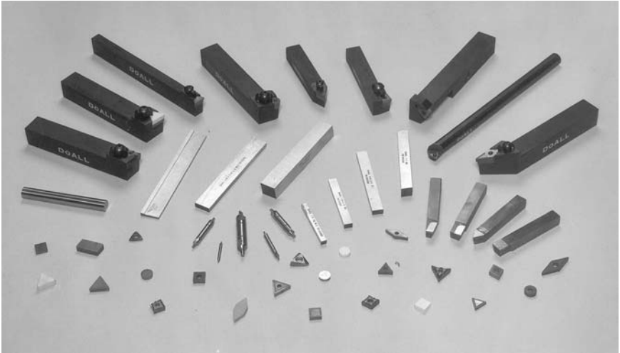
Figure 3.19. Array of carbide tool inserts and toolholders, high-speed toolbits, center drills, and brazed carbide toolbits. Top row: carbide toolholders; second row: cut-off tools and cast toolbit; third row: center drills and high-speed toolbits; right side: cemented brazed carbide toolbits; bottom row: carbide inserts, ceramic insert. (Courtesy of DoAll.)
