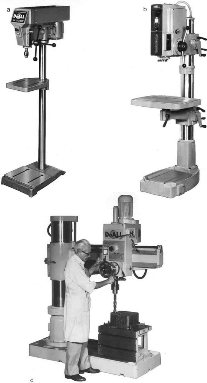
Figure 5.1. Sensitive, gear-head, and radial drill presses. These are the three drill presses most commonly used in the shop: (a) the sensitive, (b) the gear-head, and (c) the radial. (Courtesy of DoAll.)
