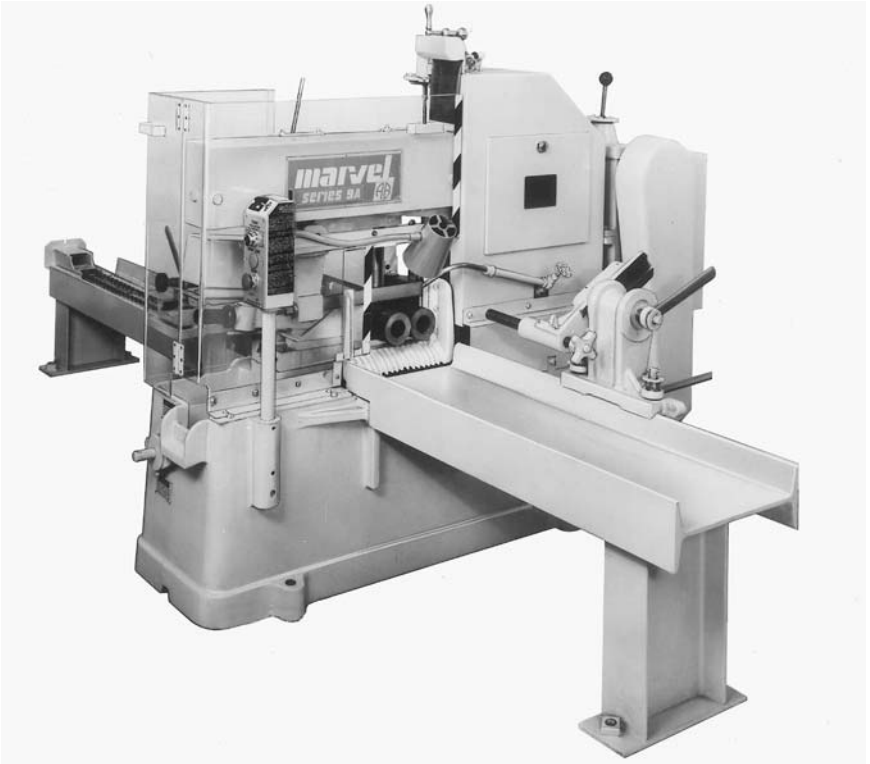
Figure 2.8. Power hacksaw. Simple and rugged, the power hacksaw has been a standby for cut-off for more than a century. Economical and accurate, it is well suited to low-volume cut-off but is too slow for volume cutting work. (Courtesy of Armstrong-Blum Manufacturing Co.)
