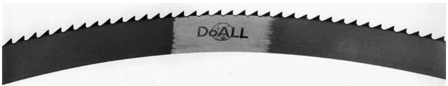
Figure 2.13. Weld area of properly welded band saw blade. (Courtesy of DoAll.)
