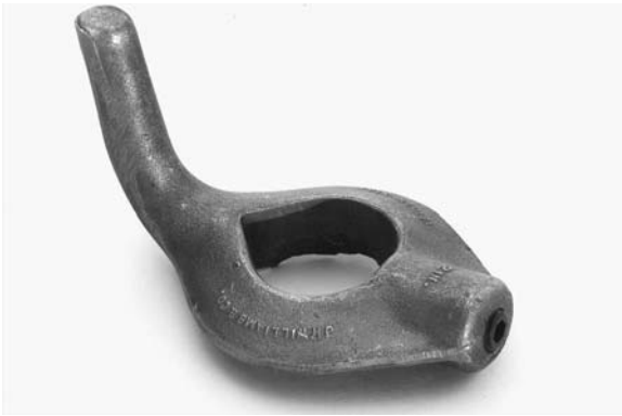
Figure 3.12. Bent lathe dog, used when turning on centers.
