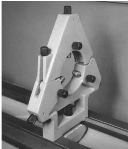
Figure 3.8. Steady rest, which is used to support heavy bars. (Courtesy of DoAll.)
