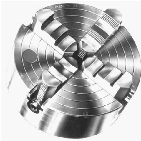
Figure 3.6. A typical four-jaw (independent) chuck. (Courtesy of DoAll.)
