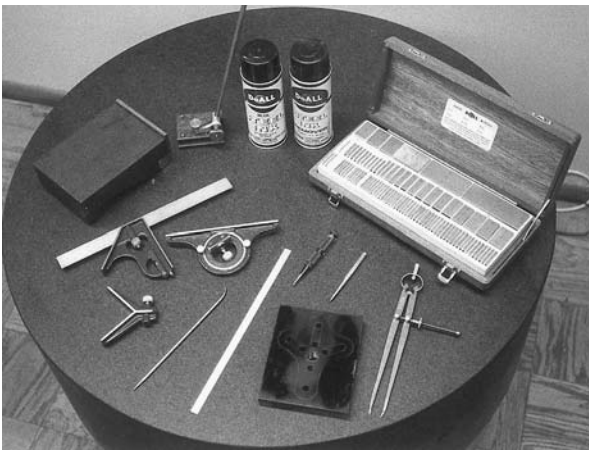
Figure 1.3. Array of gages, including gage blocks, combination square, surface gage, and other tools. (Courtesy of DoAll.)
