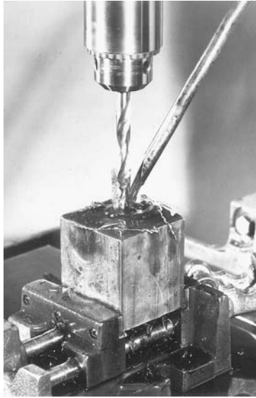
Figure 5.9. Drilling on a drill press, using cutting fluid, with part held in vise and clamped to drill press table. (Courtesy of DoAll.)
