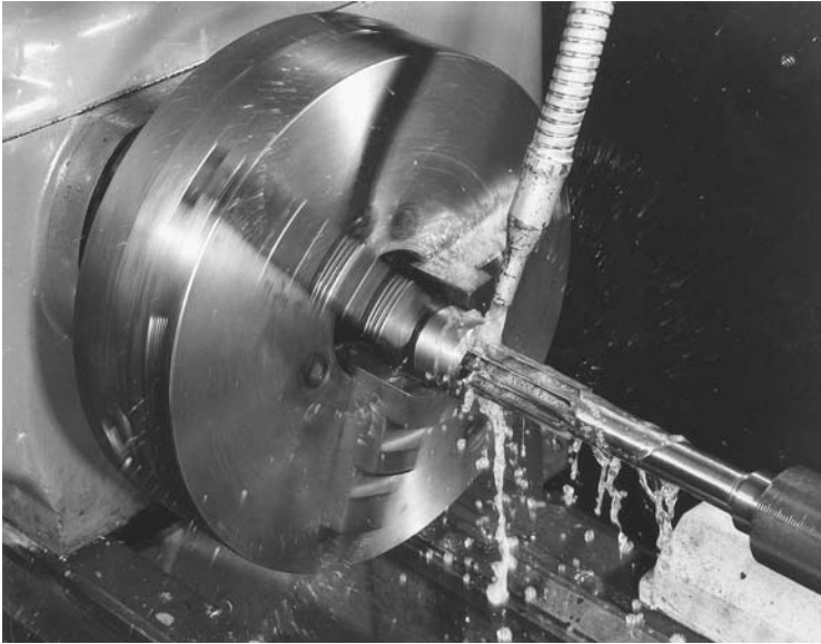
Figure 3.18. Reaming a hole on the lathe, using ample cutting fluid. (Courtesy of DoAll.)
