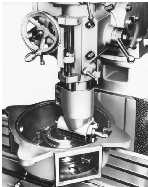
Figure 4.10. A right-angle milling attachment for a vertical mill. It fits directly in the spindle and is driven by the milling machine head motor. (Courtesy of DoAll.)
