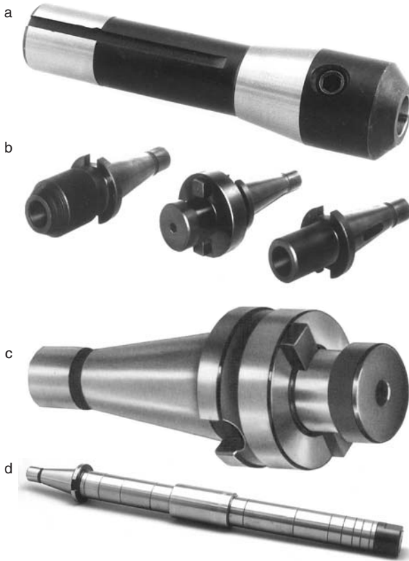
Figure 4.7. Several types of milling machine holders. (a) R-8 end mill holder. (b) ISO (National Taper) end mill holder. (c) Shell mill holder. (d) Milling machine arbor.
