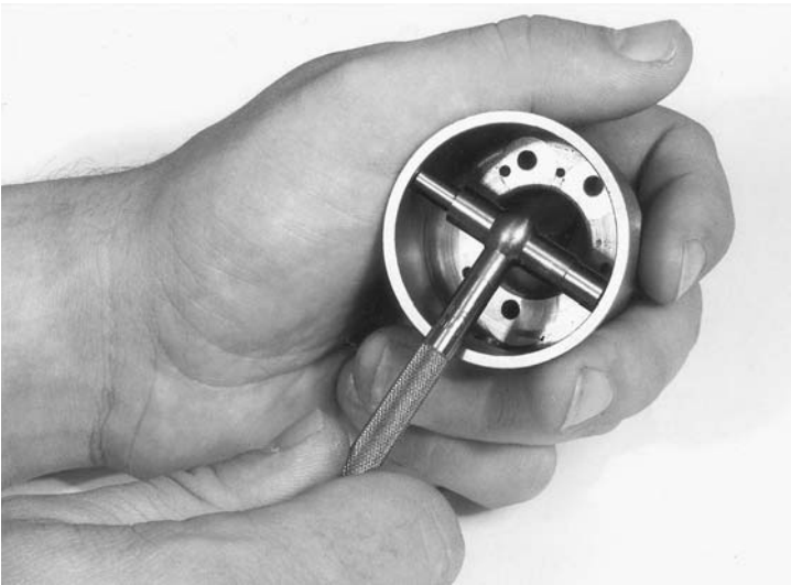
Figure 1.4. Telescopic gage measuring an internal surface. (Courtesy of DoAll.)
