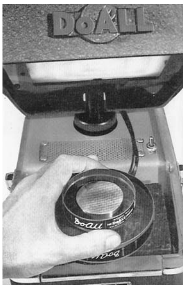
Figure 1.2. That absolute and immutable standard—the wave length of light—becomes a practical measuring tool for industry through the use of optical flats and monochromatic light generators.
