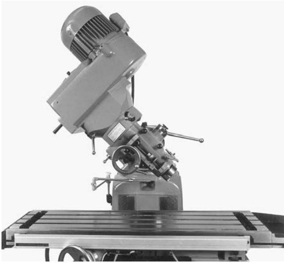
Figure 4.2. Milling machine head showing the angles it can be tilted, exhibiting its independence of movement. (Courtesy of DoAll.)
