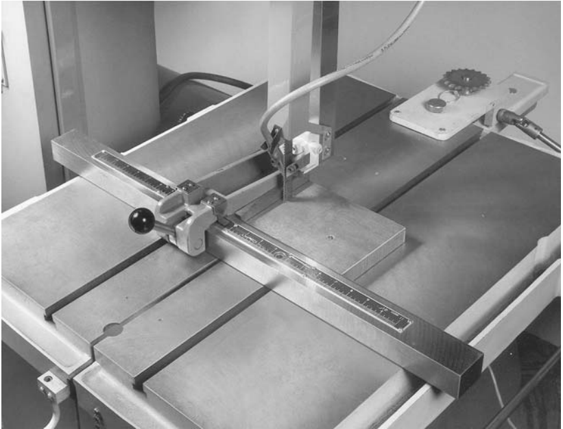
Figure 2.11. The squaring bar (shown on the left) is used to accurately position work relative to the blade for precision sawing.
