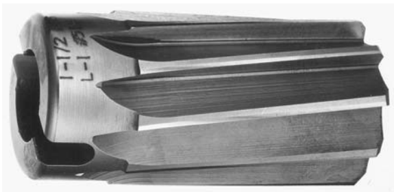
Figure 5.4. Reamer, showing chamfered cutting edges. The reamers cut on the chamfer; the angled cutting edges cut at the front of the tool.
