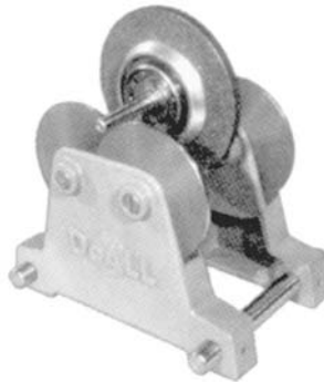
Figure 6.4. Wheel balancer. To ensure accurate, vibration-free operation, the grinding wheel must be properly balanced and trued.
