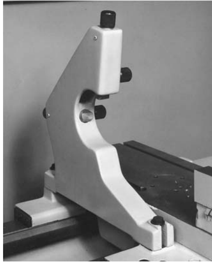
Figure 3.9. Follower rest, which is used to support long thin shafts. Otherwise, the shaft would bend due to the pressure exerted by the tool. (Courtesy of DoAll.)
