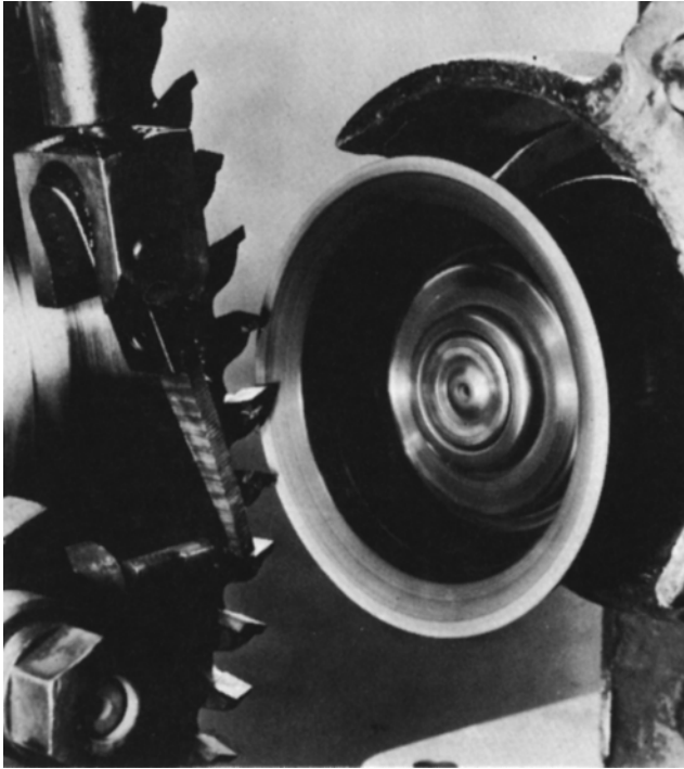
Figure 4-3 Grinding a carbide cutter with a diamond grinding wheel.
