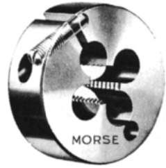
Figure 12-5 Screw-adjusting type of round adjustable die. A fine-pitch screw forces the sides of the die apart or allows them to spring back together.
