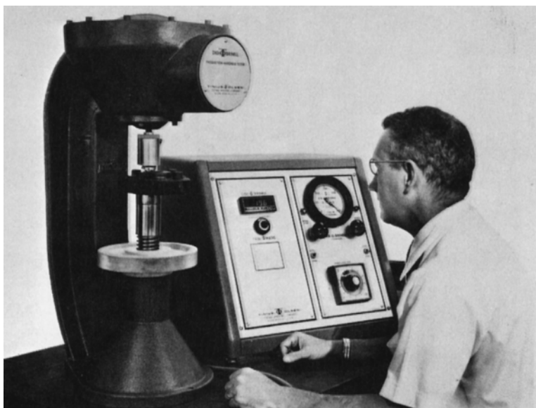
Figure 3-4 Air-o-Brinell metal hardness tester with Digito-Brinell system for digital readout of Brinell values. (Courtesy Tinius Olsen Testing Machine Company)
