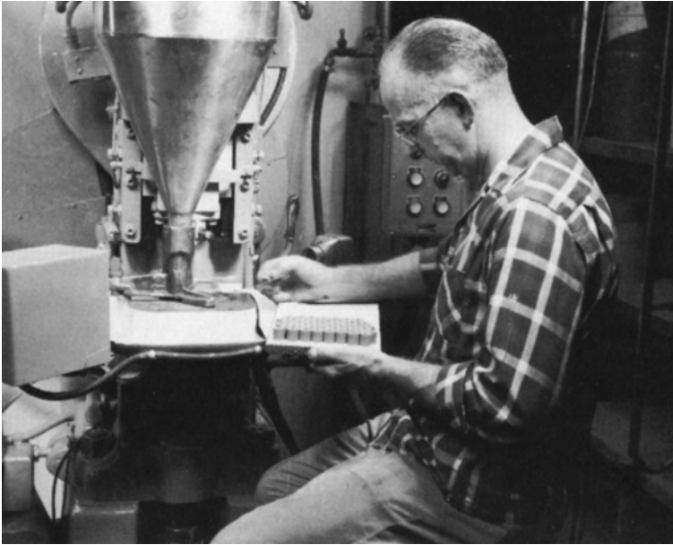
Figure 5-9 Small grinding wheels are molded in automatic presses. The operator merely removes the pressed wheel between strokes. An electric-eye safety device stops the machine if his hand is under the plunger on the pressing stroke. (Courtesy Norton Company.)
