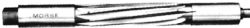
Figure 10-8 Expansion hand reamer with helical flutes. Especially suited for use in holes where the cut is interrupted by a longitudinal slot or keyway. (Courtesy Morse Twist Drill & Tool Company.)
