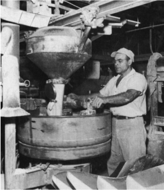
Figure 5-8 Abrasive grain and bond are mixed in power mixing machines to ensure a homogeneous blending. (Courtesy Norton Company.)
