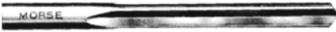
Figure 9-10 Straight-fluted drill for free machining brass, bronze, or other soft materials, particularly on screw machines. Also suitable for drilling thin sheet material because of lack of tendency to “hog.”
