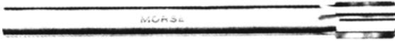
Figure 10-14 Expansion chucking reamer for light finishing cuts in all types of materials. It should not be used to cut oversize holes.
