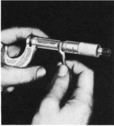
(A) Back off thimble, and tighten the adjusting nut to eliminate play in spindle nut.
