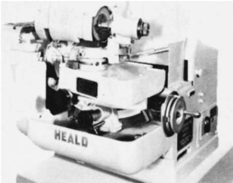
Figure 8-1 Tool-sharpening machine. Direct-reading scales and dials permit grinding different angles, plus the tip radius, in one operation. An extra wheel and freehand grinding attachment are available on the left-hand side of the machine for sharpening odd-shaped tools, or for roughing shapes that will be precision finished on the right-hand side of the machine. (Courtesy Heald Machine Company)
