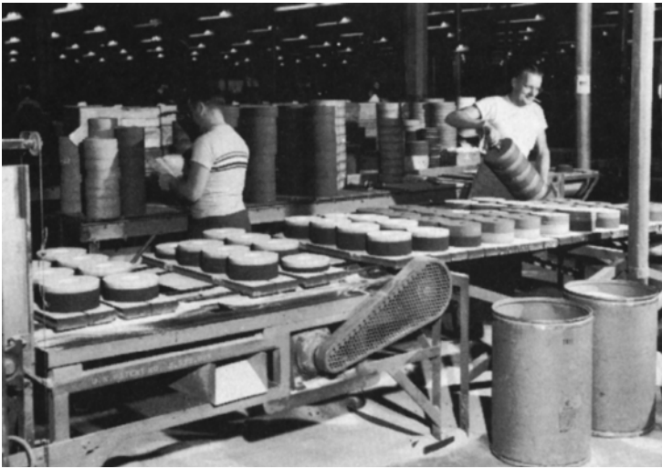
Figure 5-10 Grinding wheels emerging from an electrically heated tunnel kiln where the approximately 2500°F temperature has fused the clay bond into a strong glass. (Courtesy Norton Company)
