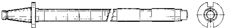
Figure 14-3 Typical milling-machine arbor, Style B. These arbors are longer and require support near the cutters for rigidity.
