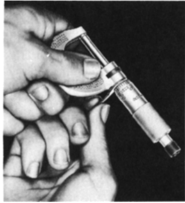
(B) With anvil and spindle in contact, adjust sleeve, so that line on sleeve coincides with zero line on thimble.
