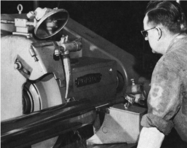
Figure 5-12 Shellac-bonded wheels are widely used for cutlery grinding and high-finish grinding. (Courtesy Norton Company.)
