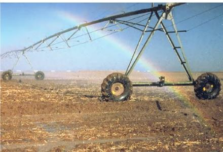
Sprinkler, overhead rain drops. Irrigation machines (e.g. centre pivots and lateral move) were developed in order to save labour and water. Because of improved nozzle alignment, nozzle spacing and timing of water application, the uniformity improved considerably ( $s \approx 0.25$ ). Target field application ratios of 70–75% are common for overhead ‘rain drops’.
