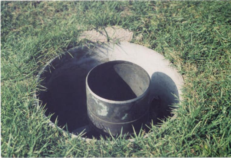
**Fig. 3.1** The equipment used to measure precipitation influences the quantity measured where, the catch diameter, elevation, and surrounding ground cover all influence accuracy
