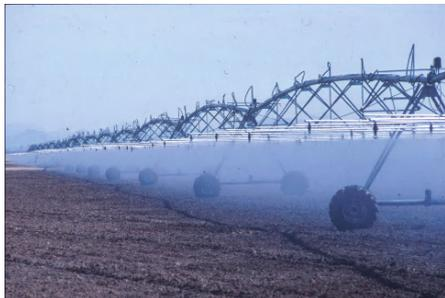
Sprinkler, downward fine spray. Multiple downward spraying nozzles reduce evaporation from ‘rain drops’ and increase uniformity ( $s < 0.1$ ). These irrigation machines thus should (and can) operate at field application ratios (efficiencies) between 0.90% and 0.95%.
